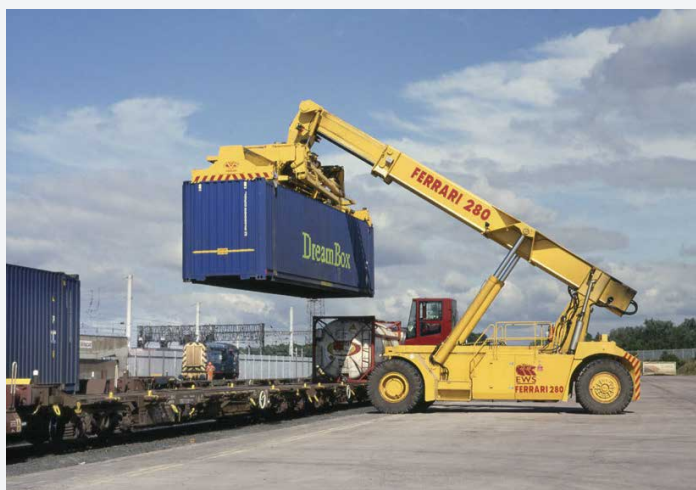
Mossend Euroterminal has never been equipped with fixed lifting equipment. One of the terminal's two Ferrari reach stackers positions a 40ft container at the terminal on August 27th, 2003, while pilot locomotive 08807 shunts empty wagons.
