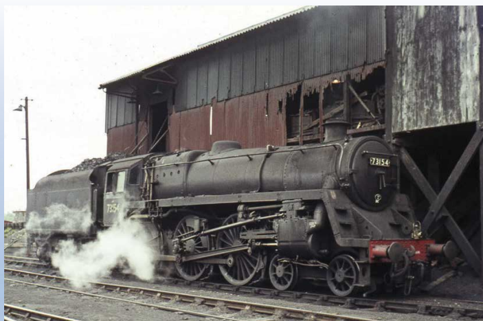
The Scottish-based Caprotti-fitted 5MTs seemed to find plenty of employment, and here the final one so fitted, 73154, is seen at Aberdeen Ferryhill shed on July 14th, 1965. It survived until December 1966. R K Greenhalgh/Colour-Rail.com
