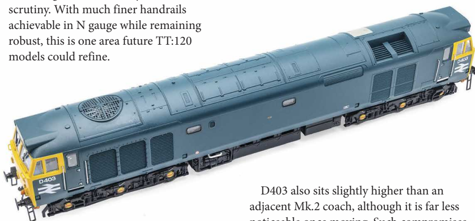
Roof panels are well-defined with fan detail visible through the grill.
