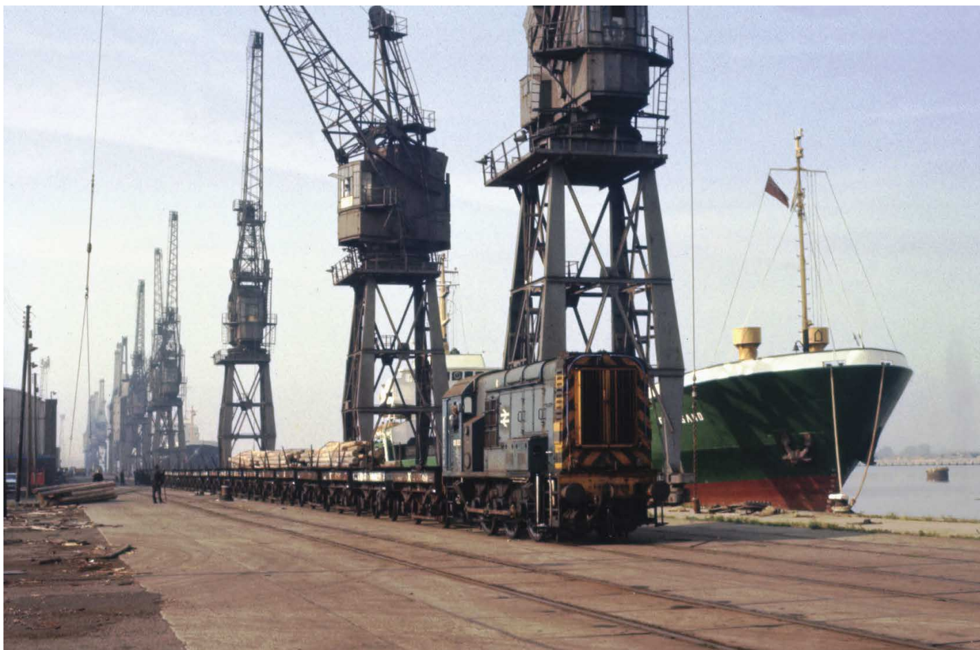
While not suitable for work at locations where very sharp curves abounded, the ubiquitous BR 350bhp Class 08 could also be found working at several docks around the country. 08822 waits on the quayside at Newport Docks as imported telegraph poles are loaded onto some of the dock's large fleet of internal user single bolster wagons during the late-1970s. TREVOR MANN COLLECTION
