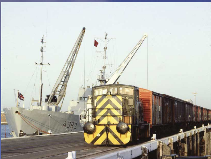
During the early 1960s, Ruston & Hornsby built 18 of its 275bhp Class LSSH 0-6-0 diesel hydraulics for the British Army. While only one was fitted with vacuum brake equipment, they were a success and were allocated to military bases around the country. Army 432, works number RH466623 built 1962, hauls a rake of BR vans along the jetty at Marchwood Military Port in June 1983; moored alongside is A382, the Royal Corps of Transport 1,393 gross tons general cargo ship St. George , which had been built at Appledore in 1981. DAVID RATCLIFFE
