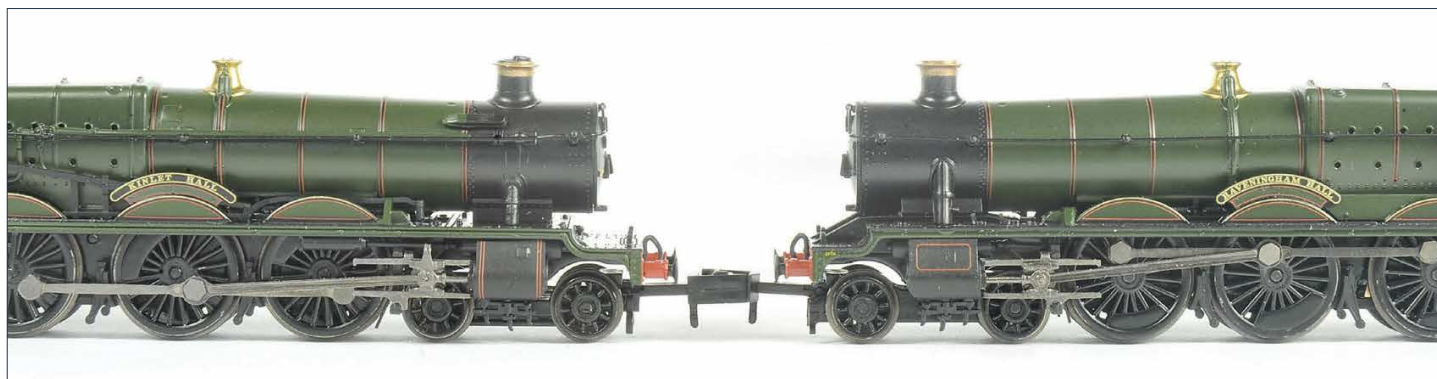
Nose to nose. The taller steam pipe and plate framing are clearly visible on the 6960 Modified Hall on the right.
