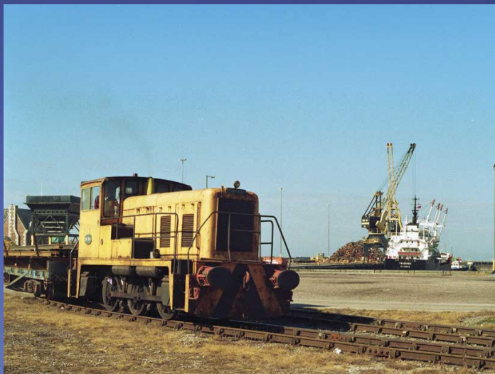
One of the four Yorkshire Engine Co. 300bhp 0-6-0 diesel hydraulics built for Richard Thomas & Baldwin, works number YE2832 of 1962, shunts at Workington Docks in September 1997. All four of these locomotives had been transferred from Llanwern steelworks to the Moss Bank Works at Workington in the early-1970s under the auspices of the British Steel Corporation. In the background, the 4,000-ton ship Trademed waits to be loaded with export steel rails bound for Nigeria. DAVID RATCLIFFE
