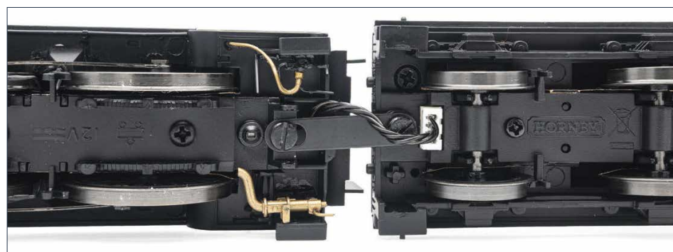
Electrical connection is via a tender socket.
