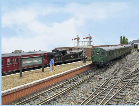
TOP LEFT: A 2-EPB electric multiple unit made from Worsley Works brass etches arriving into the station as the steam-hauled push-pull train awaits departure.
