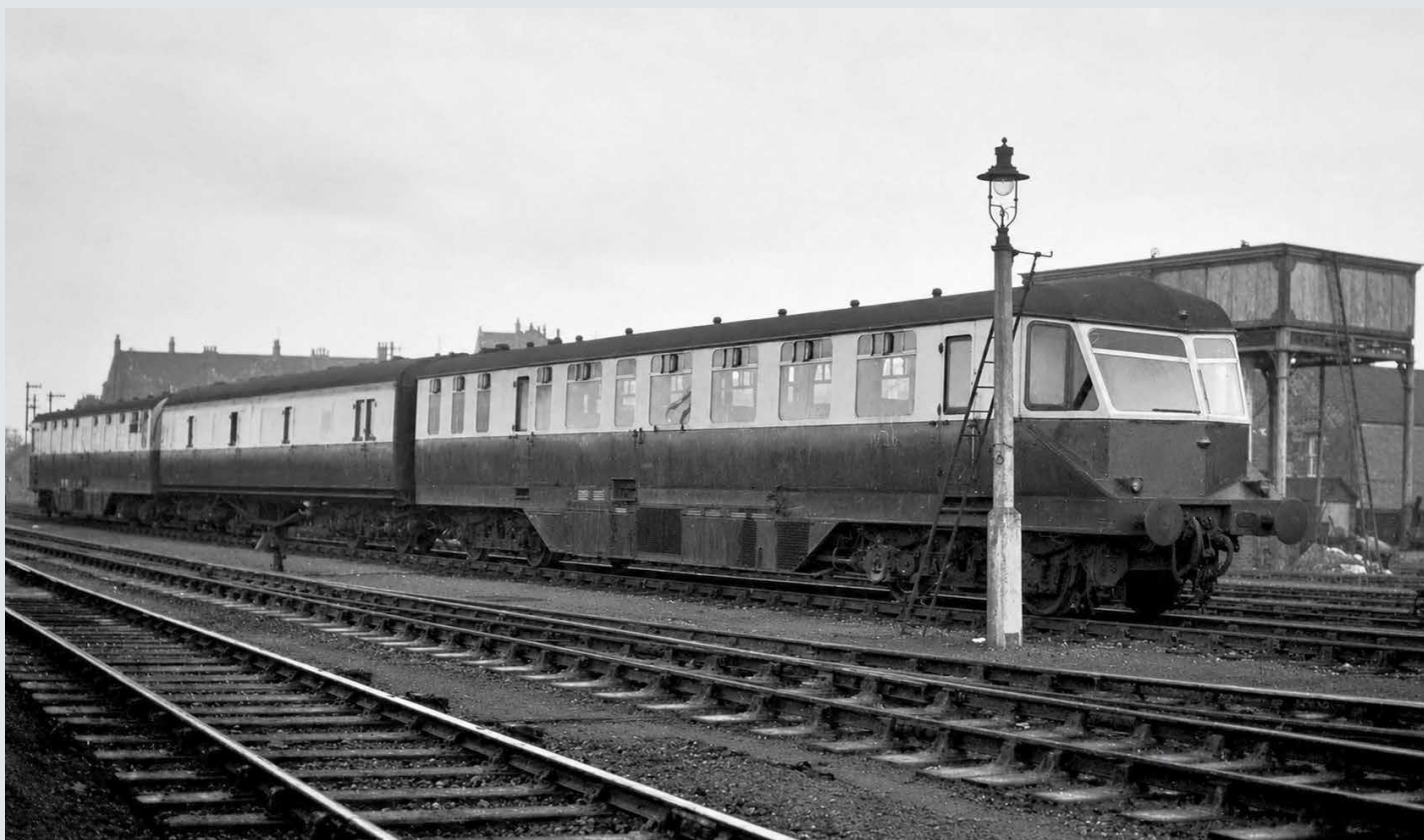
Stabled outside Weymouth station between Bristol runs in 1950 are W35 and W36 with a through-wired hauled coach between them; W36 is nearer the camera. These railcars were vacuum-braked and one had a steam heat boiler on board. It was a pair like this that startled the author in 1944.
