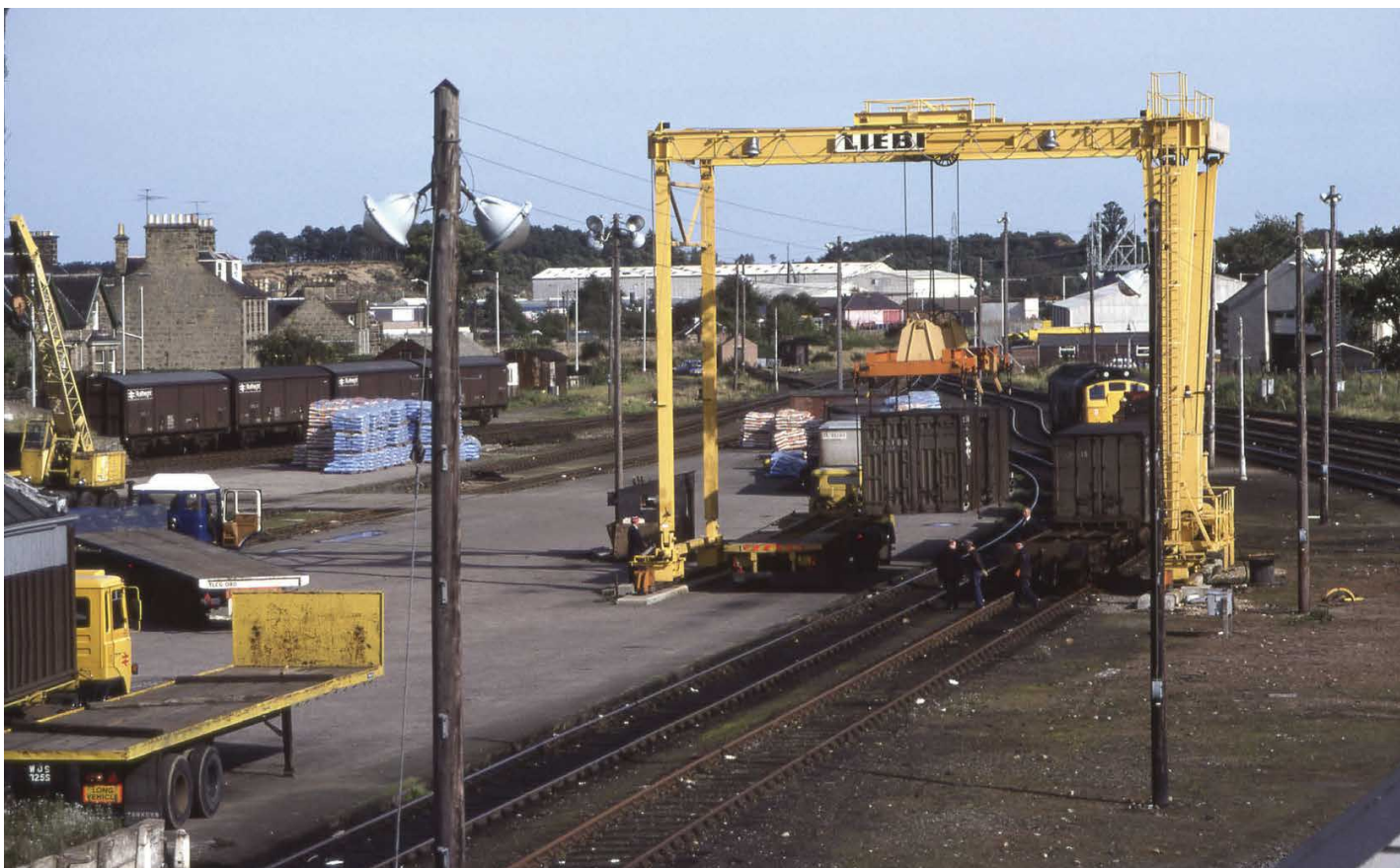
Elgin East was an unusual example of a BR goods depot with a fixed gantry crane for lifting containers. An empty whisky container is transferred to a waiting lorry on September 25th, 1980, as 25230 ticks over with a short rake of air-braked wagons. The crane saw intermittent use until 2013 and was demolished in April 2018.
