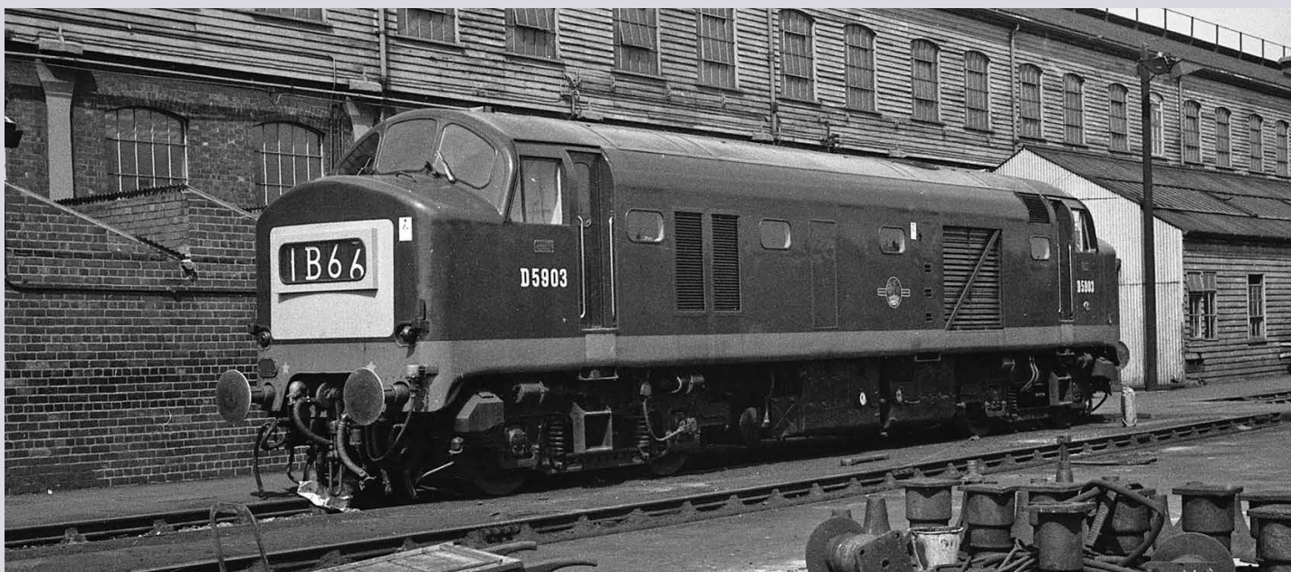
D5903 looks very smart and presumably has just been released from Vulcan Foundry in 1964 following its rebuild with a new engine, probably being sent to Doncaster, where this picture was taken, for acceptance back into stock. It now sports a red band all around the body, and four character headcode panels have been fitted surrounded by some nice yellow paint. Ultimately, the cost of rebuilding was probably never recovered as the loco was in traffic for just four further years. P MOFFAT/ COLOUR-RAIL.COM
