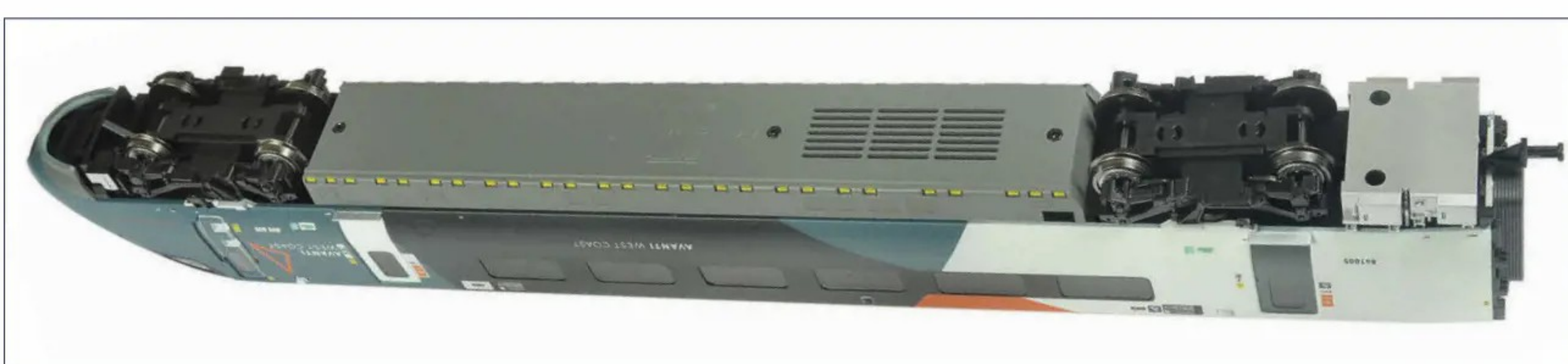
Underside view showing the three screws that release the fairing, giving access to the DCC socket.
