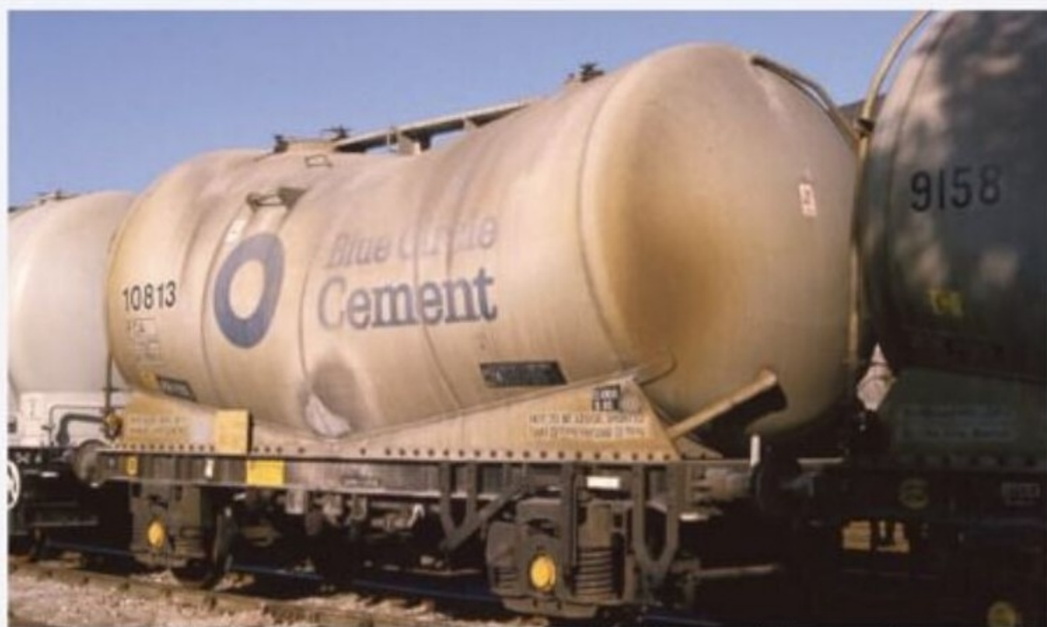
PCA No. BCC 10813 was sporting full 'Blue Circle Cement' lettering when recorded at Earles Sidings, Hope, in October 1985. Built at BREL Ashford Works in 1980, it is unusually fitted with a handbrake lever, most likely the result of a repair following accident damage, as no record of this modification appeared on the BR diagram. TREVOR MANN
