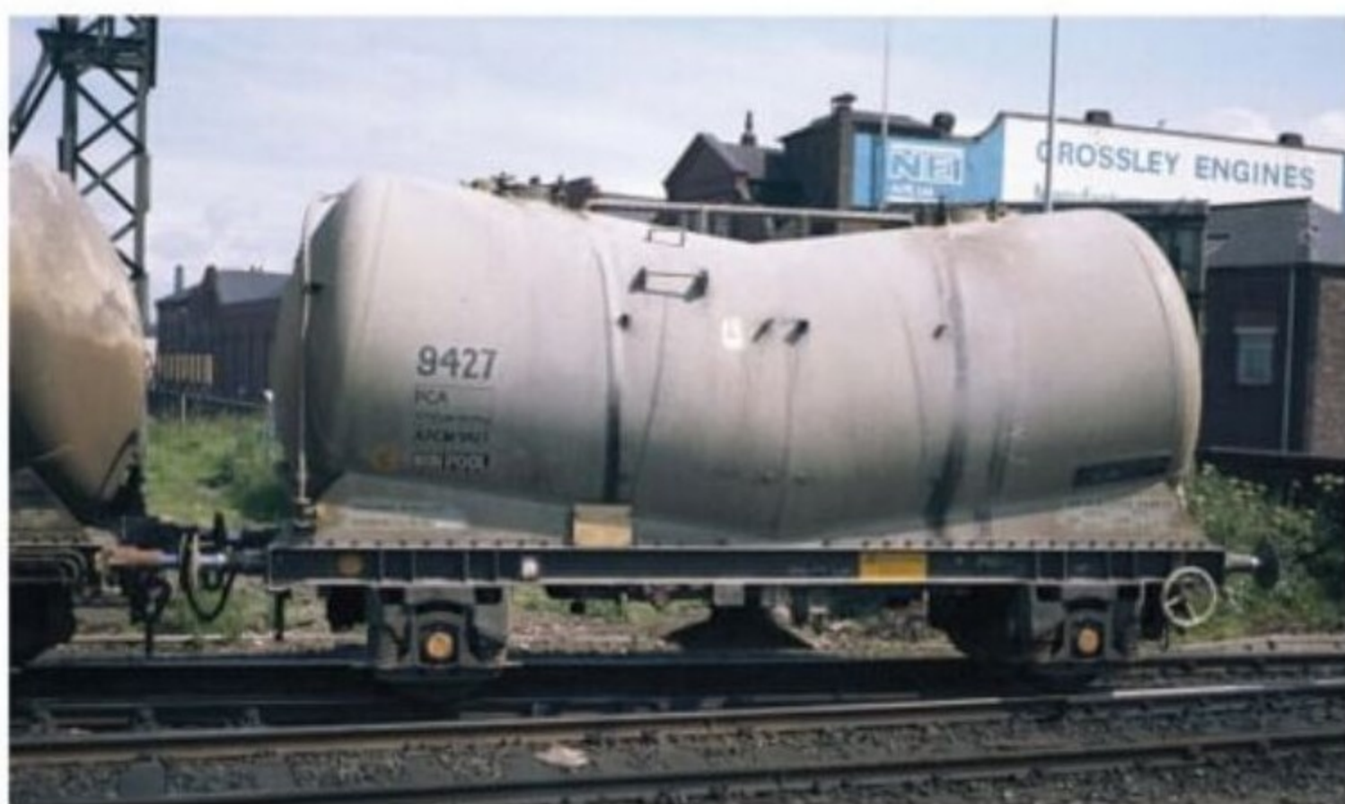
APCM 9427, one of the PCAs built at BREL Doncaster Works in 1974, was also spotted at Ashburys in July 1985. This view illustrates the opposite side of these wagons from that which carried the pipe runs along the solebar. DAVID RATCLIFFE
