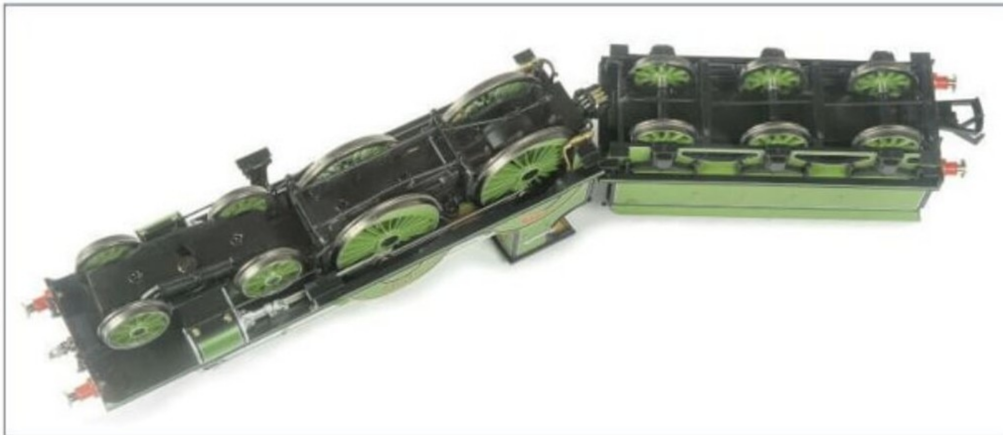
Pick-ups on all drivers and tender wheels ensure no stalling.
