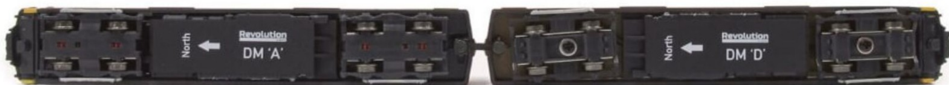
Underside view showing the simple bar coupling and removable panel for access to the DCC socket.
