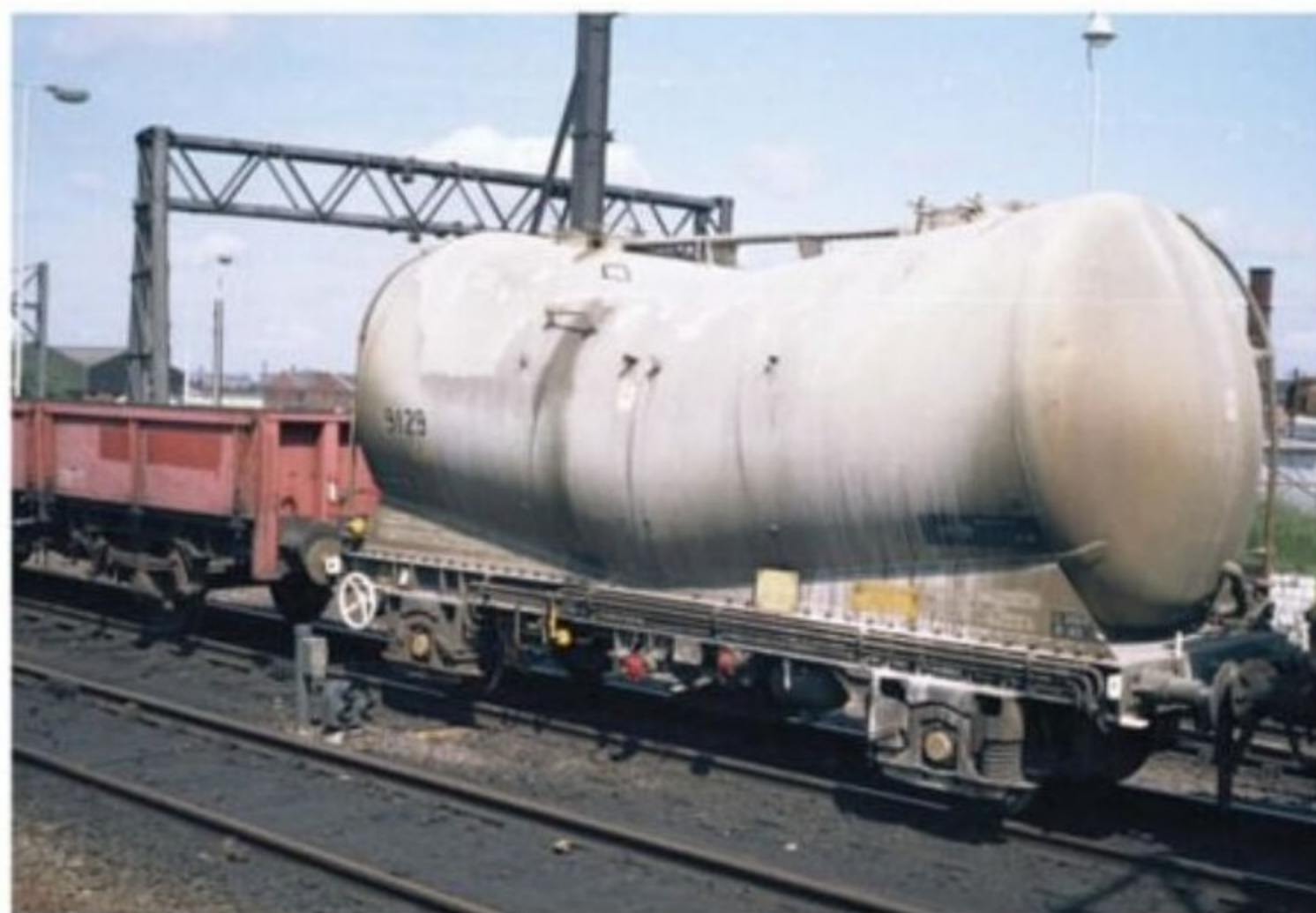
PCA APCM 9129, built by BREL in 1973, now with its original name boards removed but with the fixing brackets still in place, is seen at Ashburys in July 1985. DAVID RATCLIFFE
