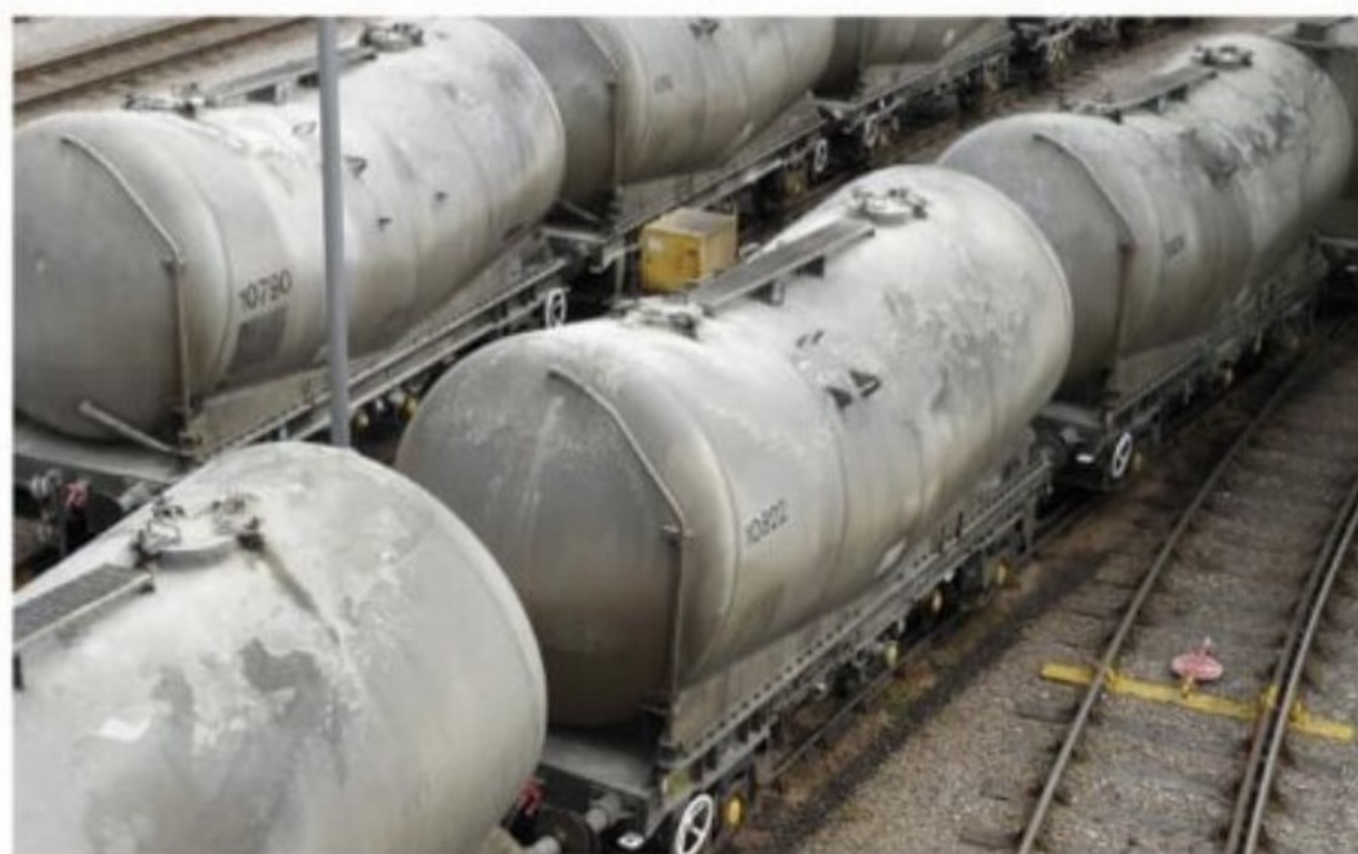
Although the APCM/BCC depressed-centre PCAs had no ladders, a short catwalk was provided between the two filling hatches on top of the barrel, as seen in this view of BCC 10822 recorded at Hope Cement Works in June 2019. DAVID RATCLIFFE
