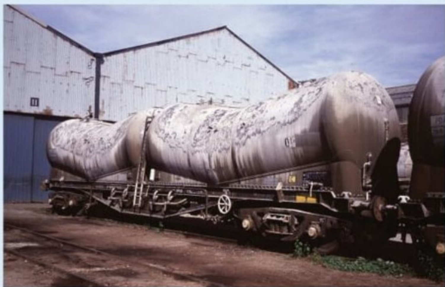
The PDAs lost their name boards in later years, while their last use in cement traffic was from the Blue Circle works at Claydon to Sizewell. 11 were allocated to that flow from spring 1988 until autumn 1991, among them APCM 9536, which was recorded awaiting repair at Stoke Wagon Works in September 1990. DAVID RATCLIFFE
