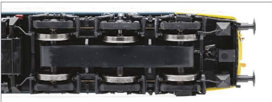
There are pick-ups from all wheels and a floating middle axle for excellent running.
