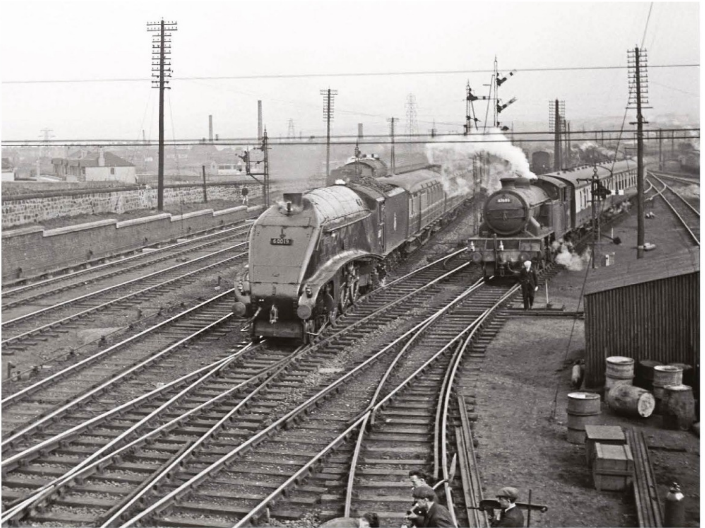
LNER A4 4-6-2 No 60019 Bittern with a down express passing Craigentenny carriage sidings in April 1953. D.T. Greenwood/Rail Archive Stephenson
