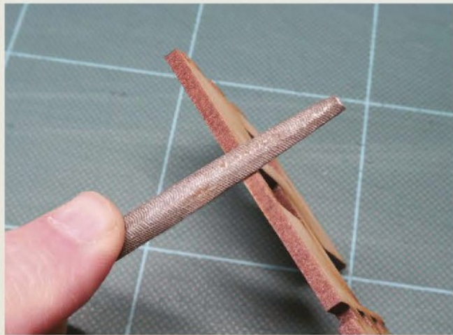
2 The wall parts simply 'pop' off the fret with a little thumb pressure. Two or more tiny tags are left on the part. To ensure a good fit, I carefully took these off with a small file.
