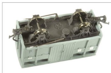
Underside view showing the simplified, but effective, brake detail.
