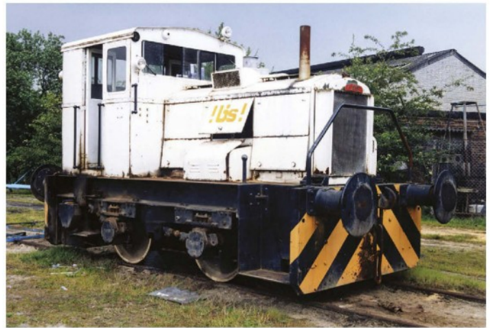
In 1958, Hibberd & Co. introduced an improved variant of the 6SC 'Planet', which had recessed steps located at the front on which the shunter could ride in safety. Ballast weights could also be added between the wheels below the frame, bringing the overall weight up to 23 tons. Works number FH4006 is pictured at Holmethorpe Sidings, Redhill on June 8th, 1991, when owned by British Industrial Sand. COLIN WRIGHT/DAVID RATCLIFFE COLLECTION
