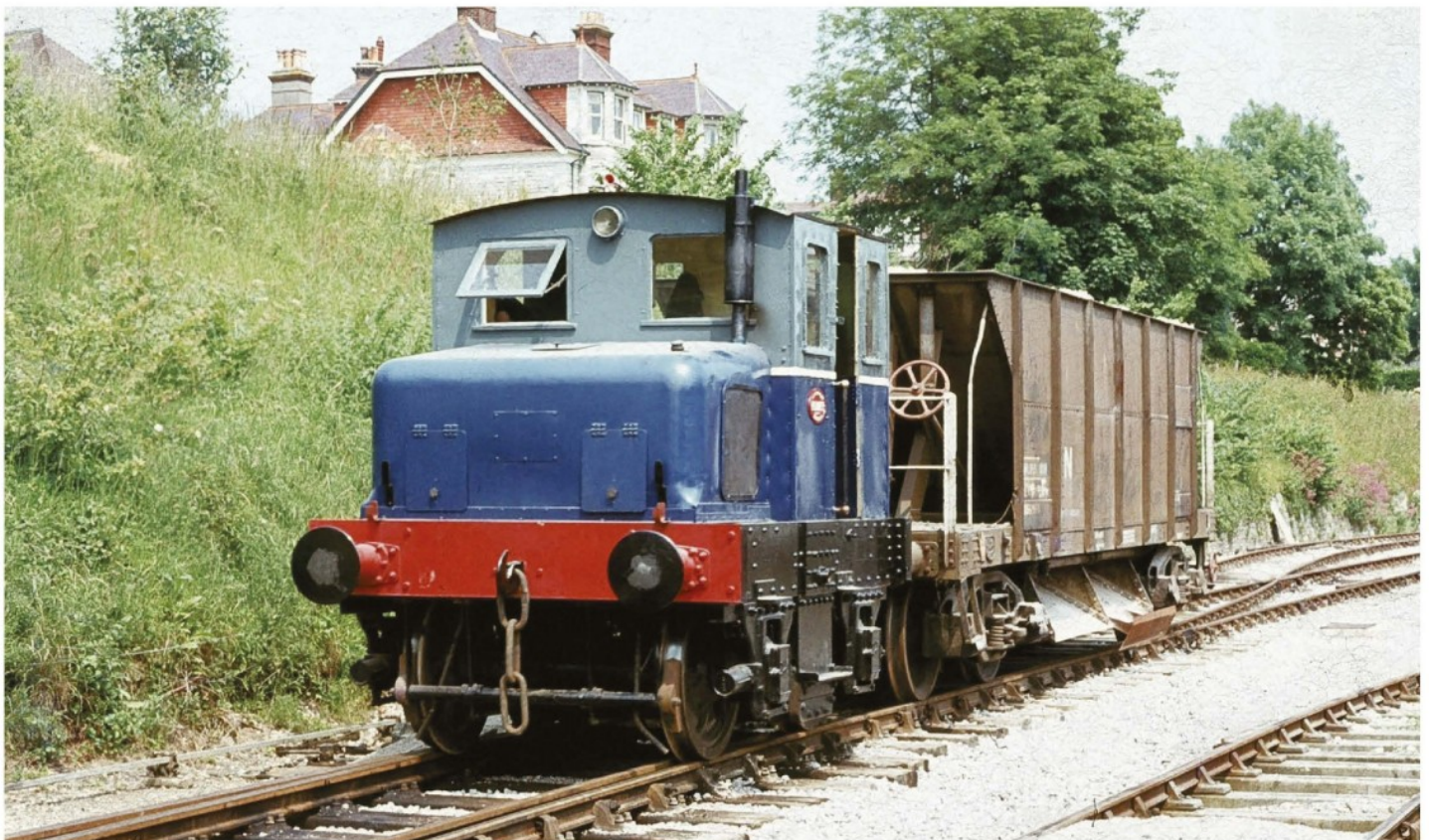
F. C. Hibberd & Co. built a range of petrol and diesel mechanical locomotives at Park Royal between 1932 and 1948, the petrol designs having much in common with contemporary Motor Rail locomotives. They included works number FH2054 of 1938, a 4-wheel petrol-paraffin mechanical (4wPM) powered by a 54bhp Dorman 4JORX petrol-paraffin engine, which first worked for the Bournemouth Gas and Water Co. In 1966, it was acquired by Corral's for shunting its coal depot at Hamworthy Quay, while a decade later, the Hibberd, which had been named Beryl , was preserved at the Swanage Railway. As its first locomotive, FH2054 saw considerable use on track relaying trains during the early years of the heritage line, being recorded hauling a 40-ton ex-BR 'Walrus' bogie ballast hopper at Swanage on August 8th, 1983. DAVID RATCLIFFE
