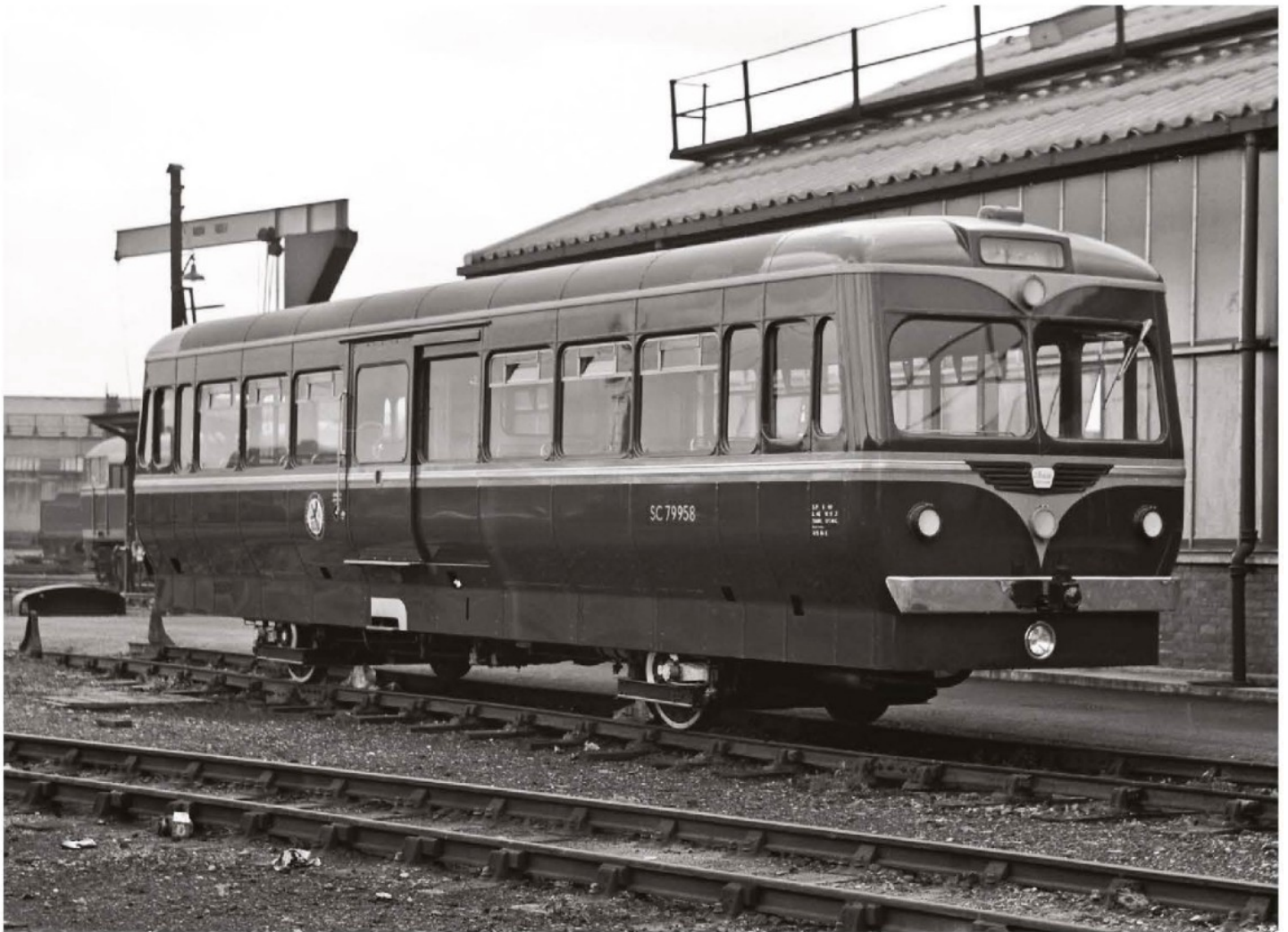
The first railbuses numerically were a pair of genuine 'buses', inasmuch as they were produced by the bus builder Bristol and were bodied by its partner Eastern Coach Works at Lowestoft. SC79958 arrived in June 1958, with the second machine following in November. 79958 was put on display at Marylebone from August 14-16th and had gravitated to Stratford shed by the 24th, where this picture was taken. It must have been an interesting trip to then work it up to Aviemore, which was its first allocation in September. Allocation changes were frequent but usually in synchronisation with fellow 79959. It was stopped for repairs in August 1964 and, despite an allocation to Inverness in August 1966, seems never to have worked again, being withdrawn the following October and swiftly cut up by T. W. Ward at Inverkeithing. COLOUR-RAIL.COM
