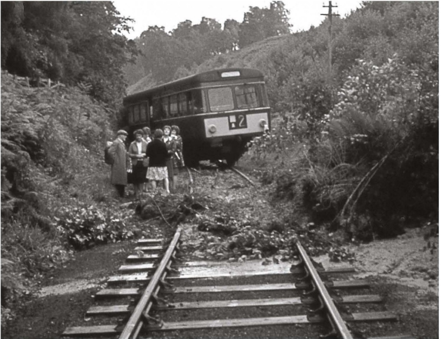
This picture illustrates the hazards of railbus travel, where a landslip has caused one to leave the track. It appears to have been a slow-speed derailment, as the unit has not travelled far beyond, looks unscathed and the passengers were able to walk away. SC79972 was the unit involved at Knockando in July 1963. 79972-4 had initially been allocated to Bedford but were soon all out of service and were subsequently moved to Scotland to join 79970/4, doing the circuit of the same sheds as the other Scottish railbuses, with the three officially classified as on loan from the LMR throughout. 79973/4 returned to the Midland in late 1965 and joined the Wickham units at Buxton, but survived less than 12 months, being cut up at Albert Loom Derby. 79970 was cut up at Ayr shed in March 1967, leaving 79971 to claim the most unusual demise of any BR DMU as its body was used as a C&W hut at Millerhill yard. When it came to disposal time, it was found to be contaminated with asbestos and so was wrapped in plastic and buried under 40ft of rubbish at Mount Vernon tip near Glasgow. COLOUR-RAIL.COM
