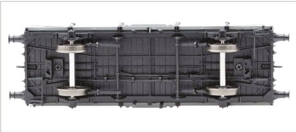
Brass bearings deliver smooth and wobble-free running.
