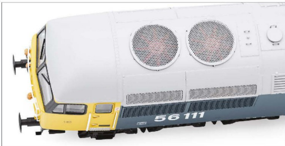
The twin fans have their own motors and spin when appropriate.
