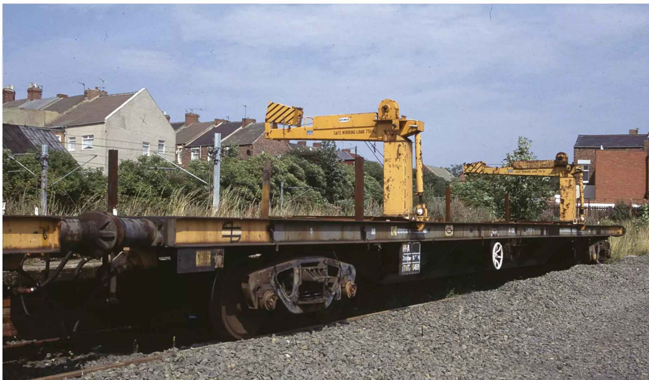
MA5 and MA6 were both fitted with dropside bodies for use as general material carriers, while MA8 had no fitments and was used to carry lengths of rail. MA3 and MA10 were equipped with Geismar rail loaders and, like the ballast hoppers and the dropside flats, could usually be found at Hylton Street, North Shields, with MA10 being recorded there in June 1991. MARK SAUNDERS
