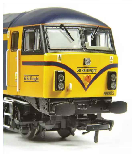
The DMU-style speed whiskers and new light clusters give the old Class 56 cab a new look.
