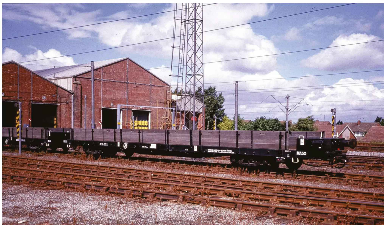
MA50 and MA51, the Metro's two purpose-built spoil wagons, were semi-permanently coupled with the outer ends being fitted with BSI auto-couplers. Their Westcode electronic brakes enabled them to operate with the Metrocars, but these unique features meant they were not registered for travel over BR tracks. The pair was recorded at South Gosforth in September 1986. DAVID RATCLIFFE
