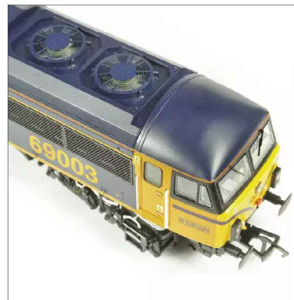
The new air intake and exhaust arrangements, necessary after the fitting of the new EMD 710 engines, on the roof of the Class 69 are superbly captured by Bachmann.
