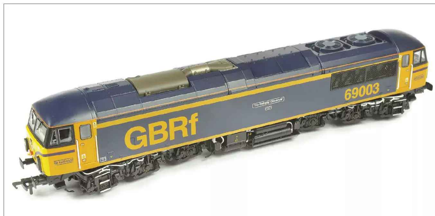
The new air intake and exhaust arrangements, necessary after the fitting of the new EMD 710 engines, on the roof of the Class 69 are superbly captured by Bachmann.
