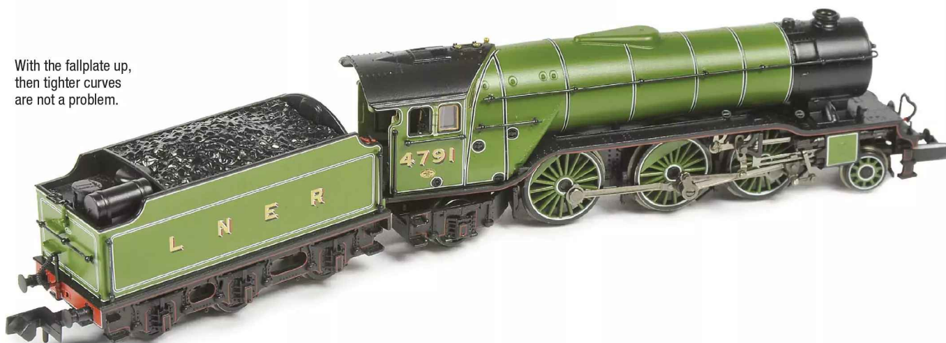
A full cab interior is present, but if you want the loco to go round tight curves, then the fallplate must be hinged-up.
