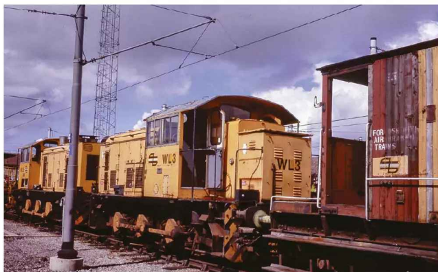
Tyne & Wear Metro 0-6-0 diesel electric locomotives WL3 and WL5, works numbers BT803/77 and BT805/77, await their next duty at South Gosforth depot in August 1987. DAVID RATCLIFFE
