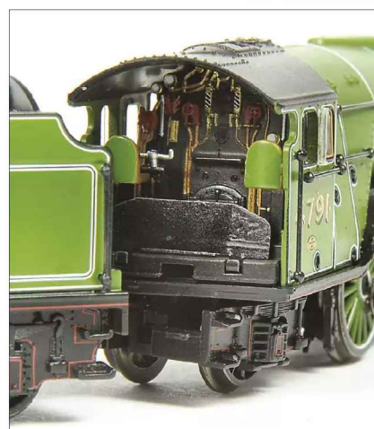
A full cab interior is present, but if you want the loco to go round tight curves, then the fallplate must be hinged-up.
