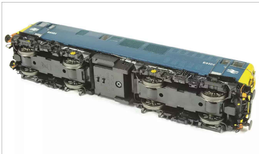
Underside view showing the light switches for DC users.
