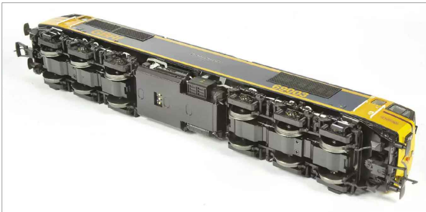
Underside view showing the three switches set into the fuel tank to allow independent control of the lights for DC users.
