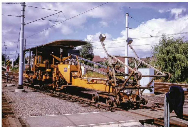
The Tyne & Wear's Switch electromagnetic ES/TD No.1976907, constructed by Tamber Inc. of West Columbia, South Carolina, and supplied by Matisa Ltd. is seen at South Gosforth in August 1987. DAVID RATCLIFFE
