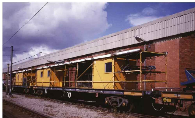
Three of the Metro's PFA flat wagons, MA2, MA7 and MA9, were fitted with frames for overhead line inspection work, with MA7 and MA2 pictured at South Gosforth in August 1987. DAVID RATCLIFFE
