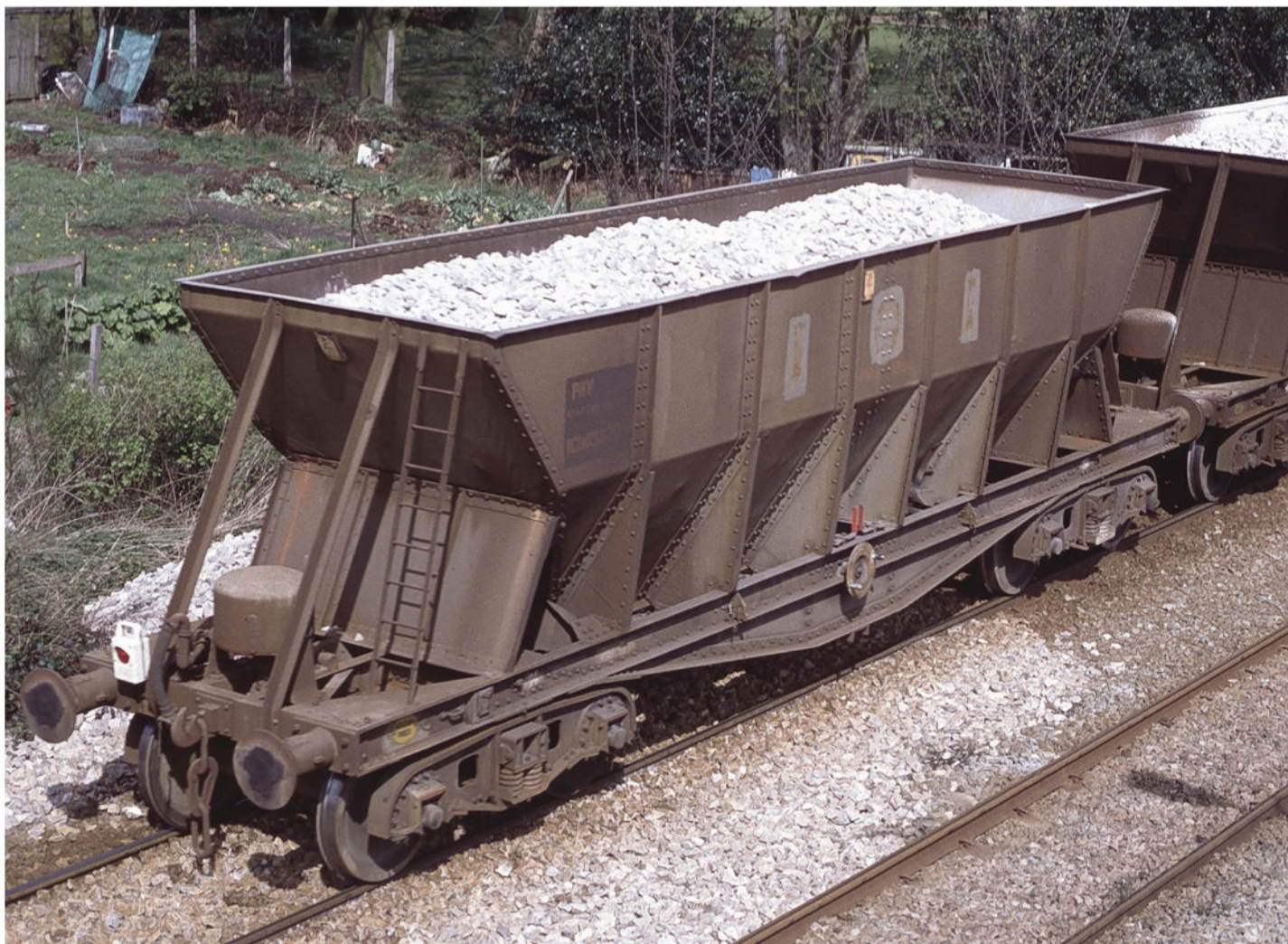
ICI Mond PHV No. ICIM19022 had just arrived with limestone from ICI's Tunstead Quarry when recorded at Oakleigh Sidings, Northwich, in April 1993. This flow conveyed large pieces of high-grade limestone used by the ICI (later Brunner Mond) chemical plants situated around Northwich in the production of sodium carbonate, a chemical widely used by the detergent and glass-making industries. DAVID RATCLIFFE
