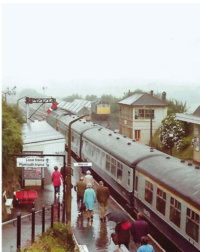
47455 has arrived at Liskeard with 1E21, the 10:21 Penzance to Leeds. 25207 is in the down sidings with clay hoods. Note the bracket signal with centre pivoted arm and was the only one like it in Cornwall. There can't be many stations in the UK with a branch platform at right angles to the main line platforms. The Looe branch goes off to the left but cannot be accessed from the up main. August 22nd, 1978.
