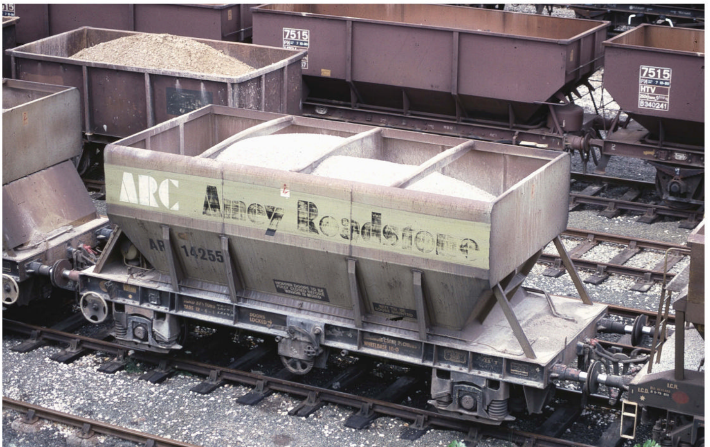
The most common aggregate load conveyed by rail during the last half century has been crushed limestone, with considerable tonnages having been transported to receiving terminals situated in many of the country's major conurbations. Depending on its grade and size, limestone can appear either white through to various shades of grey to light brown, as seen in this view recorded at Stoke Gifford, Bristol, in July 1980. In the foreground, Amey Roadstone Co. No. AR14255, carrying finely crushed stone, was one of a rake of PGAs en route from ARC's Tytherington Quarry to their hopper-discharge equipped terminal at Wolverton, while the vacuum-braked MSV wagon behind, which had also been loaded at Tytherington but with a coarser grade of limestone, was destined for Oxford.
