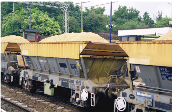
Construction sand from the Tarmac siding at Marks Tey, alongside the Great Eastern Main Line, was a regular traffic until recent years, being railed to several different terminals in the Greater London area. ZFA No.DC390570, an ex-Procor PGA modified with a cut-down body, is seen at Marks Tey when en route to Hayes & Harlington in July 2000. DAVID RATCLIFFE
