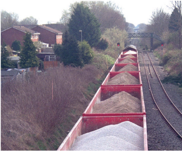
Although most aggregate traffic has been railed in block trainloads, there can sometimes be a range of grades of material conveyed in different wagons within a consist. Such was the case with this Class 66-headed Hindlow to Theale working, formed of bogie MMA open wagons, seen at Northwich South Junction in April 2017. DAVID RATCLIFFE
