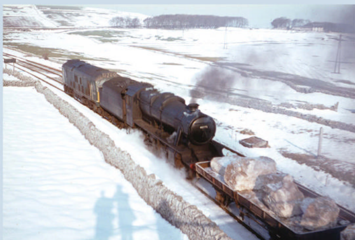
The most eye-catching of stone traffics, although admittedly the least common, is the movement of very large blocks and boulders used for the building of flood defences. On a snowy February 17th, 1968, a BR Type 2 pilots Stanier 8F 2-8-0 No. 48775 away from Hindlow Quarry, Derbyshire, with a special freight formed of BR Plate wagons conveying limestone blocks. TREVOR MANN COLLECTION
