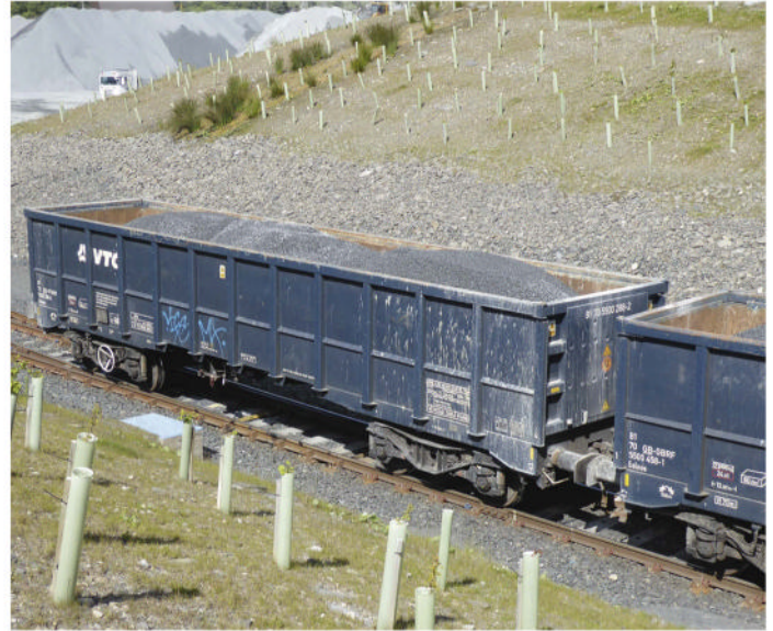
Tarmac's Arcow Quarry, next to the Settle & Carlisle line, generates a considerable tonnage of railborne gritstone traffic, much of which is used in road construction. Shovel-loading of the JNA wagons used from here usually produces an even load, as evidenced by this view of No. 81705500288-2 leaving Arcow Quarry for Scunthorpe in July 2019. DAVID RATCLIFFE
