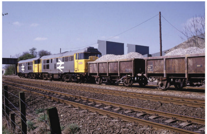
The use of vacuum-braked wagons in aggregate traffic declined during the 1980s as more air-braked vehicles were introduced, but they could still be seen carrying crushed granite for use as ballast from the quarries at Croft and Mountsorrel in the 1980s. A pair of Class 31s shunts a well-loaded train of MTVs at Croft in April 1988. TREVOR MANN COLLECTION
