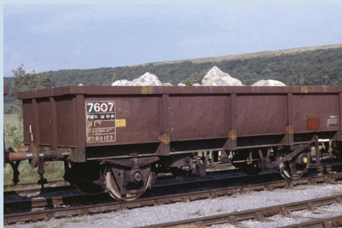
The Foster Yeoman limestone quarry at Merehead has also been the source of large limestone blocks, often referred to as 'rock armour', used for sea defence repairs at various locations around the south west of England. MTV No. B390123 waits to leave Merehead with such a load in September 1981. The large number '7607' on the side was the pool to which the wagon was allocated; its more usual task being to convey roadstone from Merehead to Fareham. TREVOR MANN COLLECTION
