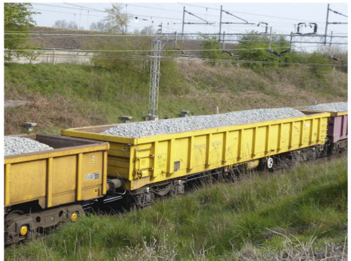
Today, new railway ballast is moved in both low and high-sided air-braked bogie wagons, such as GBRf MLA No. 503039, seen arriving at Crewe Basford Hall from Mountsorrel in April 2019 and March 2022. DAVID RATCLIFFE
