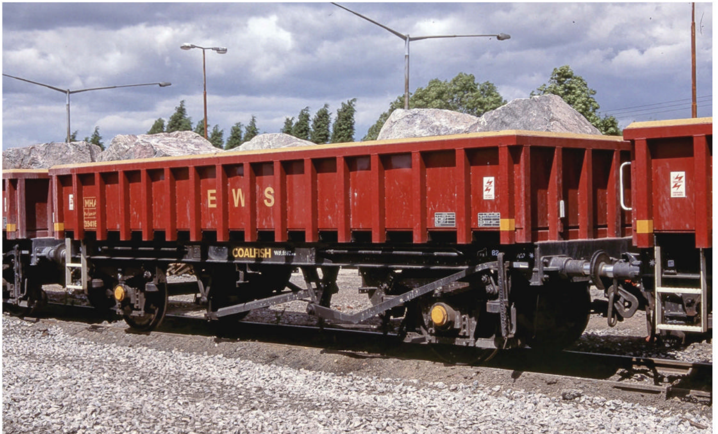
MHA No. 394164, loaded with large blocks of granite, is pictured at Bardon Hill Quarry in July 1998. The blocks were destined for Hessle, where they would be used to help protect the railway line between there and Ferriby from the encroaching River Humber. DAVID RATCLIFFE
