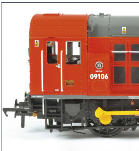
The excellent spring, brake and sanding details are all separately applied fittings.
