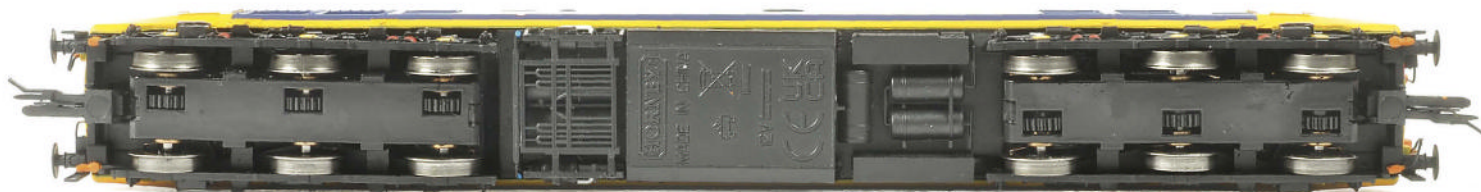
Underside shows attention to chassis details and all axle drive.
