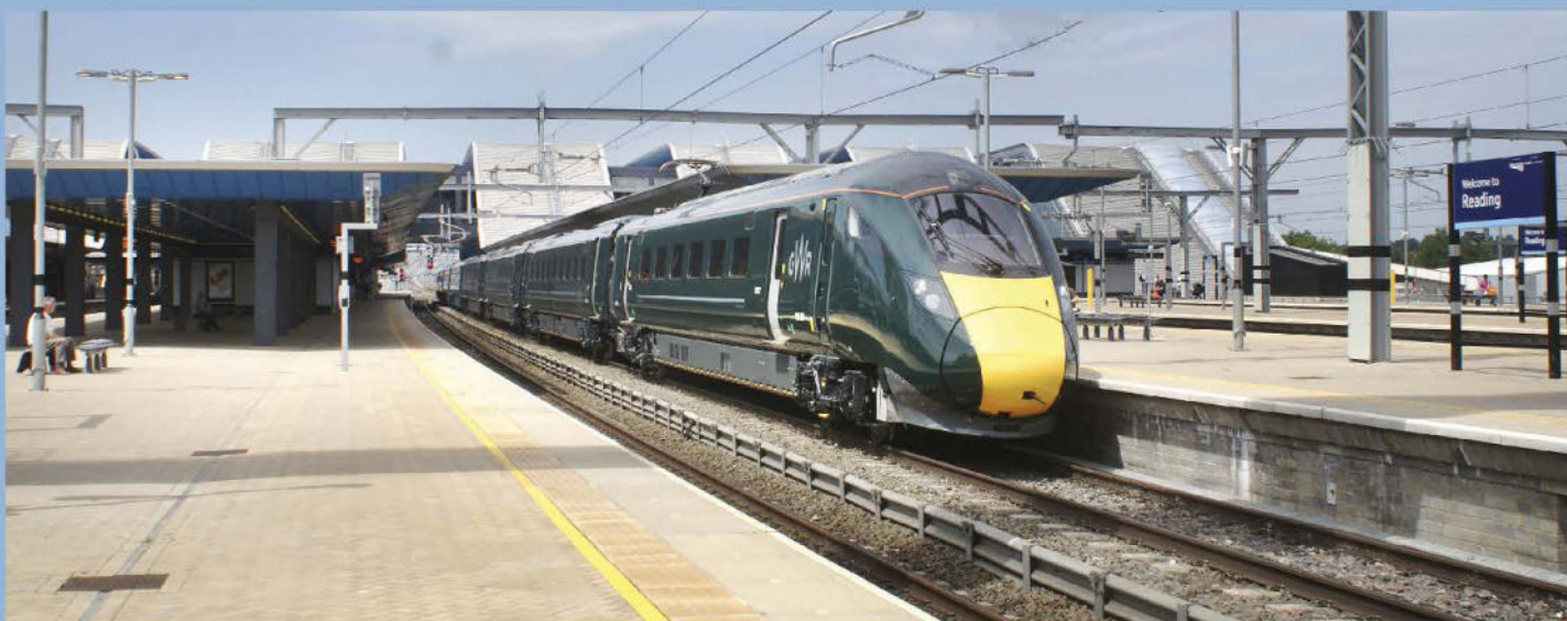
A modern example of a unit train is the Hitachi 800 series of InterCity Express trains. Because of the curtailment of the electrification programme at the outer ends (no wires up in Bristol Temple Meads or Swansea), all the GWR 800-series units are bi-modes, diesel and electric. A nine-car set is seen leaving Reading on an up service to London Paddington on July 4th, 2018. COLIN BOOCOCK
