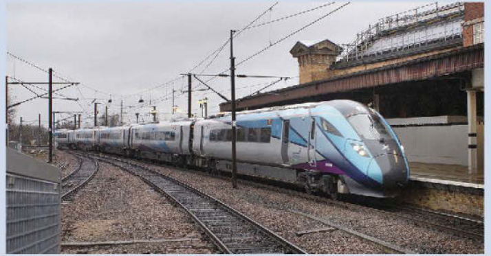
Arriving at York and already switched to diesel mode is bi-mode Trans-Pennine Express unit 802206 on a Newcastle to Liverpool service on December 6th, 2019. Sound insulation on these trains is good, making the noise of their diesel engines less intrusive both inside and outside the train. COLIN BOOCOCK
