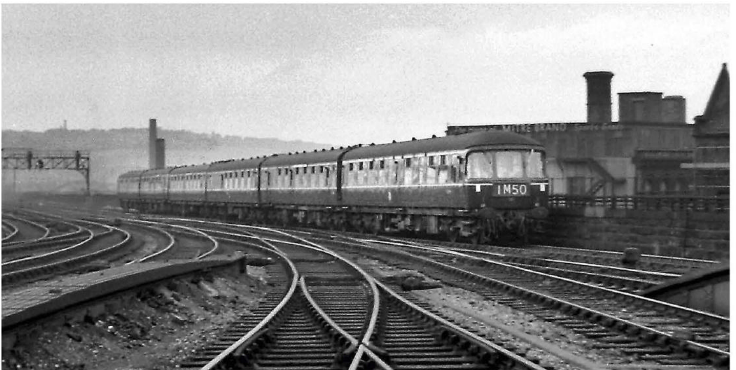
Introduced in 1960, the Trans-Pennine DMUs were six-car sets on 63ft 6in underframes and dubbed as Inter-City units even though their maximum speed was only 70mph. They included a buffet-griddle car; the catering car was later removed from each set due, apparently, to lack of demand. COLIN BOOCOCK
