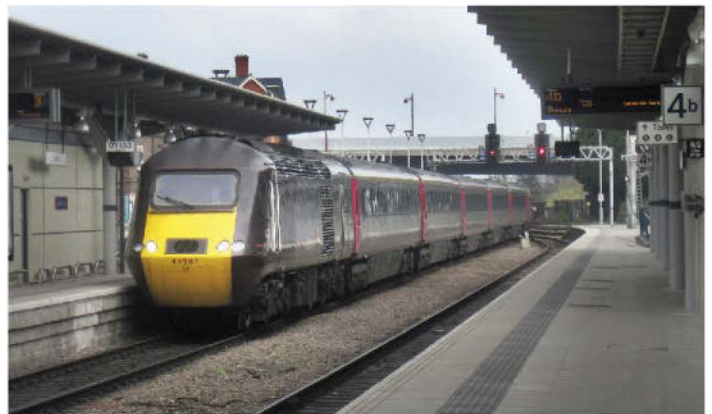
The 1970s saw firstly the prototype and then the first production trains of the High Speed Diesel Train concept, soon known as HSTs and also more formally as InterCity 125s. They were built as seven and eight-car sets, early ones with two catering cars (buffet and restaurant) but these were soon reduced to one catering car in each set. 95 HST units were built and they rescued the reputation of the InterCity business and of British Rail as a whole. This one arrives at Derby on April 2nd, 2012, on a Newcastle to Plymouth Cross Country service. COLIN BOOCOCK
