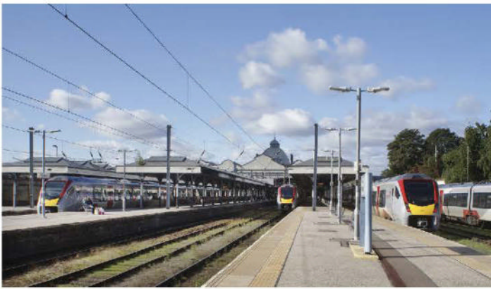
From left to right at Norwich on October 2nd, 2019, are brand new Stadler articulated bi-mode units (diesel and electric) of Class 755, Nos 413, 423, 409 and 417. These units have their power sections in short 'pod' vehicles, which have through walkways but do not carry seated passengers. As a result, the passenger areas are quieter than in units with under-floor engines. COLIN BOOCCOCK
