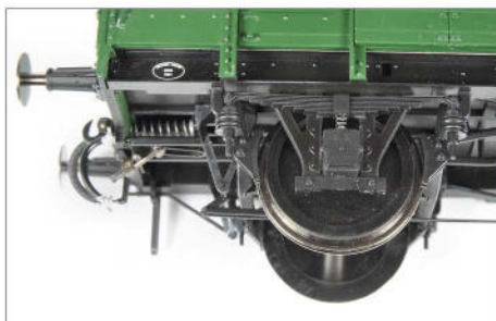
With the van on its side, the coil springs appear.
