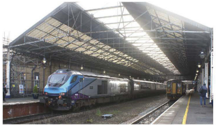
At the back of this TPE service from Scarborough to Manchester Airport, calling at Huddersfield on January 30th, 2020, is Caterpillar-engined 68023. These Mark 5 push-pull trains have been withdrawn, replaced by the older Class 185 DMUs that they originally displaced. This reduced the variety of TPE train types on long-distance services from four to three! COLIN BOOCCOCK
