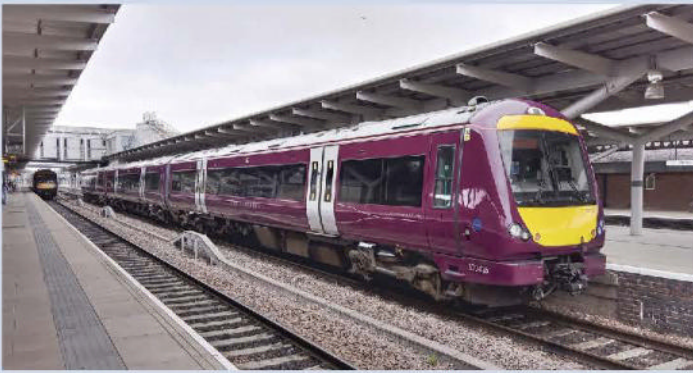
It only needs one of these Class 170 'Turbostar' units to stand with its diesel engines idling to make it hard to hear station announcements. This is 170416 between services at Derby on July 23rd, 2021, in what was then the new livery for East Midlands Railway. COLIN BOOCOCK
