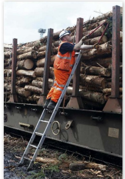
A little gardening is necessary to ensure that the train is within gauge. The wagon is a KFA converted from a Tiphook ferry van and the scene was recorded at Carlisle on July 19th, 2011. PAUL SHANNON
