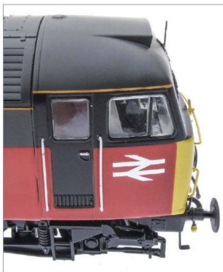
The prominent radio aerial on top of the cab looks very fine but is a wire part that is very robust.
