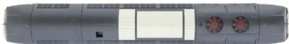
The large pale roof access doors are incorrectly modelled as two doors rather than four.
