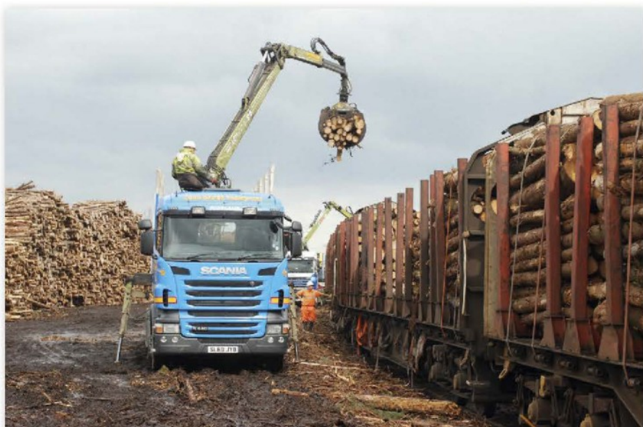
The timber being loaded at Carlisle on July 19th, 2011, comes in four set lengths – 2.5m, 2.8m, 3.1m and 3.7m – and each bundle of logs must be positioned behind at least two stanchions before being secured by two straps. Careful planning is necessary to ensure that the space on each wagon is fully used. PAUL SHANNON
