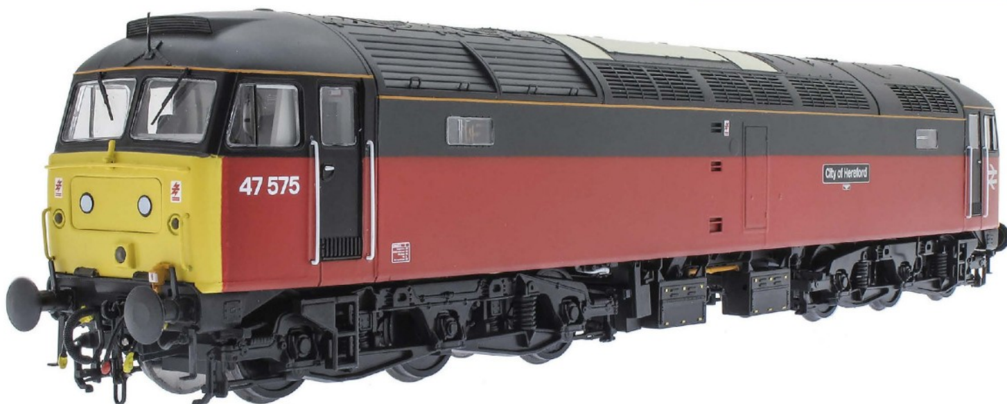
The large pale roof access doors are incorrectly modelled as two doors rather than four.
