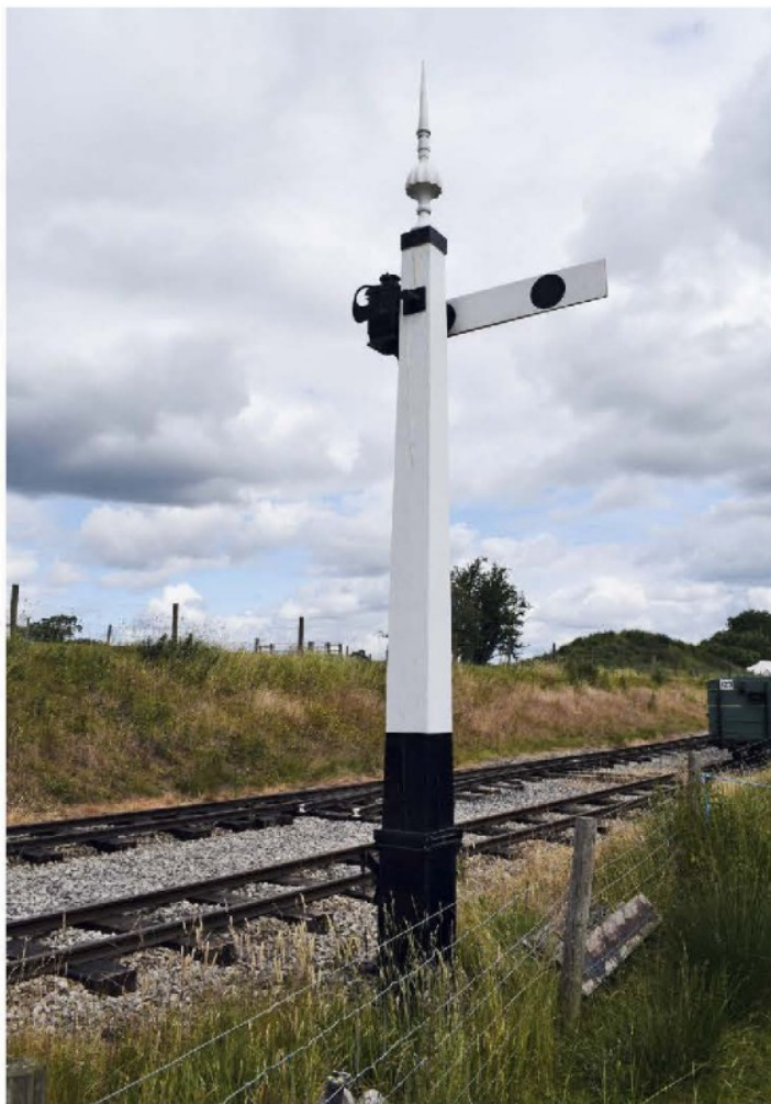
This lower quadrant McKenzie & Holland signal, supplied to the (NSR), circa 1880, now protects the station on the Amerton Steam Railway in Staffordshire. Note the taper of the timber post, cast finial and the arm with a black circle, as opposed to a black stripe, on its reverse side.
