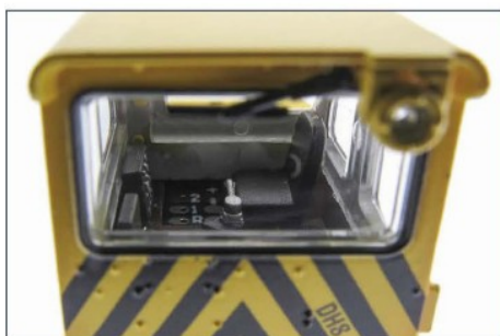
The view in the cab shows the seats and control panel sitting atop the circuit board.
