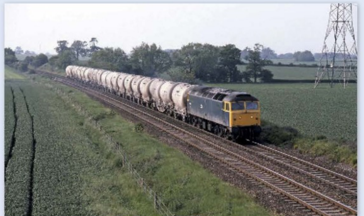
47328 is heading south at Portway with 6M18, the 16:05 Earles Sidings to Greaves Sidings cement wagons. The train is composed of fourteen PCA wagons and three bogie PDA wagons. 19th June 1986.
