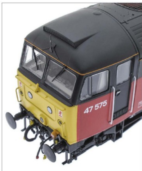
Excellent flush cab glazing gives a view into the detailed desk and bulkhead.
