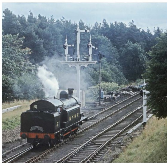
The North NER and Furness Railway (FR) both favoured slotted post-type signals as seen in this NER example captured at Goathland station on the North Yorkshire Moors heritage line. Lower-quadrant, with the posts widened at the slotted area, the earliest examples would feature arms that rotated to a vertical position, making them invisible in the 'go' position. Those in this illustration reflect later days when the arms were lowered by approximately 45°.
