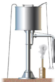
Typical Great Central Railway column mounted round tank with 'fire devil'.
