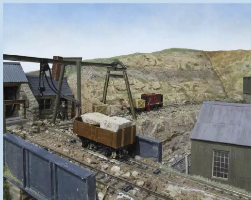
LEFT: A rope-hauled wagon incline, worked by an electric motor in the winding house, transports stone blocks from the quarry to the stone cutting works.
