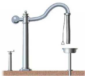
Typical North Eastern Railway water crane with valve handle and 'drip cup' mounted on pillars.
