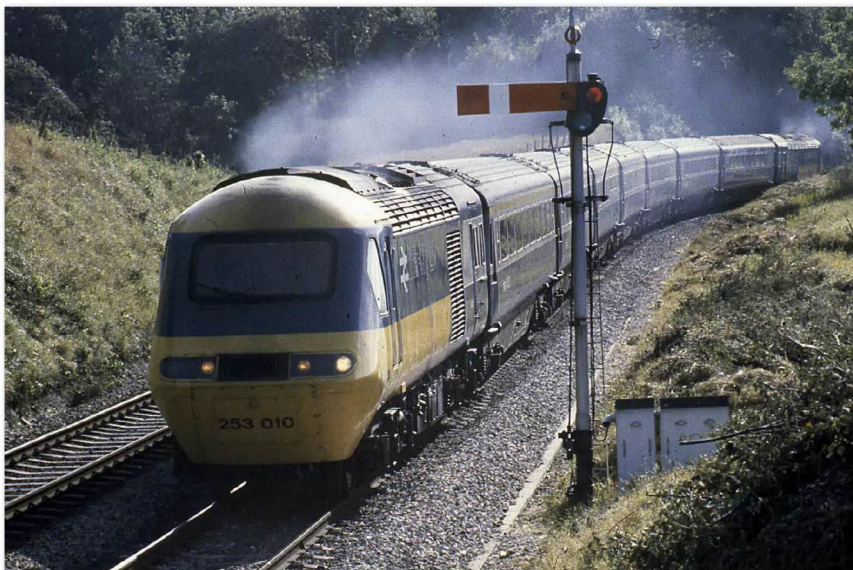
Set 253010 is working hard up Dainton bank on September 9th, 1980. The state of the exhaust suggests that fuel was not being burnt as efficiently as it should have been, the governor to fuel rack settings needed a bit of fine tuning. COLOUR RAIL
