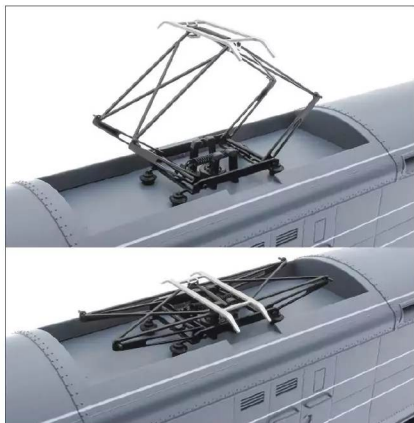
The sprung pantograph unclips easily, exerting very light pressure on overhead wires if they are below the extended height.
