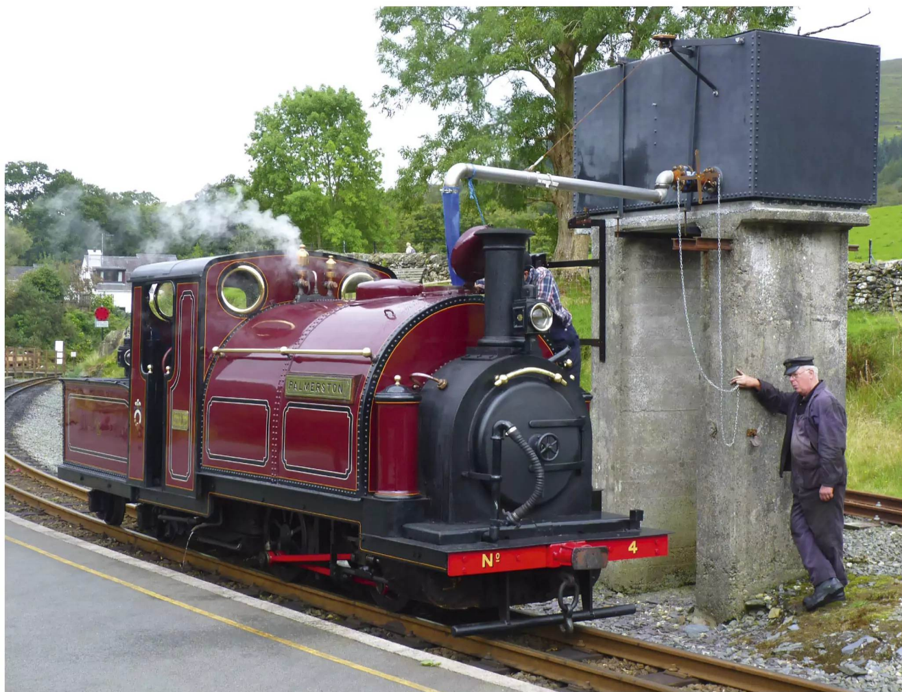
A 'brand new' water tower at Beddgelert, although the cast concrete supporting tower probably dates to original Welsh Highland Railway times. Note that a narrower diameter feed pipe is adequate to 'water' a narrow-gauge saddle tank locomotive.
