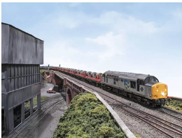
ABOVE: A Metals-liveried Bachmann Class 37/7 passes the loader with a steel train. This 37 is fitted with a Locksound decoder from Legomanbiffo and twin speakers, an EM1 in the fuel tanks and a standard 20x40 speaker under the fan.
