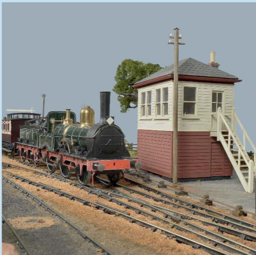
ABOVE: Cudworth 118 class 2-4-0 no. 246, one of the last built in 1874, threads its way over the three-throw turnout on its way out of the station. The model is scratch-built with homemade wheels and Stubbs gearbox and driven by a large coreless motor in the tender.
