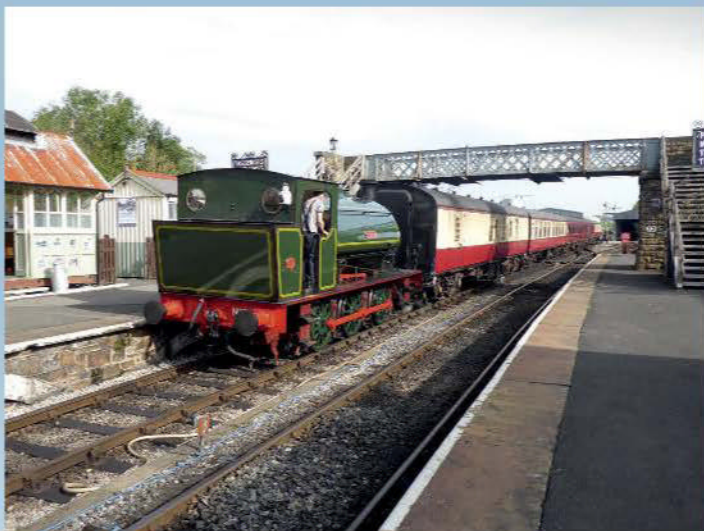
No.7 Beatrice , a beautifully-restored Hunslet built 0-6-0ST, w/n HE2705 built 1945, arrives at Embsay with the late morning service from Bolton Abbey on October 10, 2023. Prior to preservation, this locomotive had worked for the NCB at Ackton Hall Colliery, Featherstone, and is named after the colliery manager's daughter.
