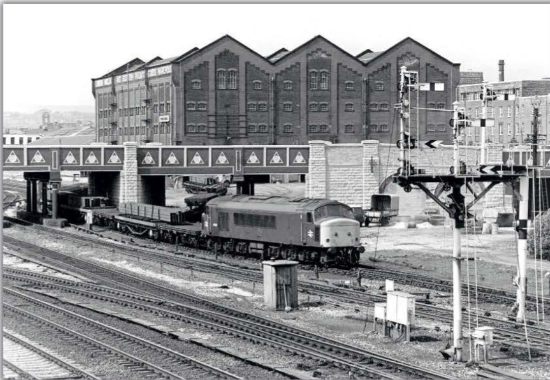
Bolton yard saw a resurgence in steel traffic after the closure of Halliwell goods depot in 1981. 45051 shunts loaded and empty wagons after arriving at Bolton with the Speedlink trip from Ashburys on 29th May 1984. Spacer wagons were necessary because the steel sections were longer than the BDA bogie bolster wagons that carried them. PAUL SHANNON
