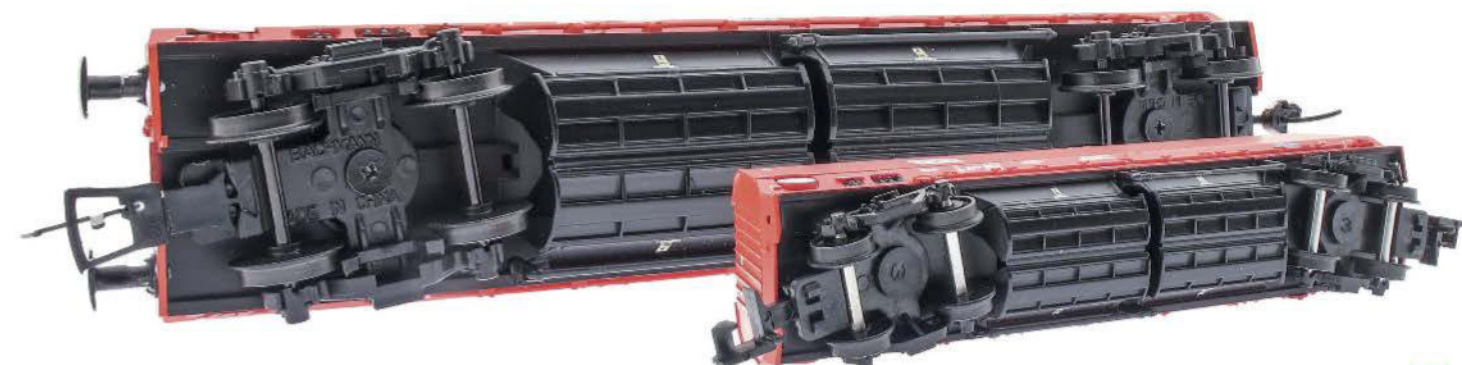
The underside of the HRA shows where the central hopper discharge chutes were abstracted from the earlier HTA.
