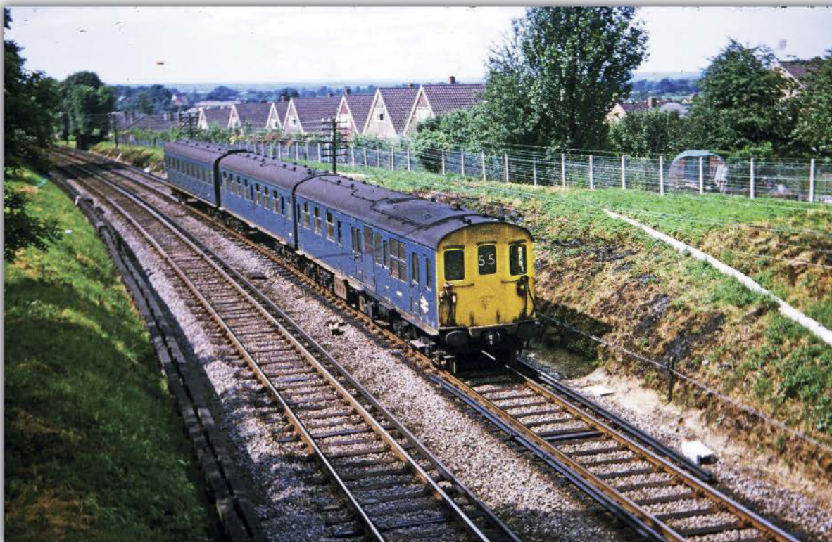
4SUB 4366 is north of Bagshot, by the side of the A322 where the line passes under the A30, and is working a Waterloo to Guildford service via Ascot and Aldershot. The unit was made up of Motor Brake Seconds Nos. 10917 and 10918, 10 compartment trailer No. 10172 and 9 compartment trailer No. 11469. The unit commenced service in March 1948 and appears to have led a trouble free life until withdrawal in February 1974. It was reinstated, but never used, and was sent for scrapping by A. King Ltd at Snailwell in October 1976.
