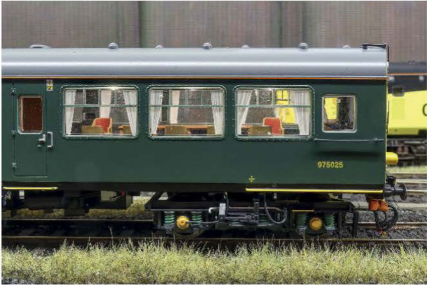
The excellent Caroline inspection saloon, produced by Revolution Trains, gets ready to move off. I modified the lighting by using black tape to cover the LED above the driver so that he is not lit as per prototype and also toned down the coach lighting by placing frosted draughting tape layers over the other coach lights. It helps to tone down the interior lighting.
