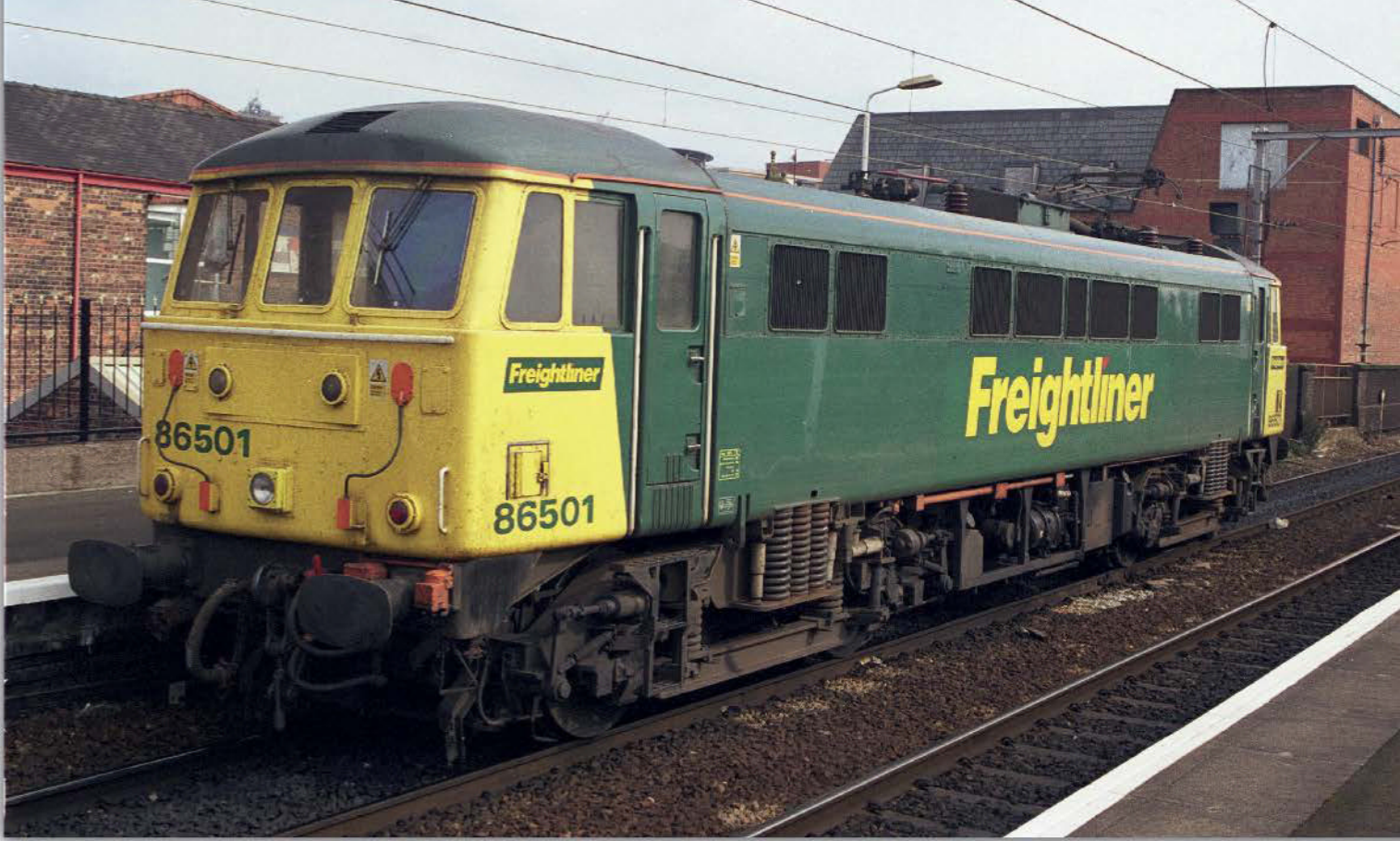
In Summer 2000 Freightliner's Class 86 No. 86608 underwent a trial conversion being fitted with revised gearing to provide improved tractive performance. Renumbered as 86501 the modified locomotive is pictured running light through Deansgate station on September 23rd, 2000.
