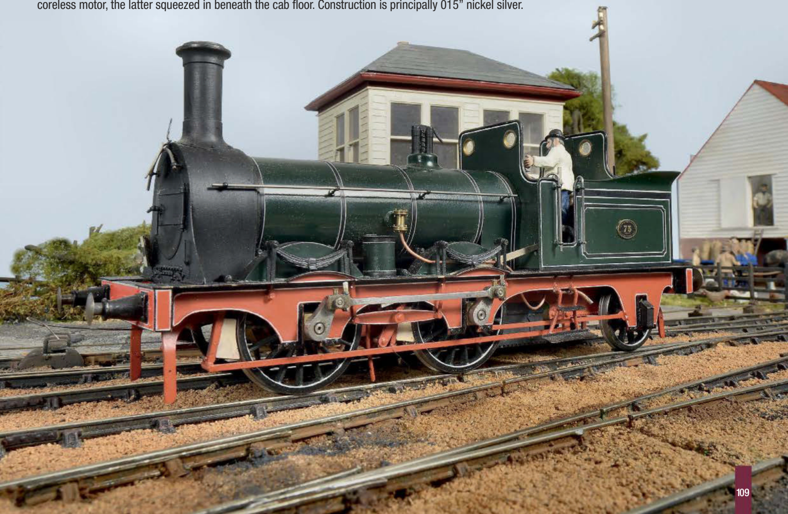
BELOW: 73 class 0-4-2WT as re-boilered by Stirling. These were essentially mixed traffic locos with 4'10" drivers though originally intended for London area freight work. The model has home-made wheels, Stubbs gearbox and coreless motor, the latter squeezed in beneath the cab floor. Construction is principally 015" nickel silver.
