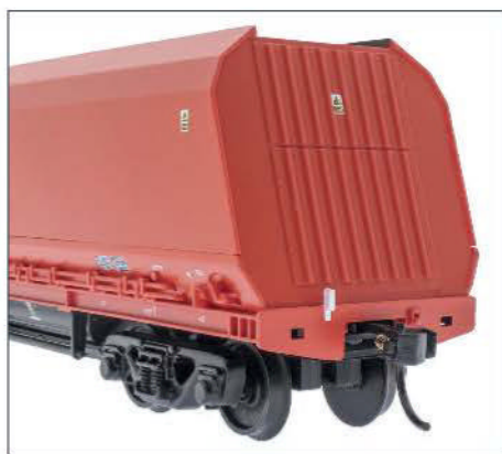
The Bachmann USA E-Z Mate sprung knuckle coupling is a good solution for inter-rake coupling; note the absence of buffers at this end.
