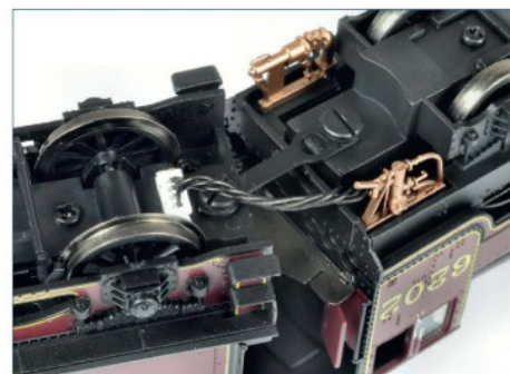
As supplied, the drawbar is in the 'long' position; the screw to adjust it also holds the rear of the loco's body in place.
