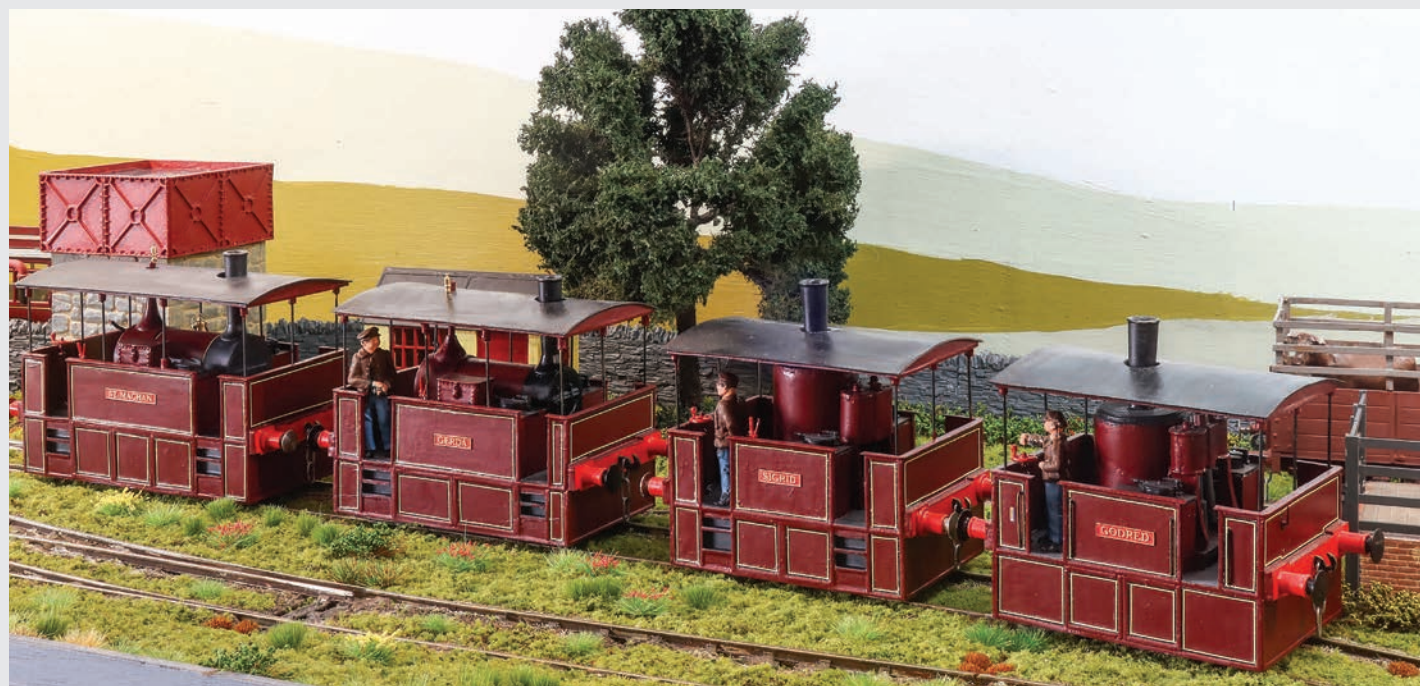
ABOVE: From right to left, we can see Nos. 1 to 4, showing the evolution of the design. The coffee pots Nos. 1 and 2 ( Godred and Sigrid ) operated the tramway for the first few years. After traffic increased, No. 3 Gerda , a slightly larger horizontal boiler locomotive, was designed. The ultimate design stage is No. 4 St. Machan , a chunky six-coupled locomotive designed for handling the heaviest services on the tramway.
