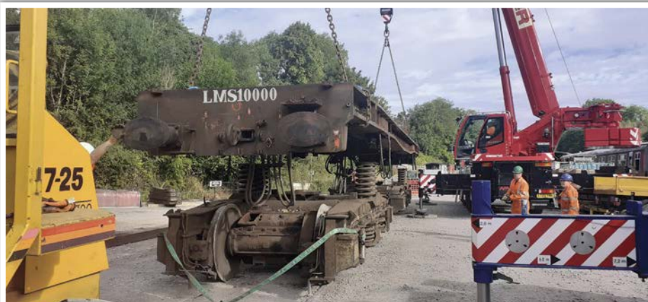
The big lift in August 2022 sees 58022's frames lifted off its bogies. IDRS
