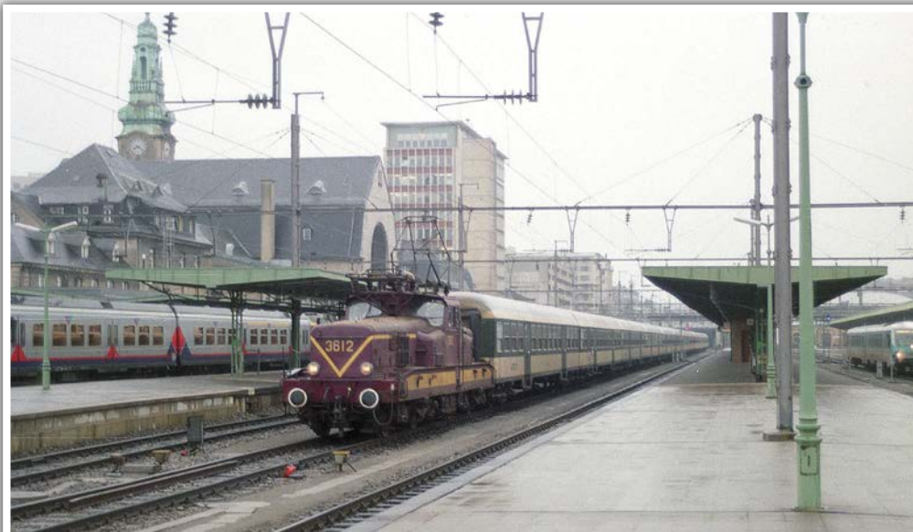
On the wet morning of 26th April 1998, centre-cab Bo-Bo 3612 stands in Luxembourg station with a long train of Wegmann coaches after arrival on a morning commuter train. To the right is a SNCB AM80 EMU for Brussels, and far right a DB class 628 DMU arrived from Trier. COLIN BOOCOCK
