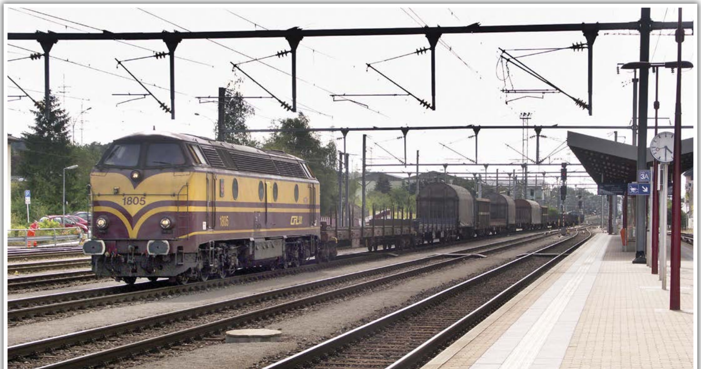
The fine-looking B&N Co-Co diesel electrics of class 1800 were based on SNCB's class 55. They were used mainly for freight, but also hauled passenger trains on the line towards Liège in Belgium until that was electrified. No. 1805 was passing Petange on 10th August 2006. COLIN BOOCCOCK
