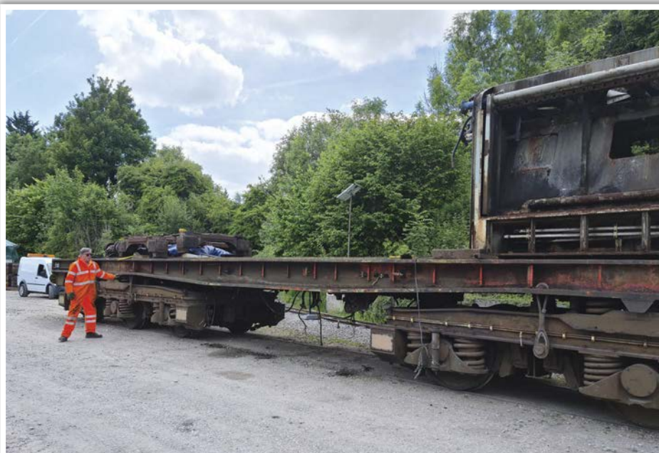
By the 14th June 2022 58022 has been stripped except for cooler frame and the number 1 end cab. IDRS
