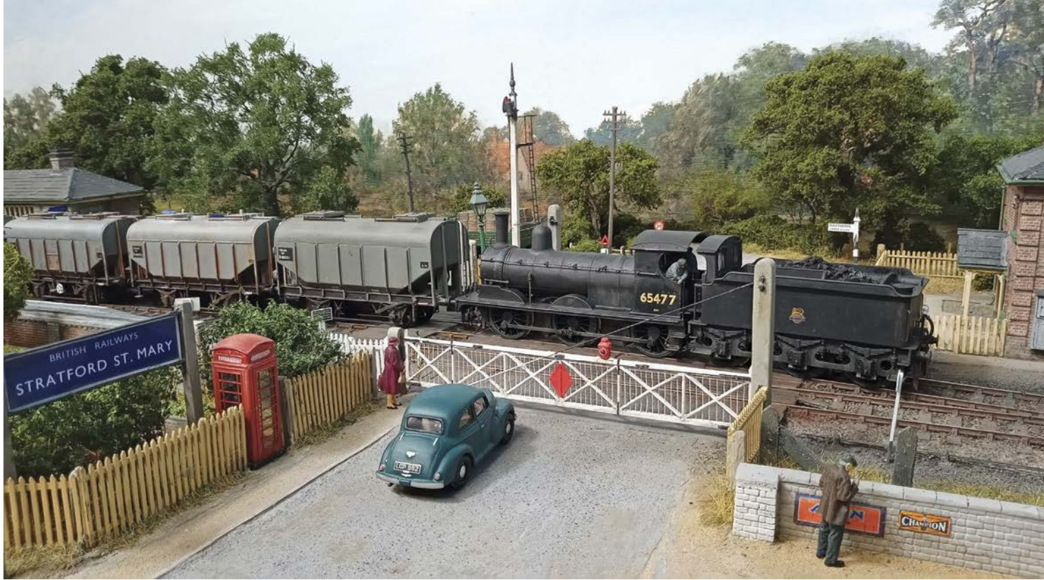
65477 eases a train of grain wagons over Dedham Road crossing. The leading vehicle is an Acorn etched brass kit, the remainder are Bachmann. The brass crossing gates, tapered along their length, with delicate infill rods and working lamps, represent Great Eastern designs adapted for use with concrete posts.
