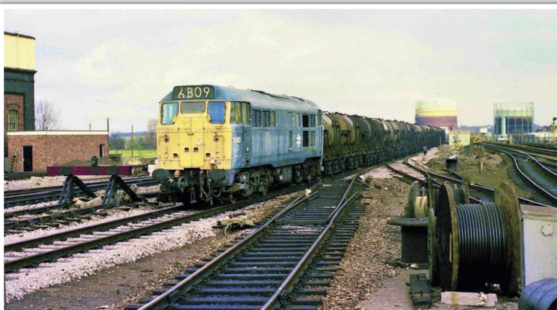
Saturday 5th April 1975: Possibly standing in for a 'Western' diesel hydraulic, 31412 approaches Reading with 6B09, the 15:47 SO empties from Acton Yard to St. Erth (arr. 06:55 Sun). This service was interesting in that it called at Swindon to attach loaded milk tanks and also made additional calls elsewhere, as described in the article. Judging from the paintwork, the Brush Type 2 looks as though it's been through the Old Oak Common carriage washing plant a few times! STEPHEN BURDETT (with thanks to Adrian Nicholls for service details).
