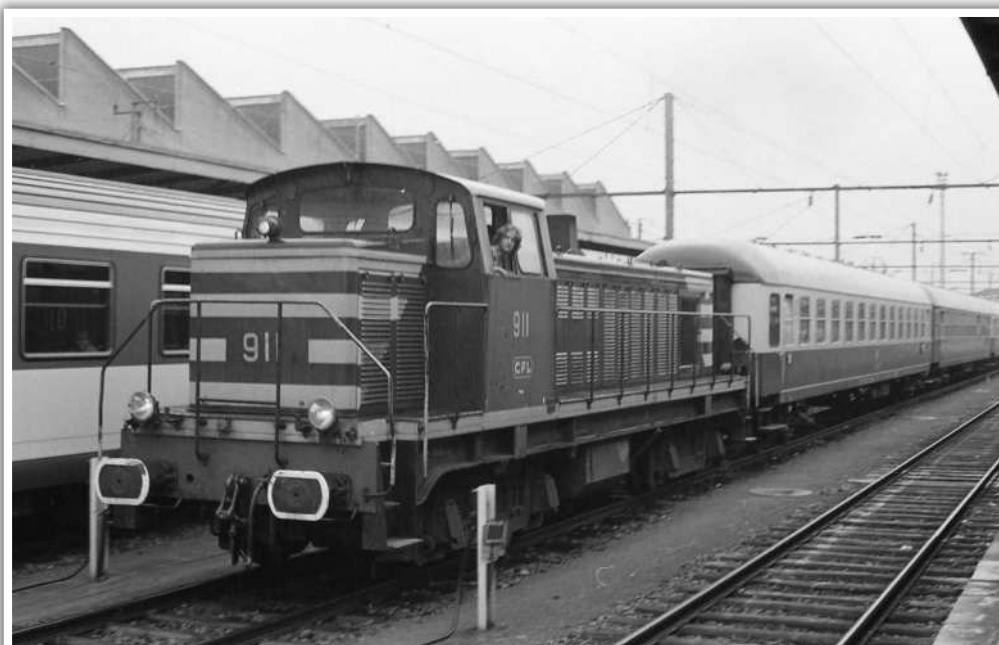
The second batch of thirteen Brisonneau et Lotz Bo-Bo diesel electrics were more powerful at 900 bhp with the locos being delivered to CFL in 1958. No. 911 is shunting the empty stock of a train from Koblenz in Germany after arrival at Luxembourg on 31st July 1982. STEPHEN RABONE
