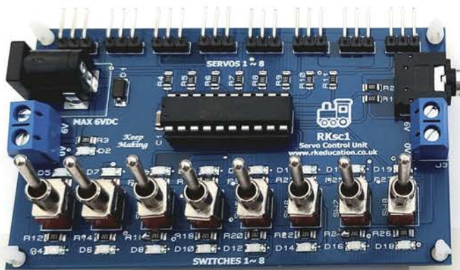
Control 8 servos with the RKsc1
