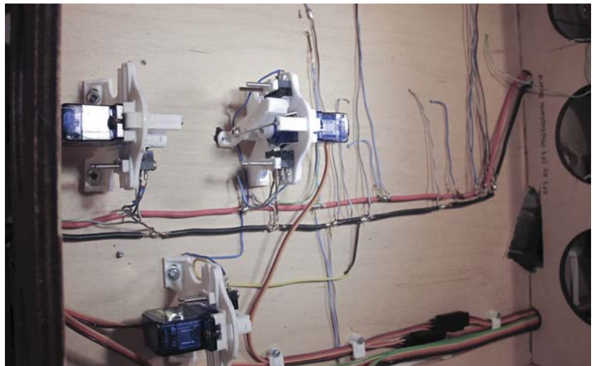
Servo-operated turnout with two microswitches
