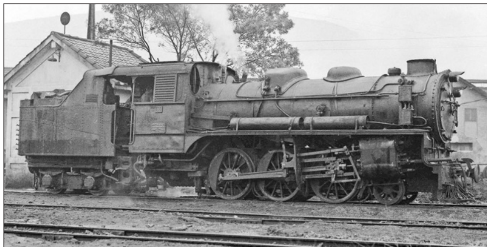
Below: Displaying its Giesl ejector chimney, no PV16 – the final Engerth built by Macosa in 1956 – is at Ponferrada.
