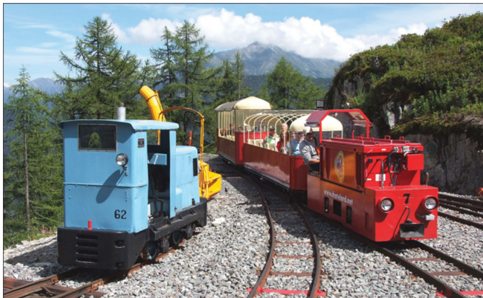
Facing page: Les Montuires station, more than 1800 metres above sea level and the start of the 600mm gauge line to Pied de Barrage. Battery loco no 7 is running round its train.
