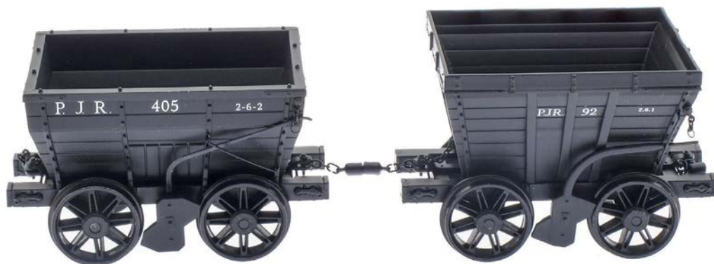
The 'greedy boards' fitted to the right-hand wagon expanded the Chaldron's carrying capacity as well as displaying differences in the planking and doors.
