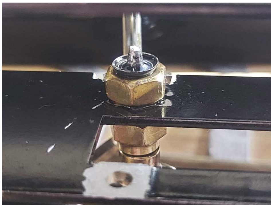
Shortened expansion link pivot to fit the inside frames.
