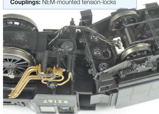
The modified close-coupling arrangement.
