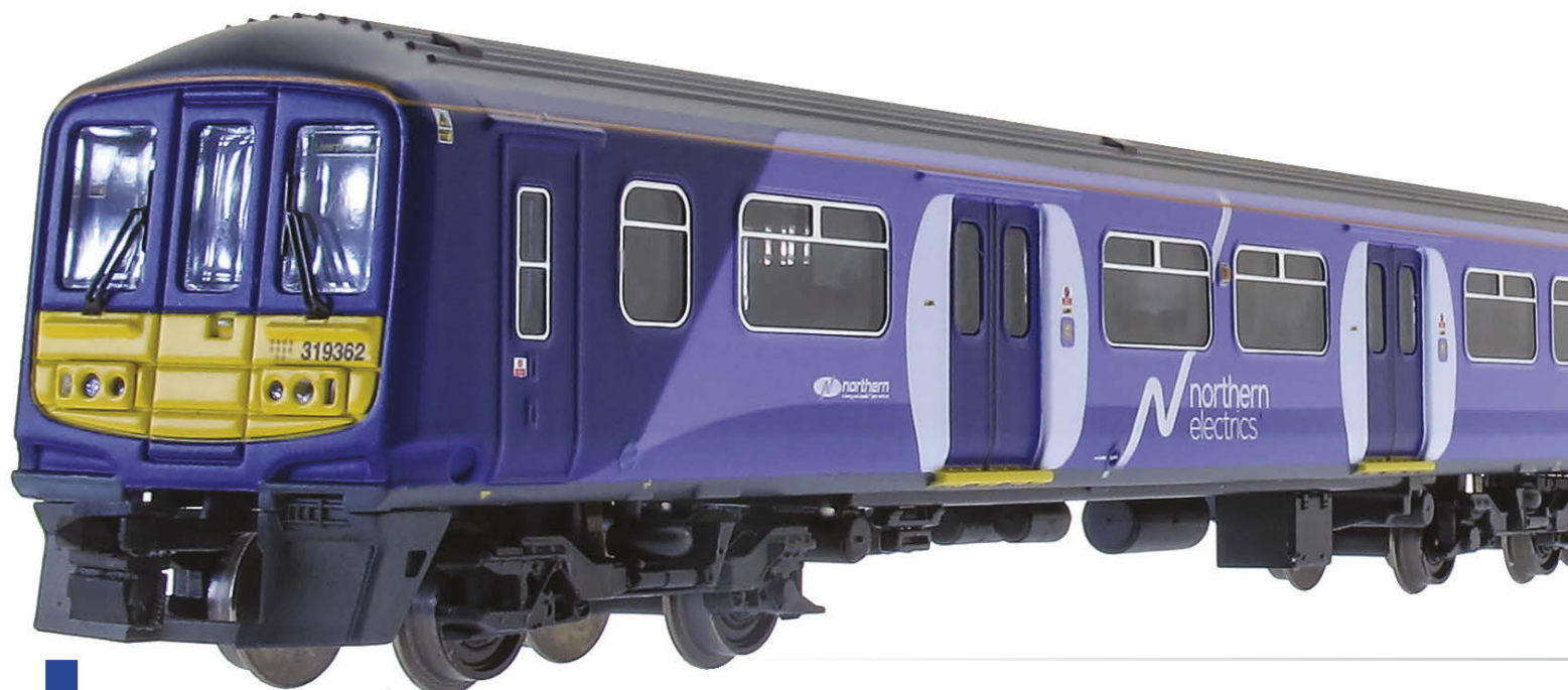
Farish's model captures the Mk. 3 style body profile of the unit well with complex shaping around the front face.
