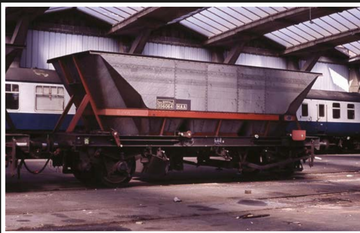
To prevent accidental door opening, safety catches were fitted, which had to engage before the wagon was loaded. If not, the wagons were permitted to run empty with a door open to a repair point and HAA No. 356064 had been stopped at Edge Hill for attention when recorded in May, 1990.
