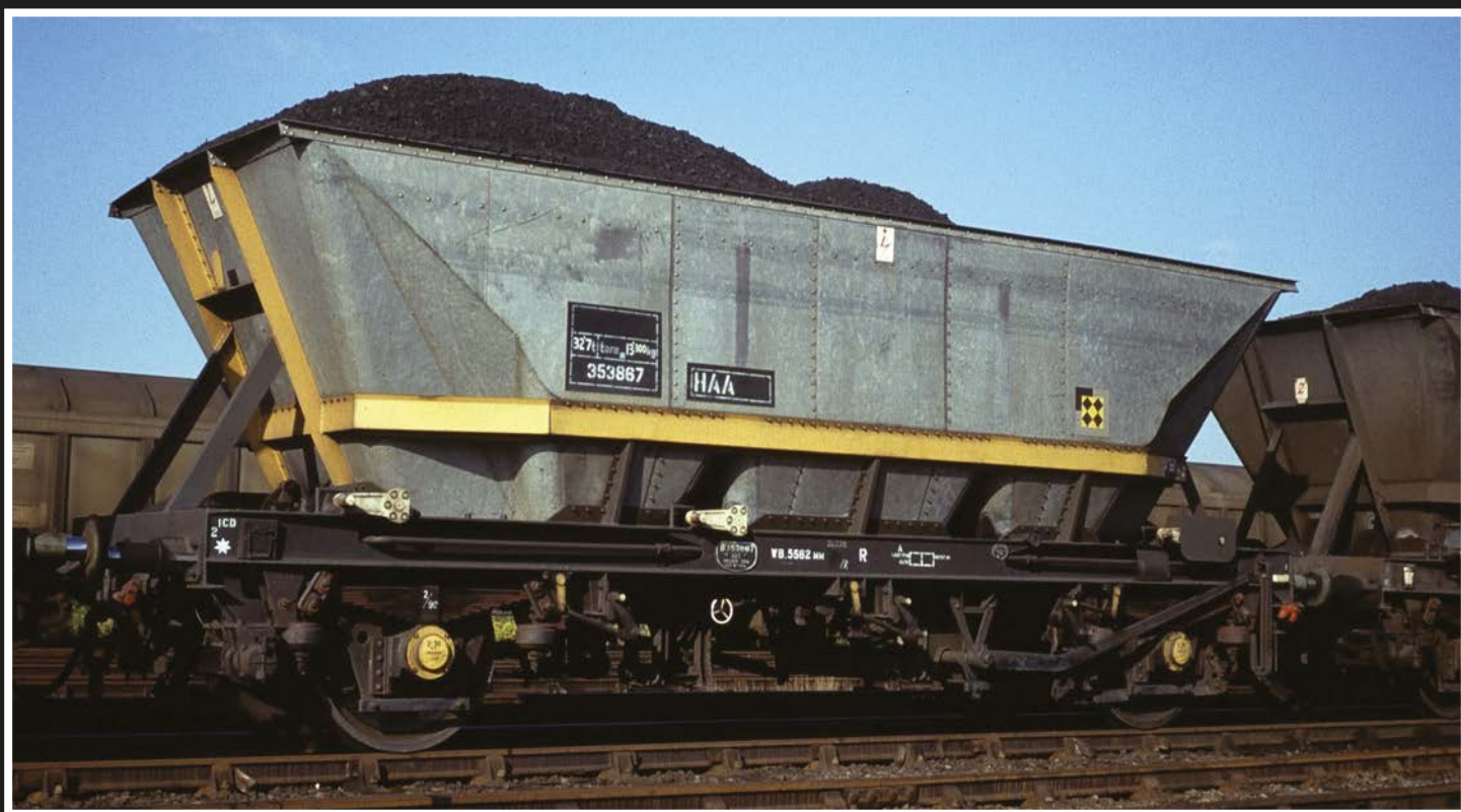
Fitted with an internal strengthening plate as evidenced by the additional row of rivets along the side, HAA No. 353867 was well loaded with imported coal when photographed at Immingham Dock in July, 1991.
