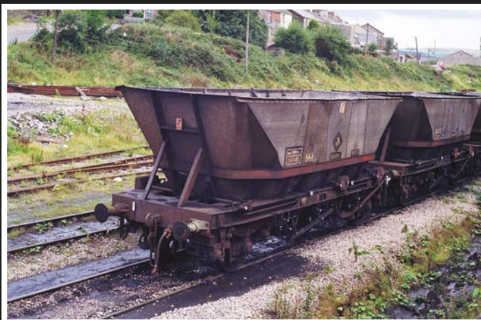
Still with its original body and traces of its HOP AB code, HAA No. 354546 had a flame red frame and Barry Depot plaque when recorded at Taff Merthyr Colliery in September, 1992.
