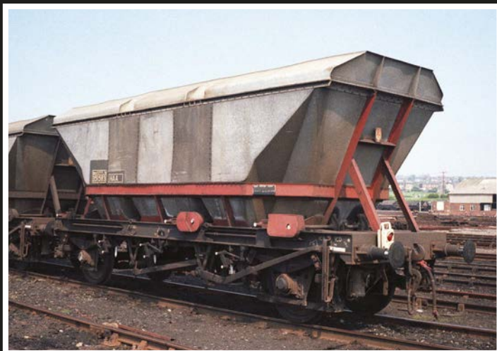
HAA No. 351583 had been fitted with a 'top-skip' when recorded at Healey Mills in May, 1989.
