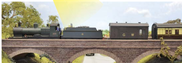
Also on 'Sanford and Banwell', this shot shows how the GWR locomotives carried spare lamps. Brackets were fixed to the side footplate for this purpose.
