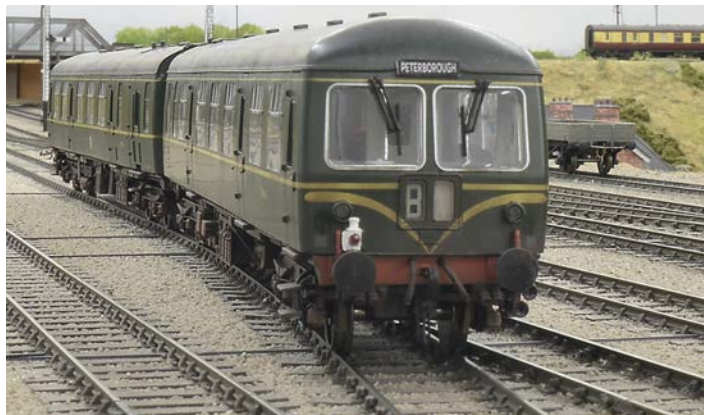
Finally, don't forget that in earlier BR DMU days, an oil-lit tail lamp had to be carried. Where locomotives or trains don't alter their workings, I'd advocate fixing lamps permanently in place to prevent their loss.
