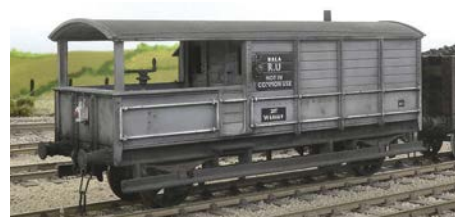
The same ModelU product, this time in 4mm:1ft scale, fixed to a Tom Foster-weathered RTR brake van. Note the side lamps as well – usually fixed (one each side) to denote an un-fitted train, where the locomotive crew could look out to ensure their train was complete. The side lamps displayed a white light forwards and a red one rearwards.
