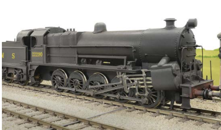
The top lamp here doesn't denote any status of train; it's 'Big Bertha's' headlamp, used when buffering up to a train before assisting it up the Lickey at night.
