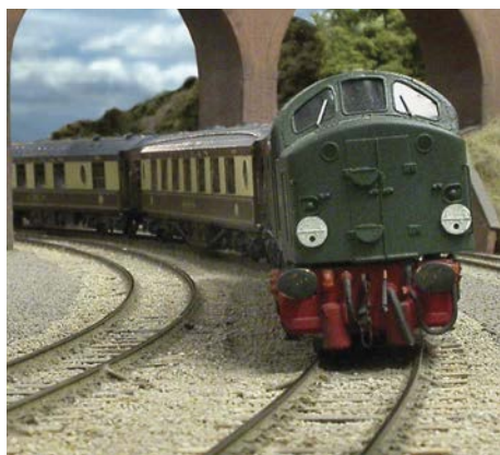
Some early BR diesels were equipped with discs as well as lamps for indicating their trains, as seen here as an EE Type 4 heads a Class A Pullman train on 'Stoke Summit'.
