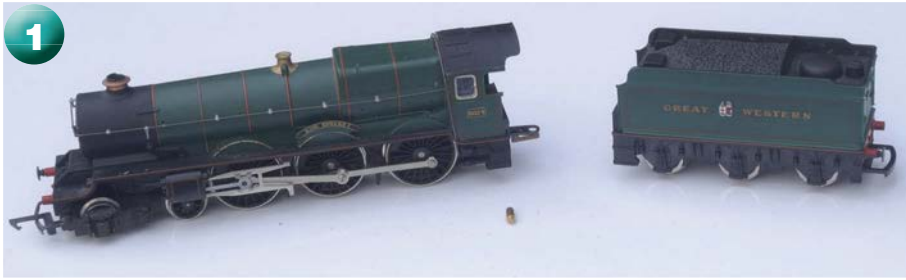
The locomotive as received. The broken pin for the loco-tender coupling was thankfully included and can be seen below the cab.
