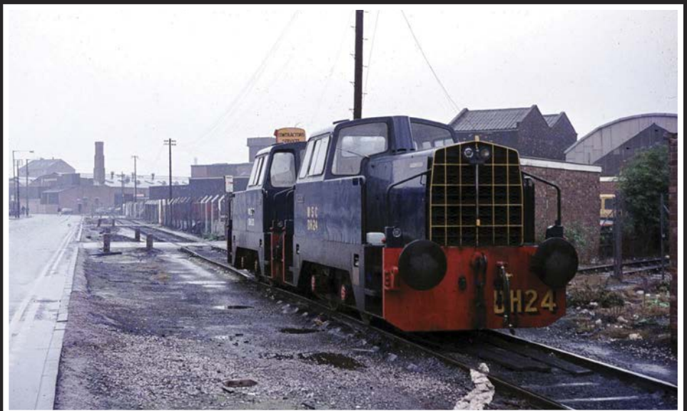
In November 1982, MSC Co. 4WDH Sentinel locomotives DH24 and DH23, works Nos. RR10227 and RR10226 respectively, both built in 1965, were recorded running light alongside Trafford Park Road on their way to collect empty coal hoppers from CPC. Hornby has a OO gauge model of these locomotives in its range, while several years ago, Hattons produced a OO gauge model of the Barclay saddle-tank in CPC livery.
