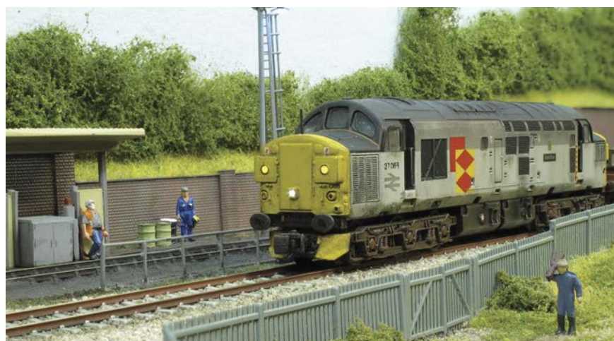
A benefit of DCC is that locomotive lighting can be operated separately to motor control, enabling more realism when it comes to idling locomotives.
