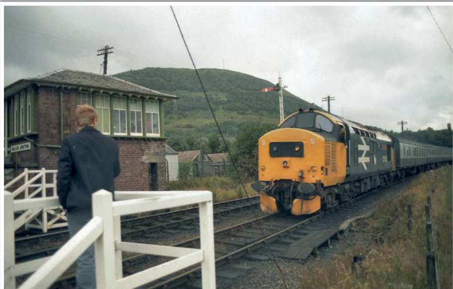
On 13th August 1987 the signalman at Mallaig Junction is about to hand over the single line token to the driver of a Mallaig bound train hauled by 37425 as it leaves Fort William. IAN HARRISON
