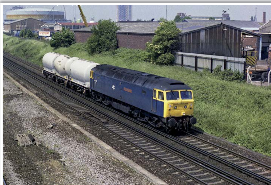
On Thursday 19th June 1986, 47409 'David Lloyd George' is approaching Millbrook, Southampton with a light load of three very clean Blue Circle PCA cement wagons on an unknown working which may be from Hamworthy. It consists of a pair of Metalair wagons sandwiching a depressed centre presflo. 47409 was a Gateshead loco and was withdrawn later that year, the name plates only being carried for one year. KEITH MANTLE
