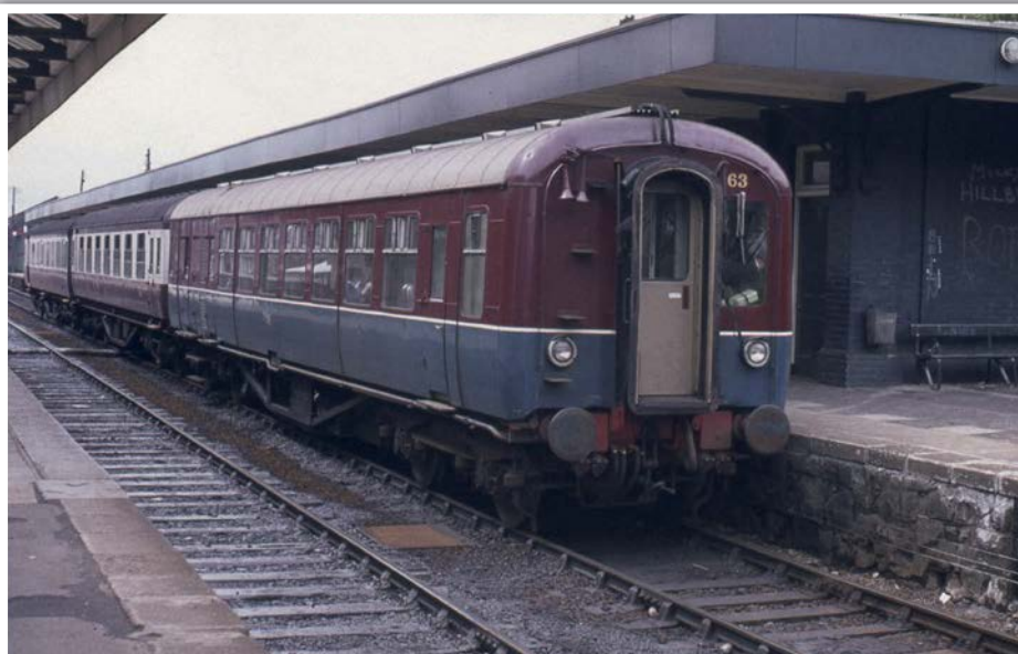
MPDs Nos. 63, 64 & 65 were built in 1961 and 1962 by the UTA with new bodysells and a 275hp Leyland engine on former coach underframes. A 260hp Rolls-Royce unit replaced the Leyland engines in 1968 and 1969. Nos. 63 and 65 received NIR's 'Enterprise' colour scheme in 1973, which No. 63 displays at Lisburn in 1974 with a Portadown to Belfast working. No. 63 was withdrawn in April 1981 and dumped in Crosshill Quarry in October 1983.
