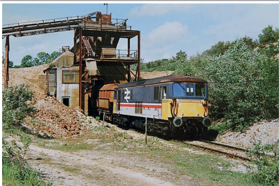
73128 pushes back the second half of its train of PHA side tippers under the loading apparatus at Lavant quarry. A combination of a full bunker and stockpiled material meant that a full rake of 10 wagons could be loaded in the space of about 40 minutes from arrival, with a bulldozer employed to fill the final 5 wagons with residual gravel stocked alongside the bunker. Wednesday 16th May 1990
