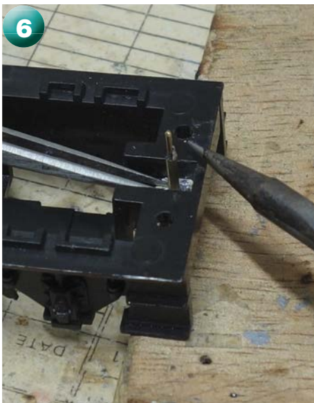
With the pin supported beneath, the washer/tube assembly was pressed down firmly and the loaded soldering iron applied at the top. Once the solder flashed over, capillary action took the solder sufficiently down the tube for a good joint, while keeping the heat away from lower down where the washer sits on the plastic – don't melt it! I then soldered the connecting wire to the top of this assembly. Once it had fully cooled, there was still some slight movement, so I ran a fillet of superglue round the shoulder of the pin from the underneath and this locked it in place.
