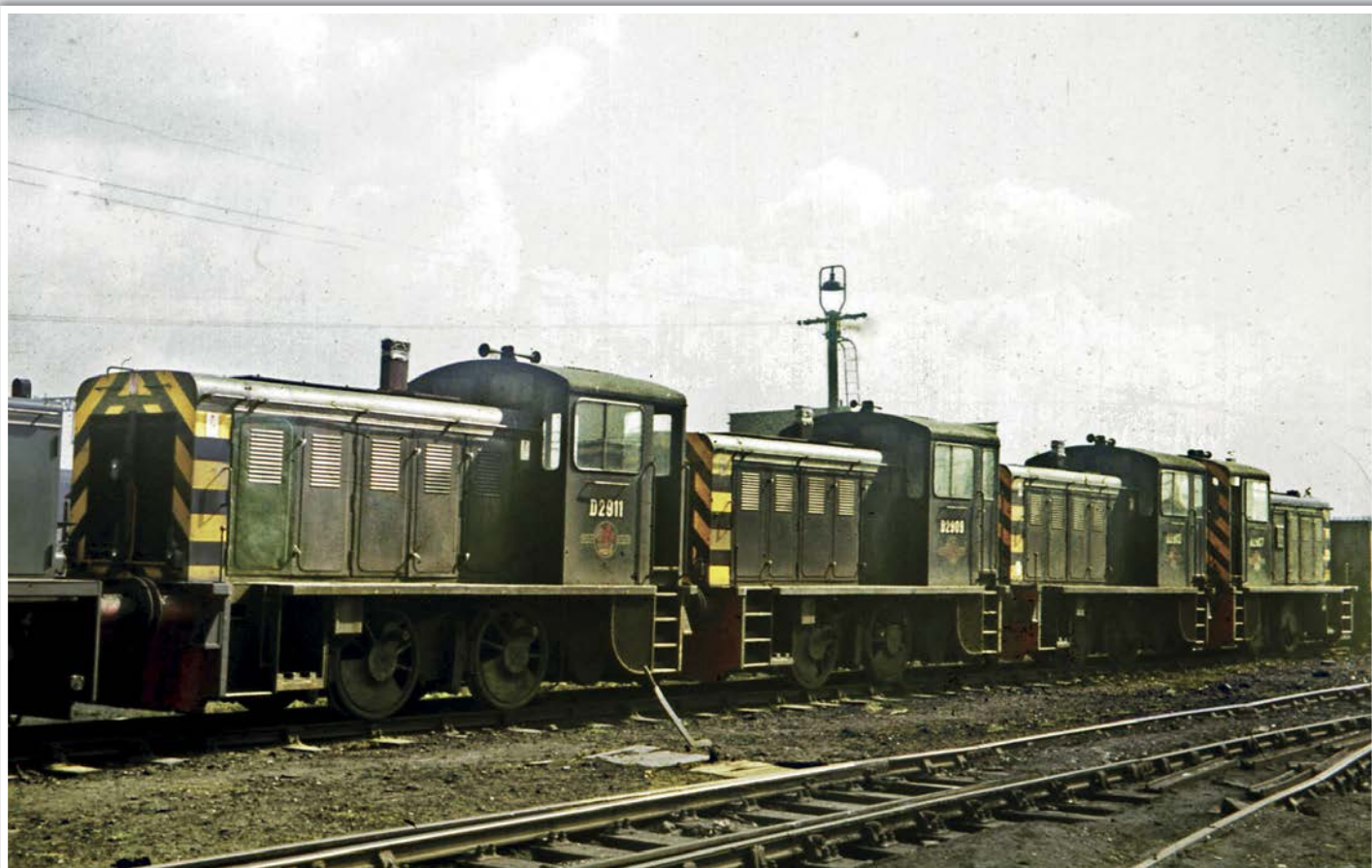
Crewe South was home to many diesel shunters including some of the types that had already been declared non-standard. A line up of D2911/09/13/07 on 31st March 1967 shows that indeed withdrawal looms as all have their connecting rods removed.
