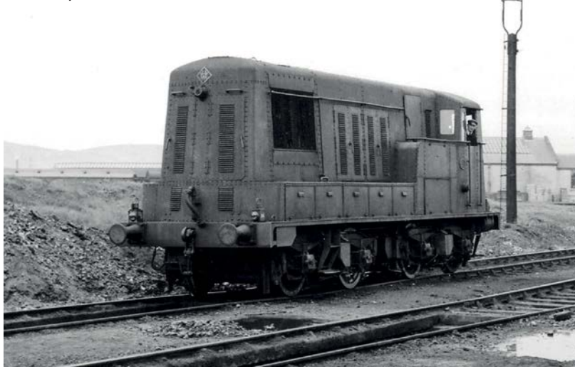
Diesel hydraulic No. 3 has disgraced itself at Lisburn in 1976 by derailling at the Belfast end of Lisburn's loop platform. Much of the NIR system was still manually signalled in the early 1970s, but centralised control and colour light signalling has now been extended to cover virtually all the system.
