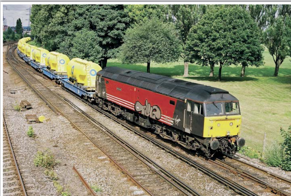
The only time I ever captured on film the infrequent and short lived 6077 Westbury to Millbrook bi-modal cement working was in the summer of 2003. A tatty looking 47843 is seen at journey's end with this service, entering Millbrook FLT, where the cement tankers would be off loaded using the terminal cranes for onward distribution around the south coast, primarily for concrete batching plants. However, the rail traffic did not last long. The specialist flat wagons went into store initially but then were exported to the continent where bi-modal workings such as this are far more common. JOHN DEDMAN
