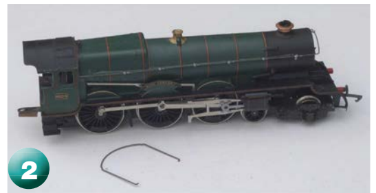
As well as the loose and distorted cab handrail, note the broken front handrail knob and the missing front buffer on the far side, with one also missing from the tender. Also missing this side is the cab glazing. It's possible that the locomotive suffered a hard impact or was dropped at some point.
