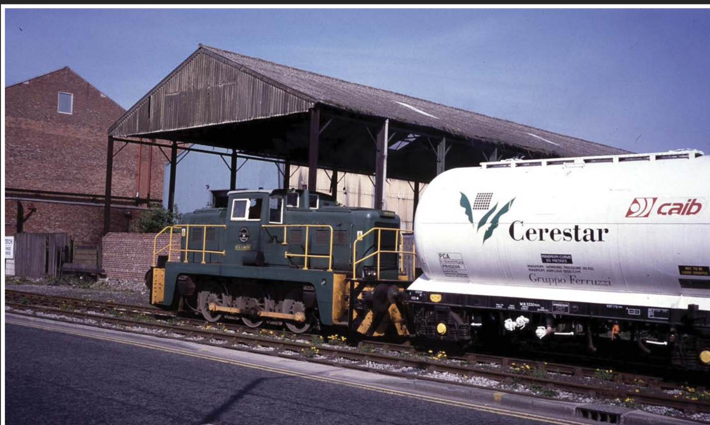
The Trafford Park Co. ' Janus ', works No. YE2878, shunts a Cerestar bulk starch wagon at the industrial estate in April 1994. Built by the Yorkshire Engine Co. in 1963, this locomotive had gained the name R.A. Lawday when with ICI at Runcorn and would retain it during its time in Trafford Park. Oxford Rail produces a ' Janus ' model in OO gauge.
