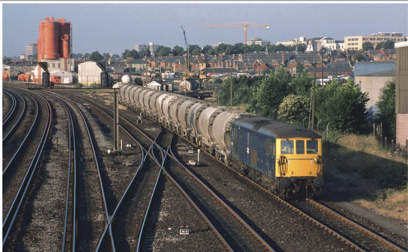
73108 is at Southampton Up Yard shunting cement wagons to form 6Y80 09:46 to Halling on 30th June 1984. These wagons are French built STS PCA wagons on hire to Rugby Cement. Accurascale produce a good quality model of these wagons in OO gauge. JOHN DEDMAN
