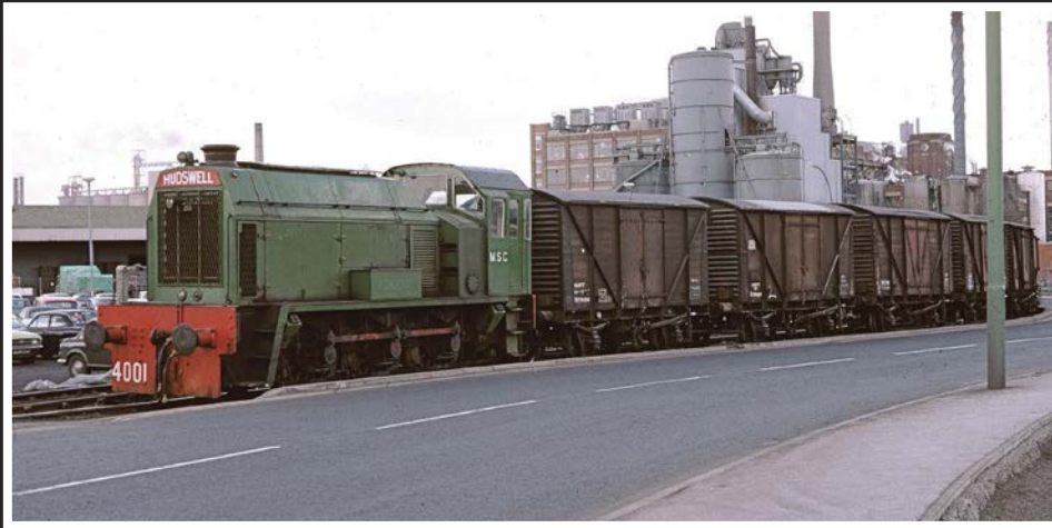
The MSC's Hudswell Clarke diesels also appeared on the CPC job, and No. 4001, a 430 bhp 0-6-0DE works No. HC D1075, built in 1959, pulls away from the CPC works with a rake of BR 12T 'Vanfits' in April 1977. On this occasion, all of the vans were loaded with bagged starch for the Wiggins Teap Pulp & Paper Co. at Corpach, near Fort William.
