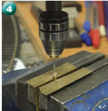
I drilled a 0.8mm hole in the centre of the pin, into which was soldered a length of 0.8mm brass rod. This solid joint gives something to attach to on the top, inside the tender front, and should also guarantee the current path to the motor.
