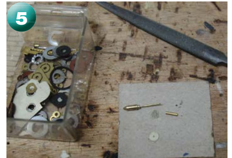
For the fixing arrangement, I used a length of brass tube (0.8mm inside diameter) and a flat washer from my 'washers' tray, where I keep all sizes and odds and ends of washers from kits – never throw anything away. I filed the washer to more of a square shape to fit the recess around the hole in the tender front, then soldered the tube to the washer, checking and adjusting until the tube was as good to perpendicular as I could get. It's ready for reassembly.
