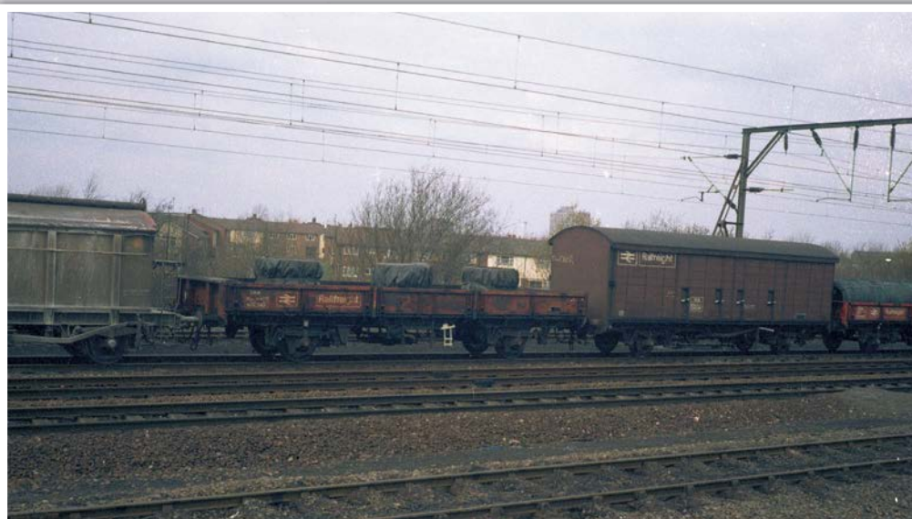
Most of the tinplate railed to Westhoughton was carried in modified BR Plate wagons recoded from SPA to SHA, such as No. 460842 seen at Crewe Gresty Lane when en route from Trostre in April 1986.
