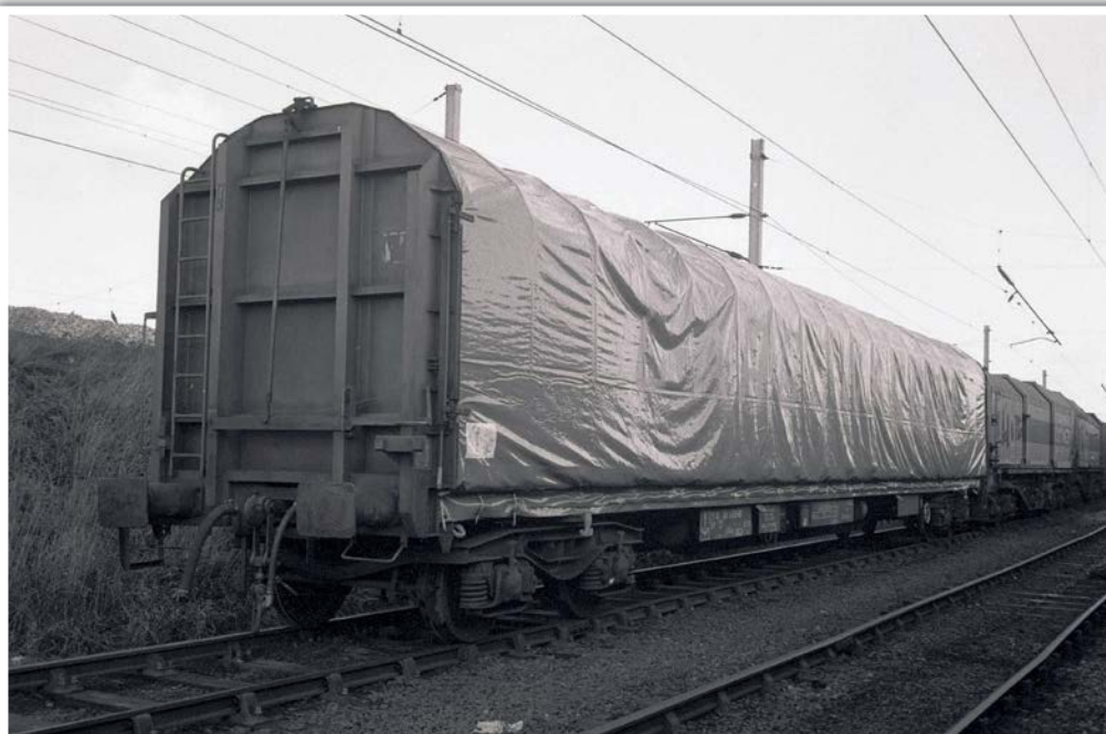
BR long-wheelbase air-braked were also occasionally used for the tinplate traffic from South Wales as were a small number of bogie Transferry curtain-hooded wagons. These included IPB No. 33 87 4746 039-6 which was recorded waiting to leave Warrington Walton Old Junction yard for Westhoughton on 12th December 1988. Beyond the IPB can be seen two VTG Telescopic hooded wagons which were also briefly used for the tinplate working.
