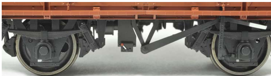
Clasp brakes are captured well on both variants. Visible in this photograph is the detailed FAT 19 suspension of the VEA, while door slides even have raised ribs, just like the prototypes.
