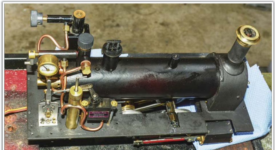
With the body removed, I fitted a servo to the reverser.
