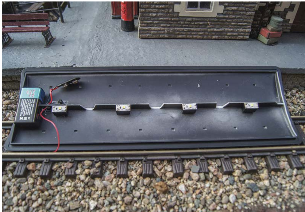
LED lights are glued to Lego blocks fitted under the roof.
