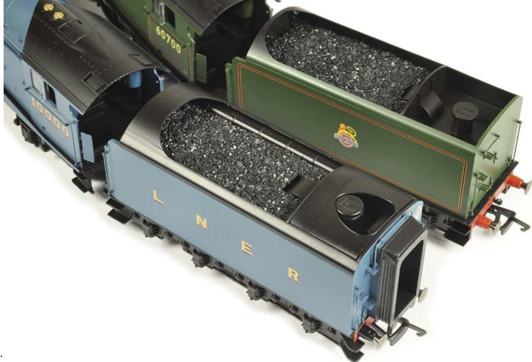
Both tenders are accurate representations of the 1928 corridor type (10000) and the 1937 streamlined non-corridor sort (60700).
