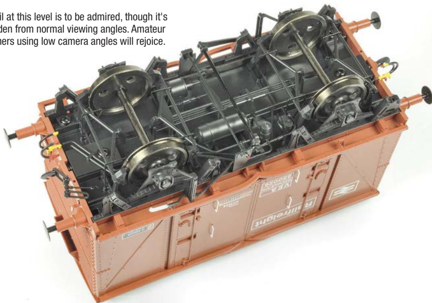
Clasp brakes are captured well on both variants. Visible in this photograph is the detailed FAT 19 suspension of the VEA, while door slides even have raised ribs, just like the prototypes.
