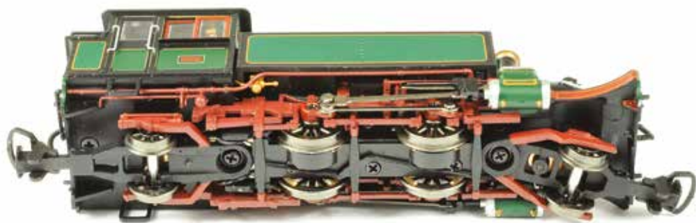
Both ponies incorporate light springing using phosphor-bronze strips to ensure good track holding, but the rear also picks up electricity; you can just see the wires on either side of the pivot.
