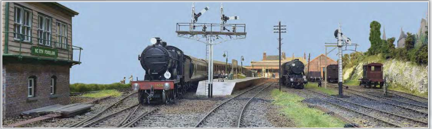
Boarding was essential to minimise the risk of railwaymen tripping over the rodding. 'North Foreland' in O gauge shows this feature.
