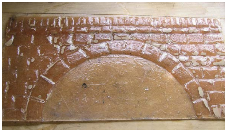
The appliqué panels for the abutments were made from glass fibre.
