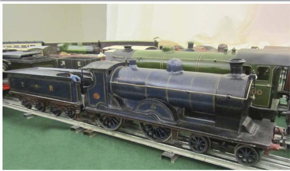
Stuart Rose's Bing Dunastair, converted to electric drive but otherwise original, on the Vintage Tinplate Group layout at the 2019 G1MRA AGM show last October. Note the loco footplate, curiously lower than the tender, which prevents the fallplate from lying flat.
