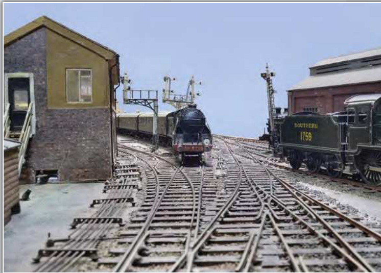
One of the oldest layouts still running is 'Metropolitan Junction' in EM. Here, not only is the point rodding visible, it actually operates the points. Levers are hidden behind signal box facades that operate the points.
