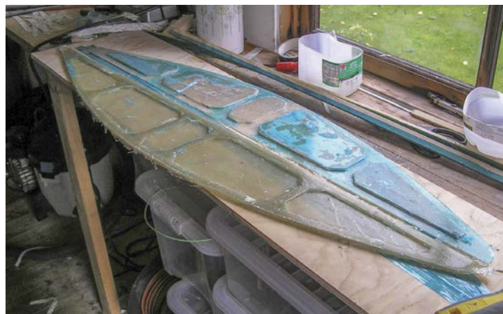
A bow string bridge laminate was also made from glass fibre.
