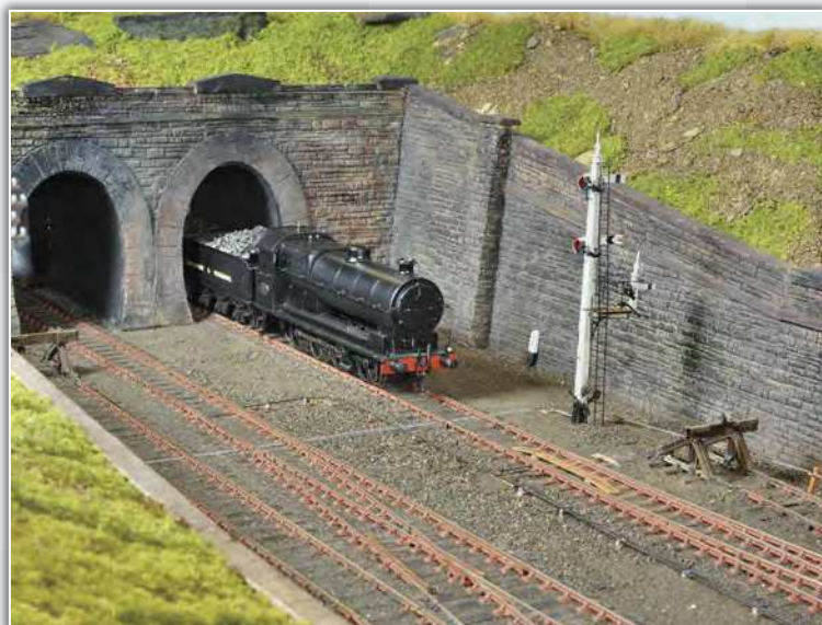
Facing points would require a locking bar, meaning two stretches of rodding to operate a point; as shown here on 'Calderwood' in OO gauge. The wooden covering is typical.
