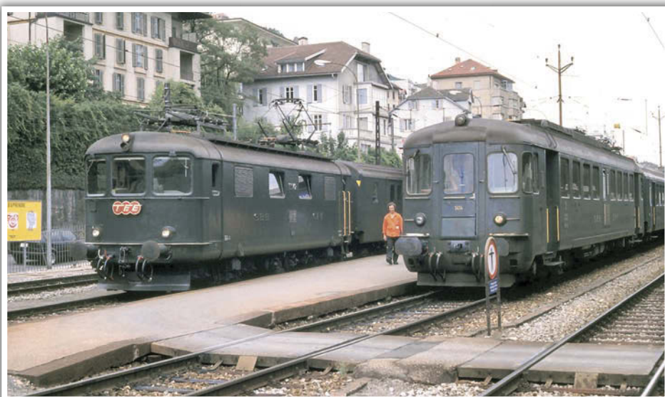
The second batch of Re4/4s, that later became reclassified Re4/4I to differentiate them from later locomotives, were built with full width cabs. Some were used on Trans Europ Express (TEE) services, which No. 10042 was certainly not working when seen on a local train at Neuchatel in the 1980s. DAVID FORD
