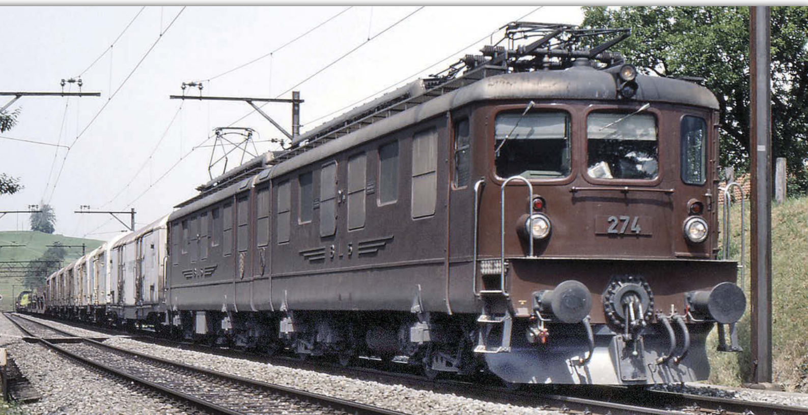
In 1959, the BLS received four giant double Bo-Bo locomotives for the Lötschberg line's heaviest freight trains. These were basically each a pair of back-to-back Ae4/4s with the wheel arrangement Bo-Bo+Bo-Bo. No. 274 is seen near Kumm, north of Spiez, on 11th July 1984. PETER ALDER
