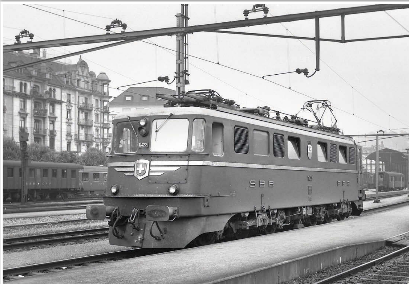
The new 'grand dame' of SBB in the 1950s was the Class Ae6/6 Co-Co design which was used on heavy international passenger services across the Alps. Dark green No. 11422, which carried the name Vaud and the town's crest, was being released from its train at Luzern on 27th August 1959. COLIN BOOCOCK
