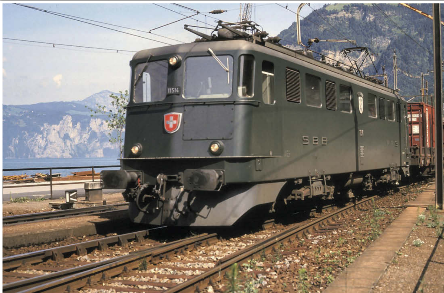
Ae6/6 11424 is seen with northbound freight at Flüelen on the 17th August 1988. Note that the aluminium trim has been removed due to corrosion. DAVID FORD
