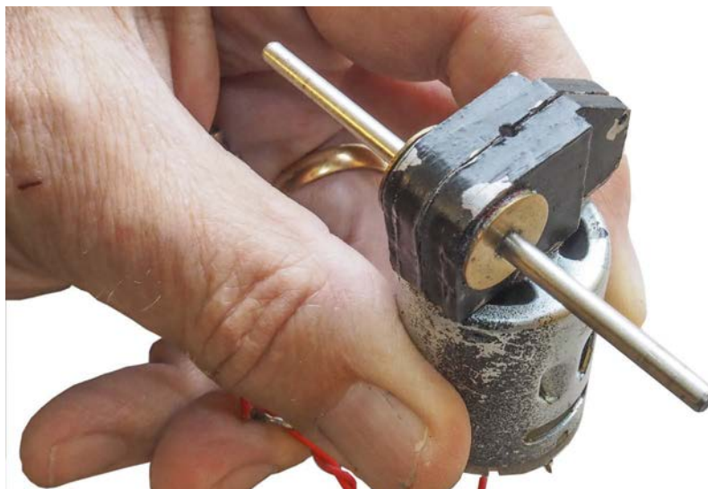
The plastic gear pressed onto a spline and was encased in a white metal gearbox casing, which was then glued to the motor. This was the weak spot of this old design.
