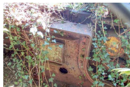
The south end of the up-turned wagon. The yellow roller bearing axlebox cover is correct for B900110.
