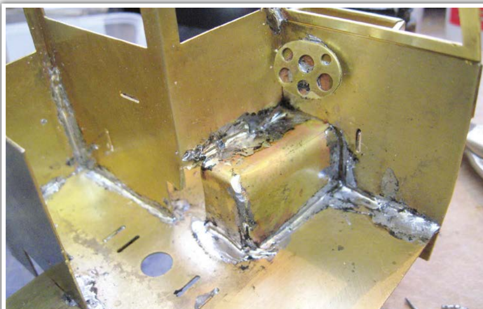
A view showing the inside of the cab and the additional "engine cover" to provide room for the third 185650 li-ion battery. My soldering was not quite so neat in this confined space! However, a bit of filing soon tidied this up.
