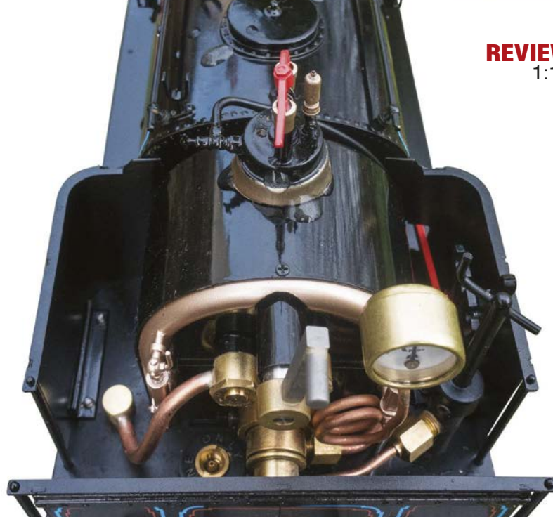
The open cab makes it easy to see, and operate the controls, but will make fitting radio control a challenge.
