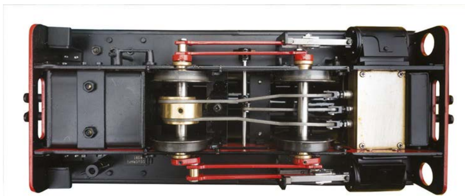
Looking underneath at the Simulated Stephenson's link valve gear.
