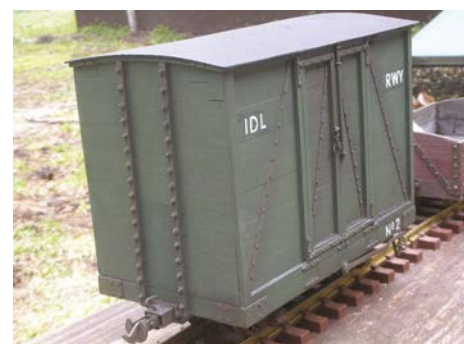
Lots of nut-bolt-washer details adorn the ends. These are castings, whereas the simpler bolt heads on the side are slices of plastic strip fixed with MEK.
