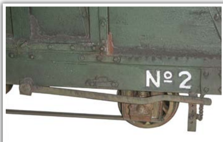
The brake lever details were cut from 16g steel. The chain is from an old piece of jewellery.
