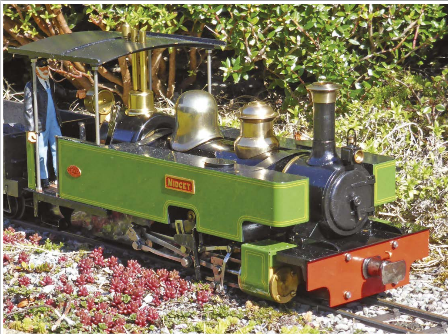
Meths-fired "Midget" built by me.
