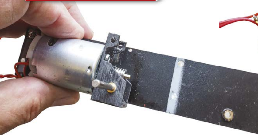
The new gearbox almost fitted and was carefully adjusted with new holes for the torque rod drilled into the chassis.
