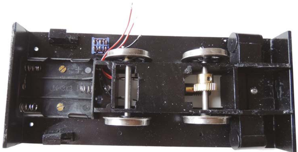
The chassis with wheels, gears, switch and battery holder fitted.
