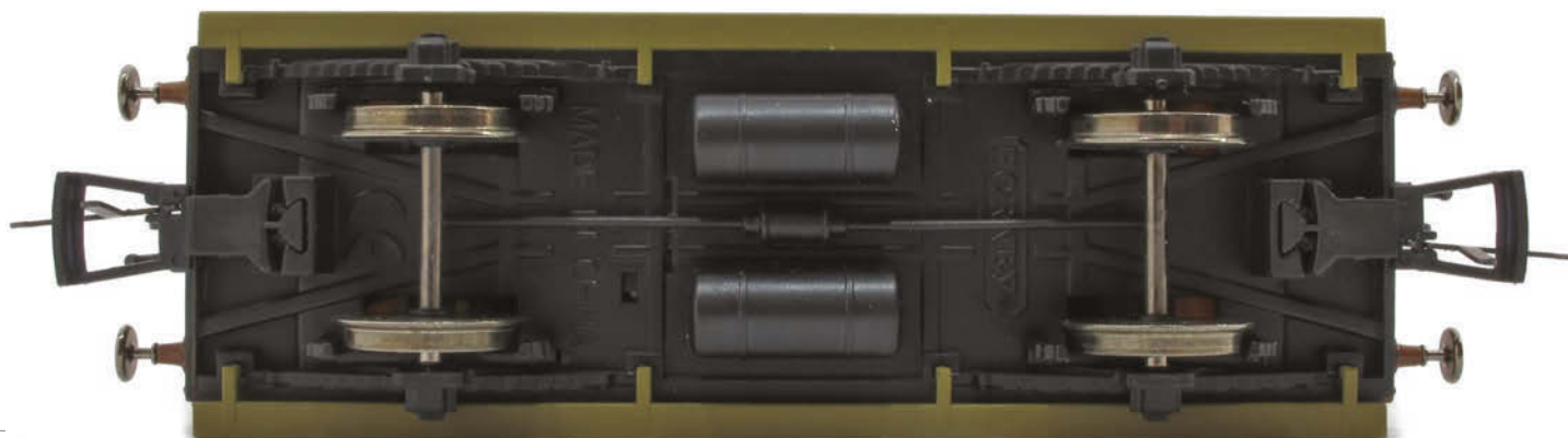
Underneath, we have gas tanks to match the gas light tops on the roof.
