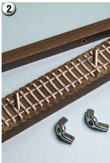
Drop the sleeper bases into the assembly jig and tighten the locking bar. Avoid over tightening as this may distort the sleepers.
