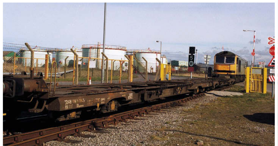
A wide range of container wagons appeared in EWS intermodal services with the rarest being Unilog's fleet of Belgian registered IJA single flats. These included No. 33 88 4910 107-0, which was photographed on 18 August 1998 when being shunted by Class 09 No. 09021 shortly after it had arrived at Hams Hall from Muizen in the consist of the 08.35 from Wembley.
