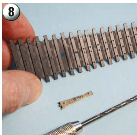
Carefully remove the cast frog fitted to the Sleeper base. Drill a 2.5mm hole between the sleepers, which will be hidden by the frog. Replace the push-fit frog after you have drilled and deburred the hole.
