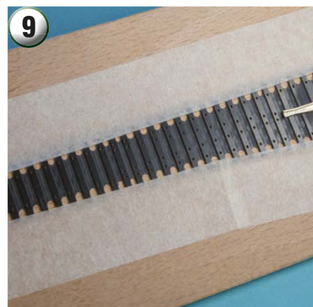
Tape the sleeper base to a piece of scrap plywood. Ideally, use a piece that is flat and not warped. This provides a stable temporary work surface during assembly.
