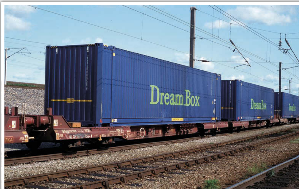
During 1999/2000 Thrall's York workshop built a fleet of 150 low-deck FKA twin flats for EWS. These were capable of accommodating high-cube boxes within the standard British W6 loading gauge and could subsequently be seen on almost all EWS intermodal services. FKA No. 81 70 4908 056-4 was marshalled in the consist of 4Z59, the 11:35 Warrington Dallam to Glasgow Shieldhall (Deanside Transit) when photographed at Warrington Arpley on 3rd June 2001. Only running for a couple of years the 'Dream Box' train conveyed Safeway products.
