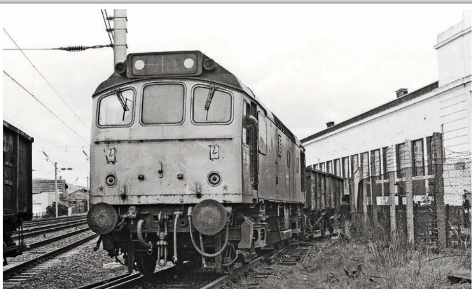
April 1981: Class 25 No. 25190 delivers a couple of 16-ton mineral wagons to Vauxhall Motors' Luton plant, which was sited just to the south of the town. The wagons were apparently used for out-going scrap metal/off-cuts rather than for the delivery of coal. Note that the 'Bed-Pan' electrification catenary is already in place on the main lines.
