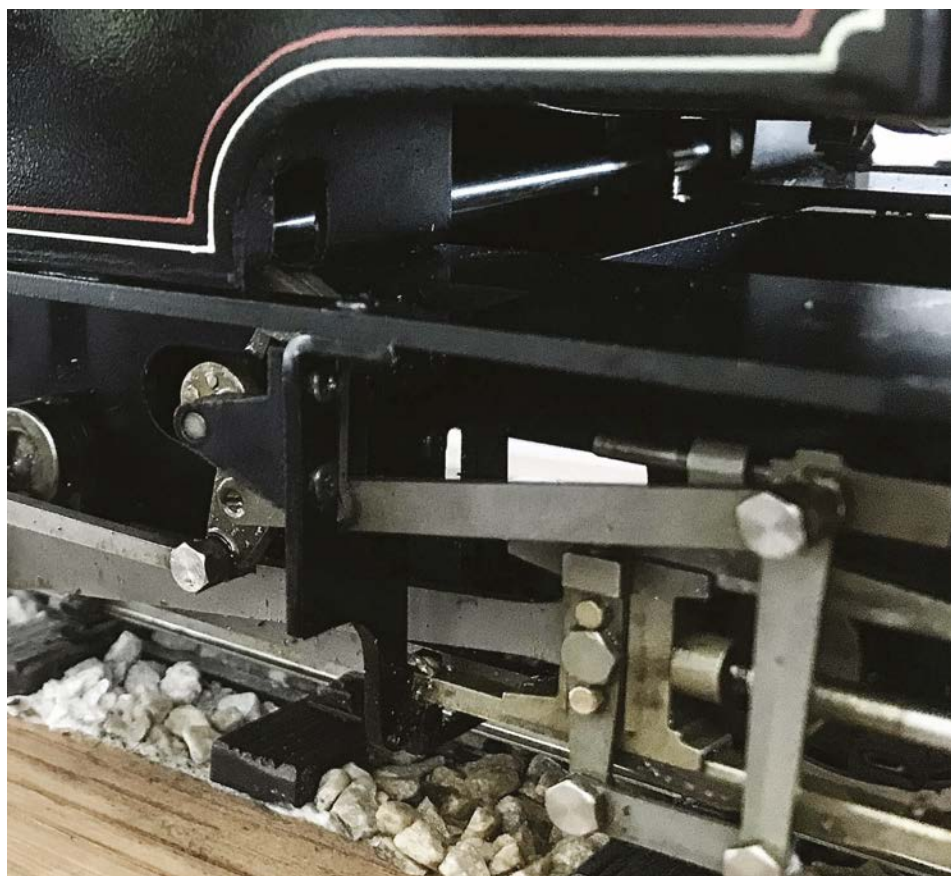
If you look closely, you will just see the filed slot in the tank round down (taken from around three inches away).
