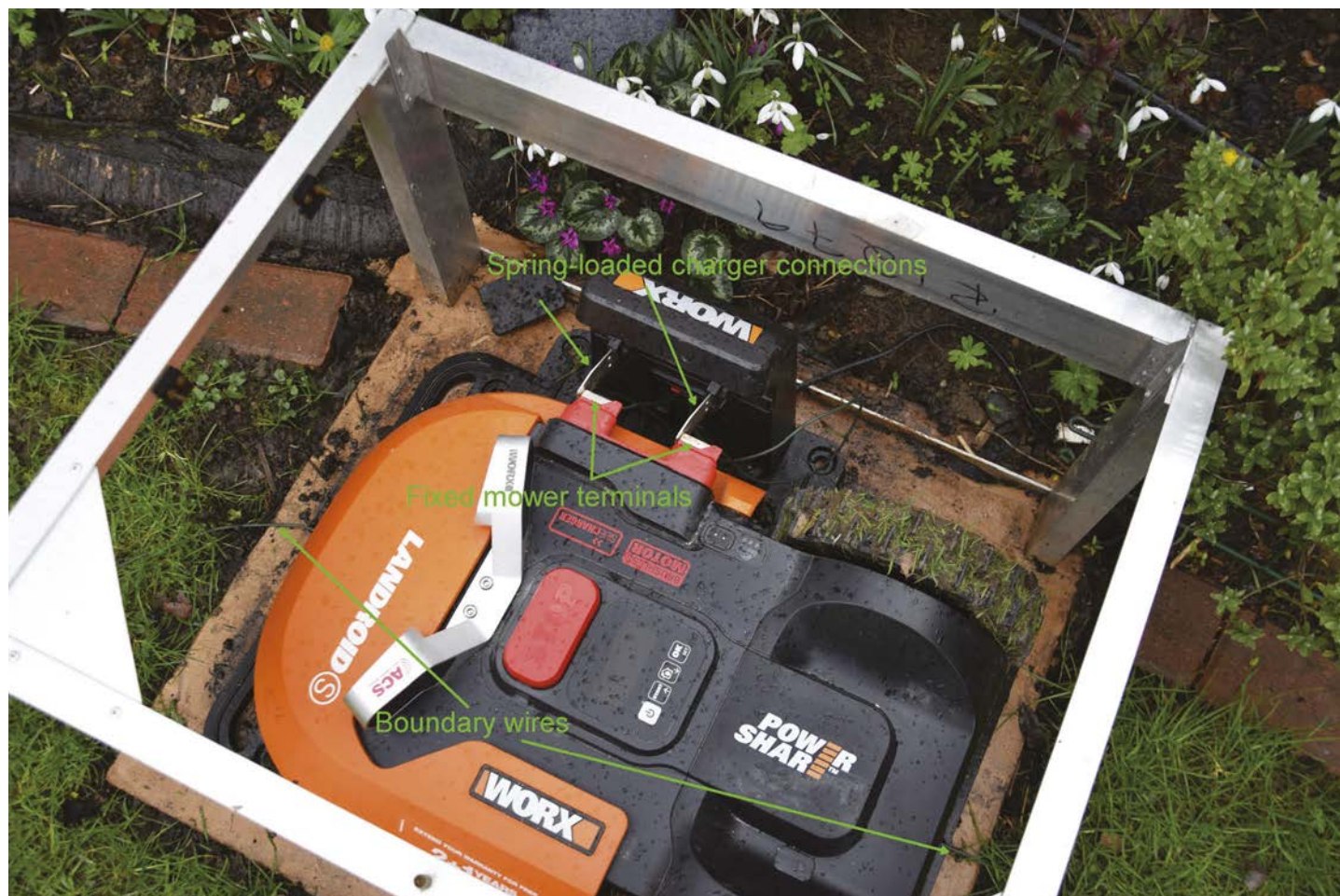
The basic frame of the building showing the way it accommodates the mower and charger.
