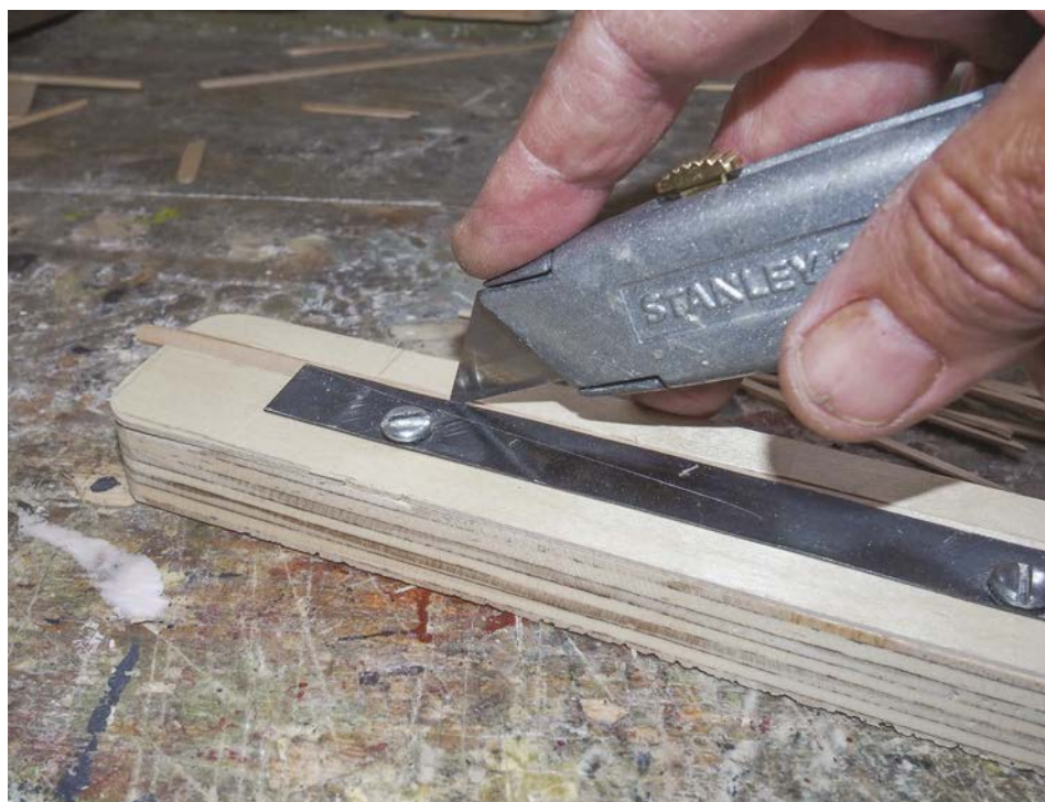
To get more realistic detail for the seat slats, it was necessary to cut coffee stirrers in half. The jig was made to guide the Stanley knife blade.
