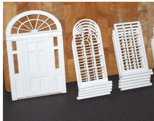
The front door and the window frames stacked ready for use. This is where a 3D printer really becomes useful – draw one arched window or chimney, and print as many identical copies as required. Then, if one accidentally gets damaged, simply print another.
