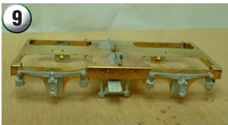
The assembled bogies with cast white-metal axle boxes and bolsters fitted using superglue. The axle boxes fit snugly over the waisted brass pinpoint bearings. Solder flux has been removed with household cleaner and an old toothbrush.
