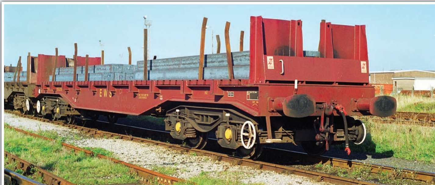
Recently repainted into EWS livery, BBA 910298 was photographed at Workington Yard when carrying a load of steel blooms from Lackenby in September, 1997. Note the replacement spoked handbrake wheel fitted to one bogie.
