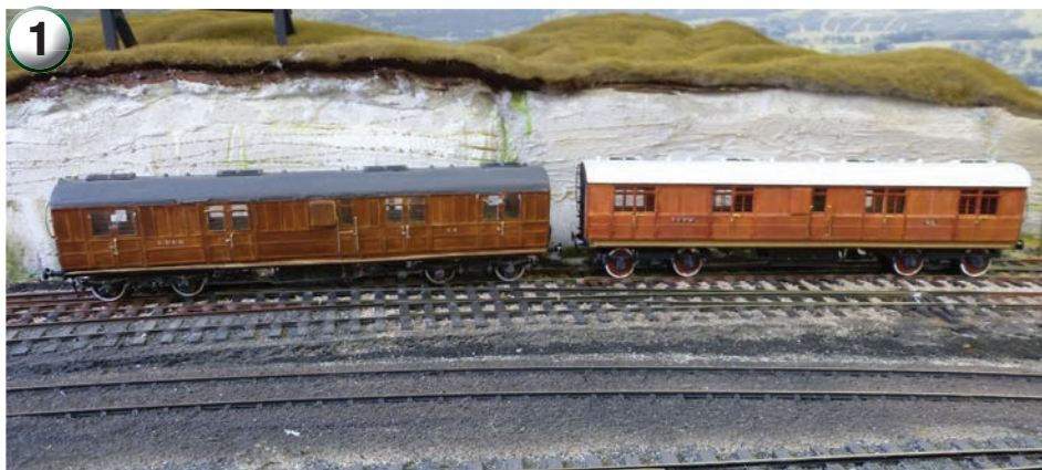
My scratch-built effort (left) with the Isinglass kit finished in pristine condition (right) to highlight the contrast. The 40-year-old scratch-built model features Perspex sides and Plastikard ends with detailing from 5 thou Microstrip. The teak finish represents an older "in service" vehicle. McGowan cast white metal bogies add weight low down to aid stability. Pinpoint bearings and EM gauge wheels make this a free running bogie van.
