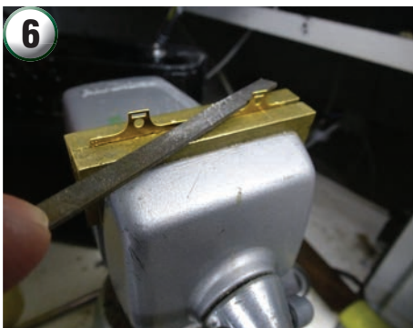
The Roxey Models' etched brass bogies need the usual cusp to be removed after separating from the main fret. A modeller's vice helps to steady and protect the delicate sides. Only a few strokes of the file are necessary.
