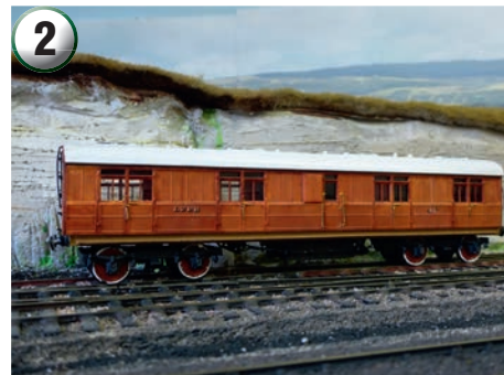
The Isinglass model shows off the mild wood grain texture inherent in 3D printing, highlighted by subtle graining of the Precision paint. The grain above the waist is vertical and below is horizontal. The underframe has etched brass queen posts and cast vacuum brake and battery boxes.
