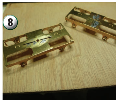
The bogies assembled with solder fillets to beef them up. The design incorporates a simple but effective three-point compensation using wire soldered to the tops at right angles to each other on each bogie.
