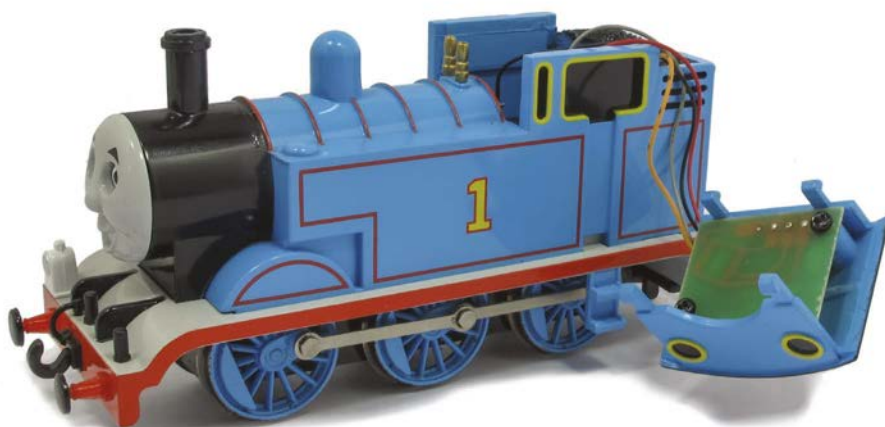
The cab roof unclips to give access to the circuit board. Undo the screws in the corners to reveal the Next 18 DCC socket.
