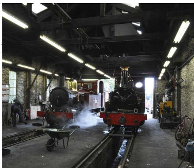
Tours of the Douglas shed are a step back in time. This is a working steam shed, which has the potential to carry out all the work needed to keep a fleet of locomotives in operation, although many jobs are now contracted out. Here we see 2-4-0T Hutchinson on the left and the unique 0-6-0T Caledonia on the right in the running shed.
