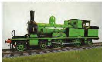
1:32 SCALE ADAMS RADIAL TANK 4-4-2T The model is 1:32 scale for 45mm gauge track, gas-fired with a single
