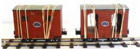
The coach roofs being held in place with elastic bands, which I cut off after the roof was set as there was less risk of damage to the body.
