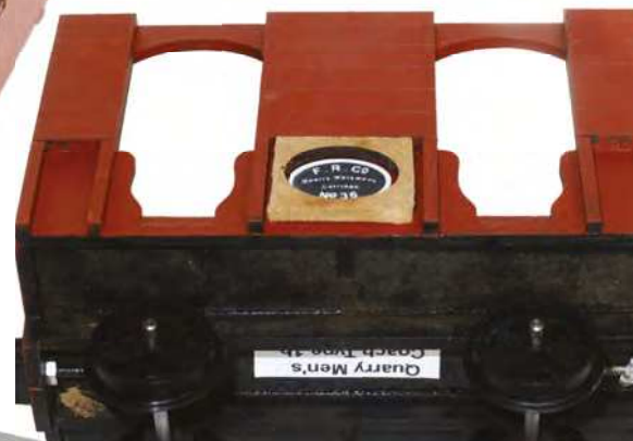
I cut out around the fret that the maker's plates were located in and used this as a useful template to help to get them mounted neatly on the carriage sides.
