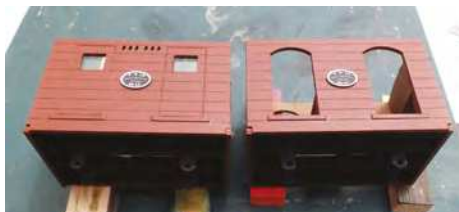
Wooden supports allow me to mount the maker's plate to one side, then flip the bodies over to repeat the process without disturbing the plates on the lower sides of the models.
