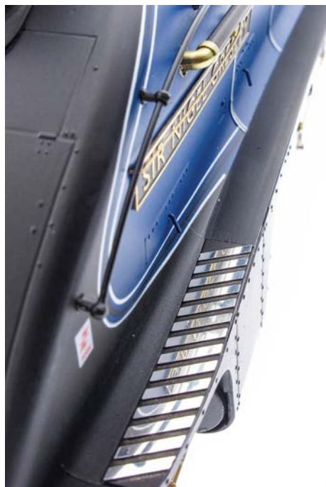
This model unusually features polished-steel treadplates over the cylinder area whilst the complex-shaped lining changes can be appreciated from this angle.
