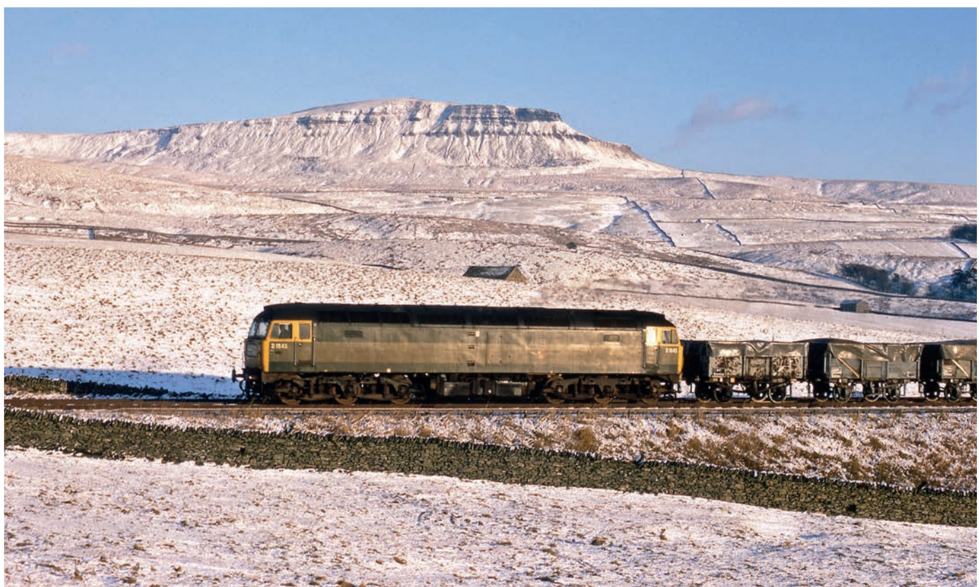
Green liveried No. D1545 had recently been reallocated from the Crewe Division of the London Midland Region to Tinsley. The Eastern Region depot has already painted its trade mark steam era shed code '41A' on the cab side. The Brush Type 4 is seen climbing past Horton-in-Ribblesdale with a freight that includes sheeted mineral wagons and is believed to be the Skipton to Carlisle pick up freight. 29th November 1969
