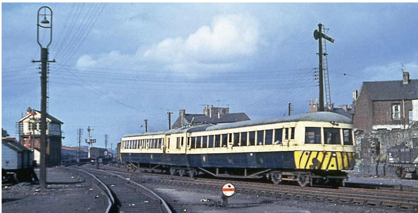
GNR(I) railcar D was photographed on the Warrenpoint line in Northern Ireland after being taken over by the Ulster Transport Authority and renumbered 101. This unit was withdrawn in 1963 after 27 years use. The power pod rides on three axles that are coupled by side rods, which can be seen clearly in this picture. Colour-Rail
