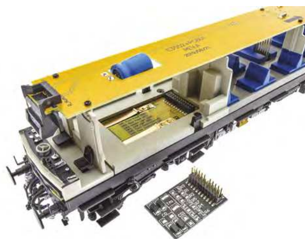
The PluX22 blanking plug and socket are to be found inside the guard's compartment.
