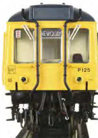
Close up of the 121 Driving cabs showing the cab end exhausts and the variations in buffers and headcode boxes over the three models - The green Class 117 (35-500) doesn't feature marker lights as was typical for its era.
