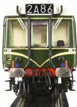
Close up of the 121 Driving cabs showing the cab end exhausts and the variations in buffers and headcode boxes over the three models - The green Class 117 (35-500) doesn't feature marker lights as was typical for its era.
