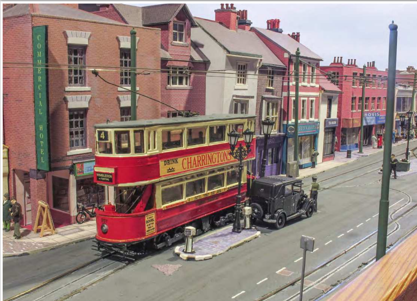
An E1 passes the Commercial Hotel. All of the trams have at least four tiny skids which improves electrical continuity. The overhead wire support poles were put in with a slant away from the road so the cross wire pulls them back to upright to provide stability to the pole wire.
