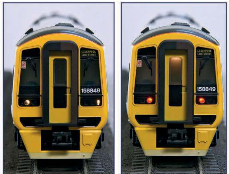
Front and rear lights are a given, but the Branchline model also features illuminated destination panels plus the option to illuminate the rear cab - ideal for the guard travelling in the rear of the train as they often do.
