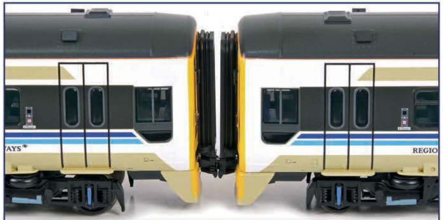
The BSI couplings fitted to the outer ends of each model not only look realistic, they're operational too allowing two units to be coupled together.
