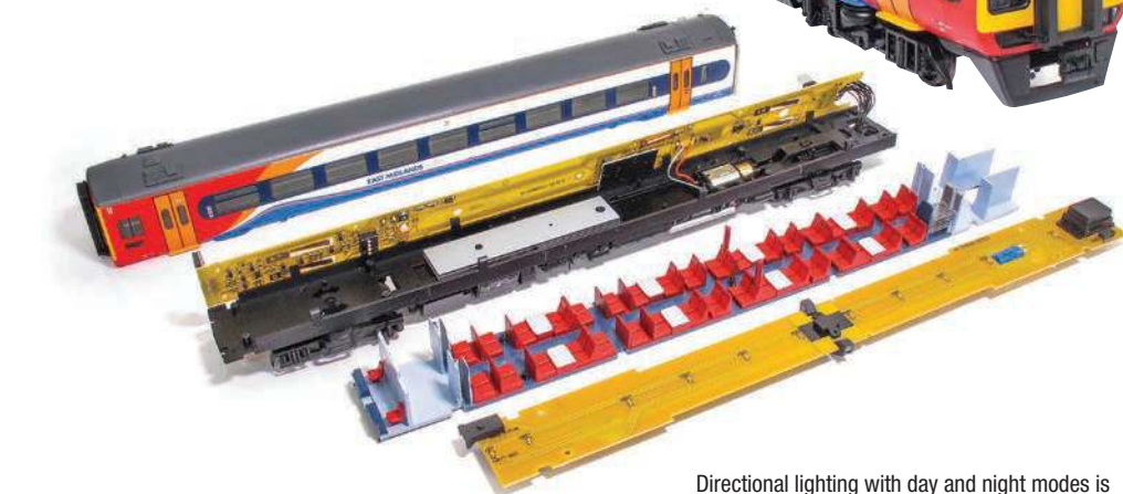
Disassembling the model highlights how unobtrusive the motor and drive mechanism is. Both vehicles are motorised.
