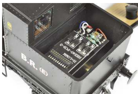
A decoder board housed in the spacious water tank and coal bunker is revealed by lifting the tank lid. Very neat.
