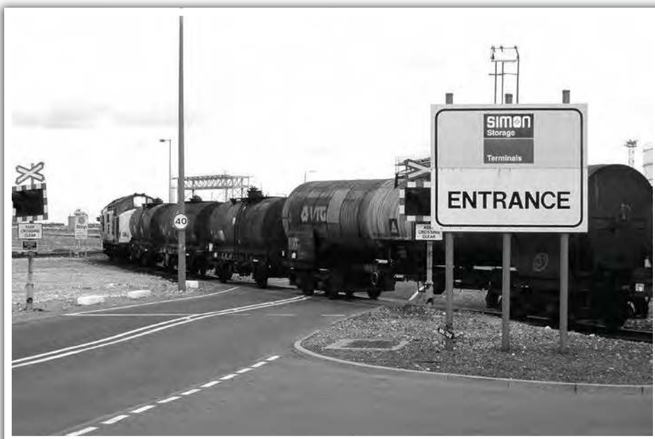
Thursday 8th April 1999: Working 6P60, the local Tees Yard tripping turn that served Haverton Hill, Port Clarence and Seal Sands, 37801 is seen at the furthest extremity of the Seal Sands branch shunting Dow Chemicals caustic soda traffic. This had been loaded at the Simon Storage facility and was destined for Dalry (Roche) in Ayrshire. The 45 ton (glw) tanks next to the loco were hired from CAIB, having previously worked from ICI at Runcorn. The larger bogie tank was one of two such vehicles hired in from VTG. IMAGE & CAPTION, TREVOR MANN.
