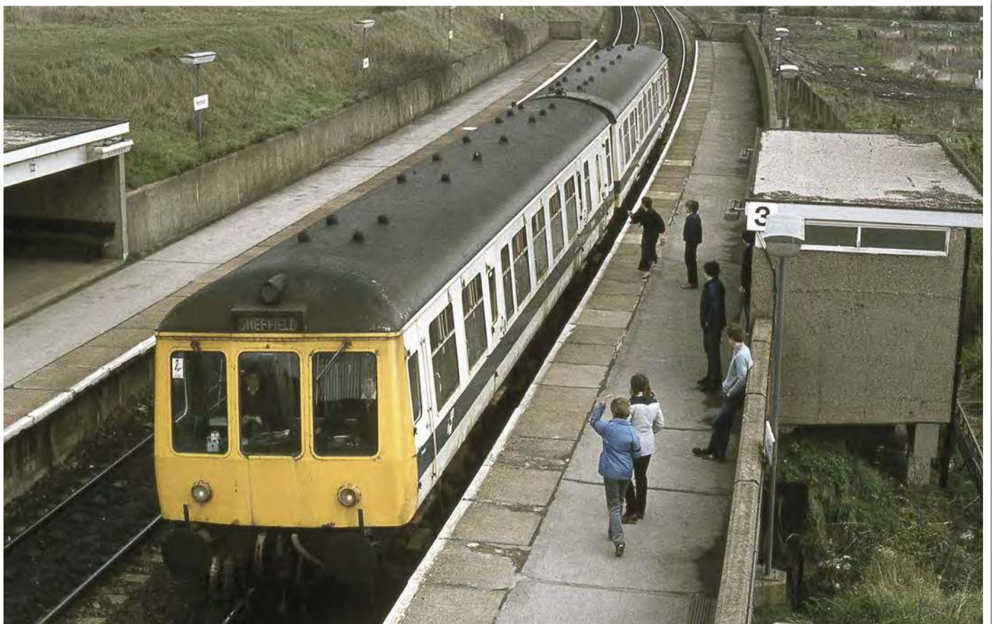
One of the Lincoln based Class 114 DMUs, formed of power car E50042 and driving trailer E56038, is seen calling at Retford Low Level on 23rd March 1981. The 49 units of this type were 64' 6" long compared to the normal 57' 6" of the visually similar Class 108s. DAVE HIGSON
