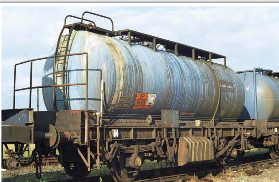
Between 1993 and 1996 sulphuric acid from Seal Sands to Dalry was carried by a pool of five two axle 32 tonne capacity tanks hired from EG Steele by Hays Chemicals. They had been converted from nitric acid tanks and TTA No. STL 51952 is pictured at Port Clarence in July 1995. At Dalry the sulphuric acid was used as a catalyst in the Reichstein Process of manufacturing vitamin C.
