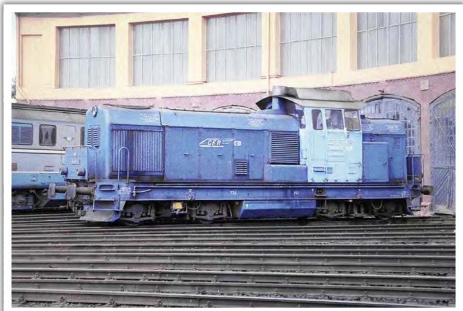
(ABOVE) On 3rd August 2003, Sulzer-engined B-B diesel hydraulic No 80-0278 stands outside Sibiu depot. Locomotives of this type were exported to other countries such as Bulgaria and Hungary, but with different power equipments.
