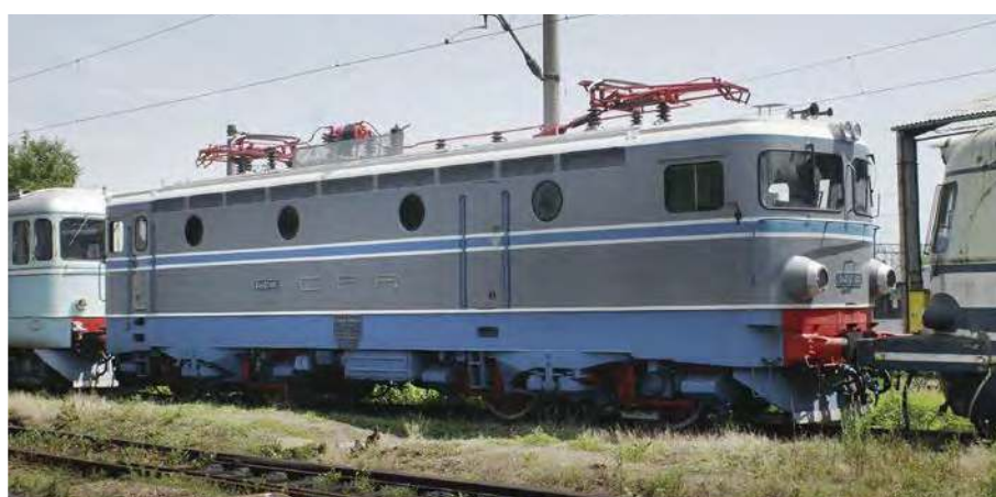
The first Bo-Bo electric locomotive to be delivered to CFR was this one, 040-EC-001, seen in its preserved state at Dej depot on 26th August 2015. It subsequently became 43 0001. The class was built in Yugoslavia by Rade Končar of Croatia and is used for secondary and main line passenger trains and freights across the country.
