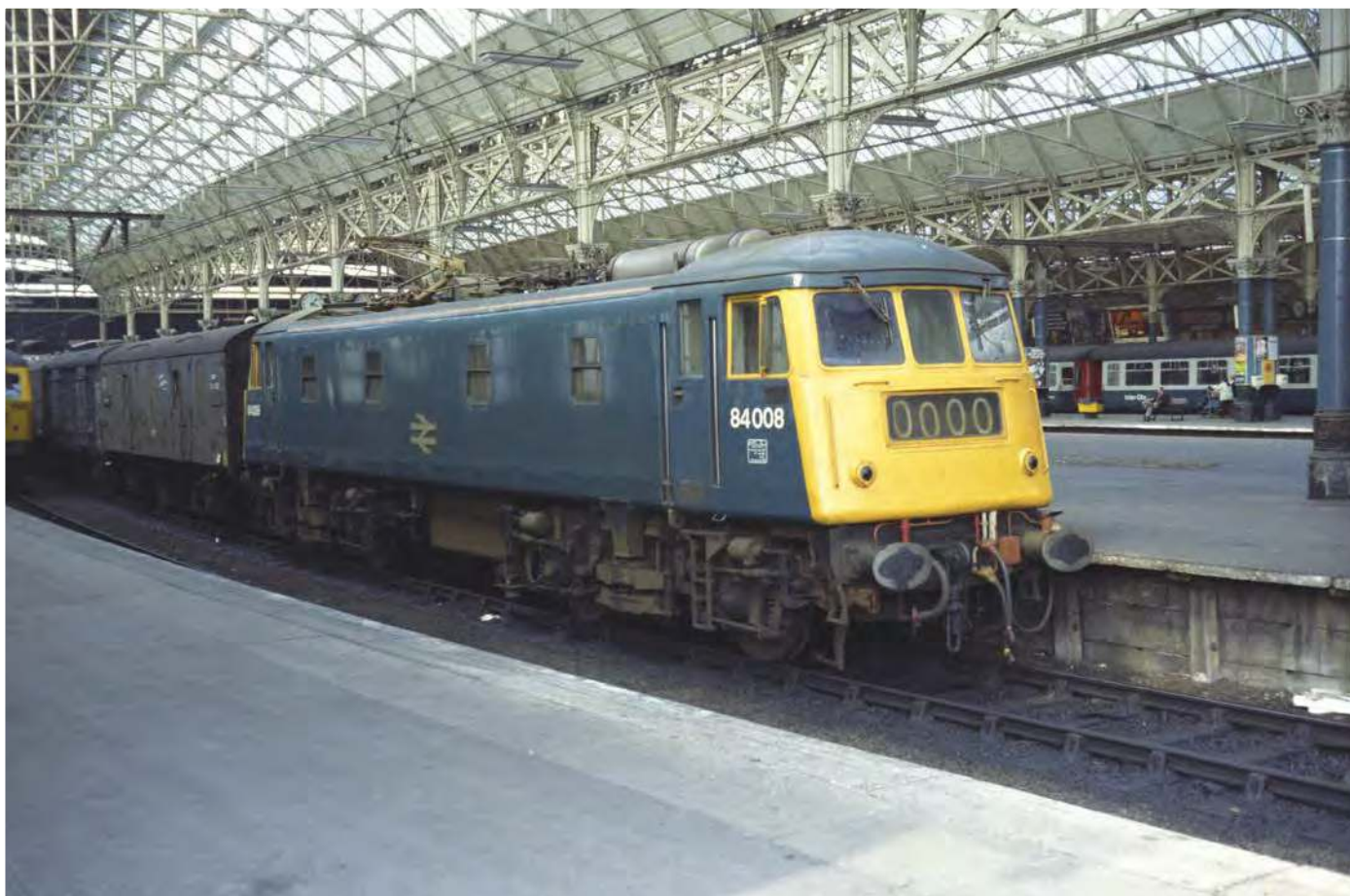
Mick had no driving experience of the Class 84s but recalls seeing one with its characteristic oval buffers. 84008 is seen at Manchester Piccadilly on a typical duty for this rather unreliable class, a parcels train. The date is 25th August 1979. RAY BRISCALL
