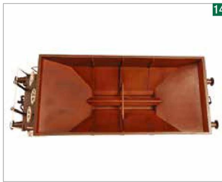
A look inside the wagon reveals rust speckles. Reduce the airbrush paint flow until it spits, rather than sprays, using a contrasting darker colour.
