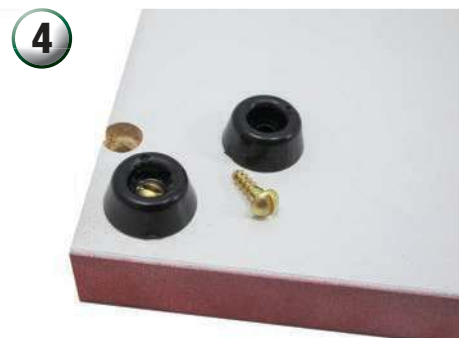
4 One thing that, in my opinion, is better under the board are the wires, so to allow a bit of space for them, I fit some rubber feet on to the bottom of the shelf.
