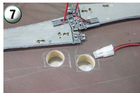
7 Point controls plug in under each motor and are supplied with plugs already fitted to the leads. This means a big hole is required under the board, so I use a 22mm wide spade part in a power drill. Overkill, a smaller hole would work, but this way I don't have to be as accurate with my positioning and the point will cover everything up.
