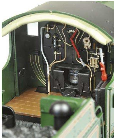
A very-neatly modelled cab interior. With the firebox door dropped down, an LED is visible which simulates a firebox glow. The rolled-up weather shield is a nice touch.
