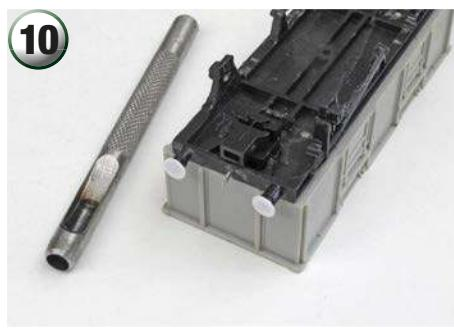
Fit larger buffer heads. Stamp these out from thin plastic card using a 5mm hollow punch. File the old buffer head flat first and then round the new buffer faces after fitting.
