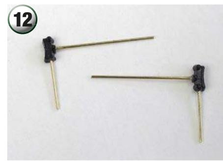
Cut the brake blocks out from the brake gear you previously removed. Drill two holes in each and glue in 0.45mm brass rod of lengths 20mm and 10mm as shown. Note that these fittings are handed – drill where the cuts were made.
