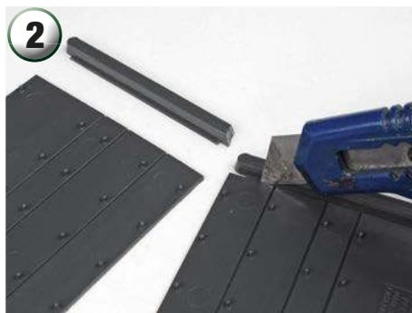
First remove the sprue from the end of each platform surface. Make several light passes with a knife and then bend to break along the score.
