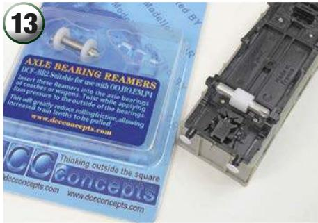
Fit the new wheels in place and check that they turn freely. If not, then adjust the fit using DCC Concepts' bearing reamers.
