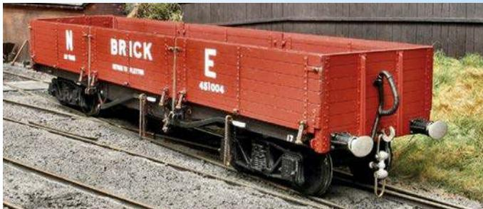
Built for the GNR in 1920 to carry products from the Peterborough-area brick makers, 25 of these fully-fitted wagons were built, with a further 25 by the LNER in 1930. They could transport 20,000 bricks, and being fitted allowed them to provide extra brake force on unfitted trains. Connoisseur Models' kit captures the essence of the prototype and contains a 22-page step-by-step booklet.
