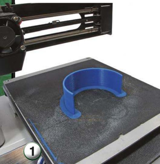
The curved parts are printed vertically, a clever move because it saves having to build a support structure inside. This is a separate file to the other parts, so you can print as many as you need.
