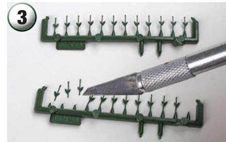
Line up the stalk sprues and then go down the length of each with a knife cutting out each stalk as you pass along. You will find it easier if you hold the top of each stalk down as you do so.
