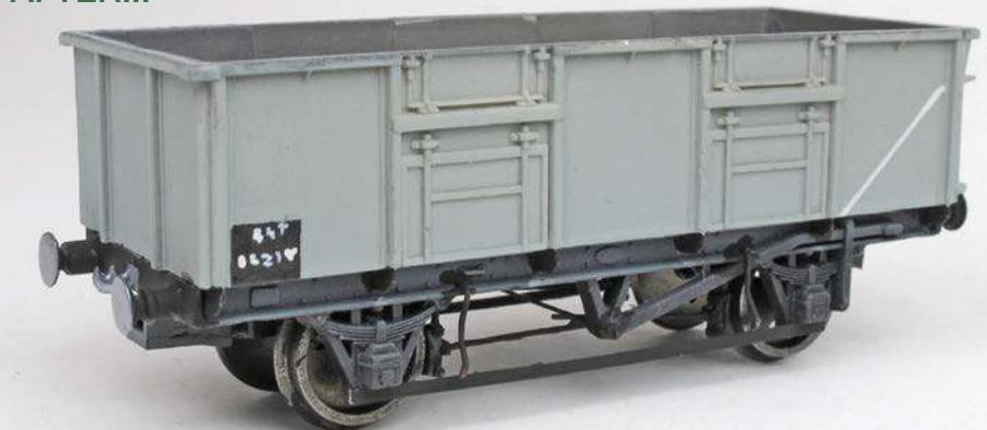
a model freight wagon from the 1970s-1980s to see if it could fit in with the high standards of modern model railway equipment. The item I have chosen is a Playcraft 24.5T mineral wagon, however, the techniques could be applied to much of the older stock that is freely available.
