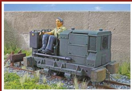
A smaller Ruston of 16hp. The prototype was supplied new to Woolwich with the nonstandard coupling gear. The model features an exhaust conditioner fitted to the rear of the locomotive. The wooden buffers on the model are made from a piece of pitch pine that was formerly part of an 1895-built 15in gauge Heywood coach that was replaced during its' restoration.
