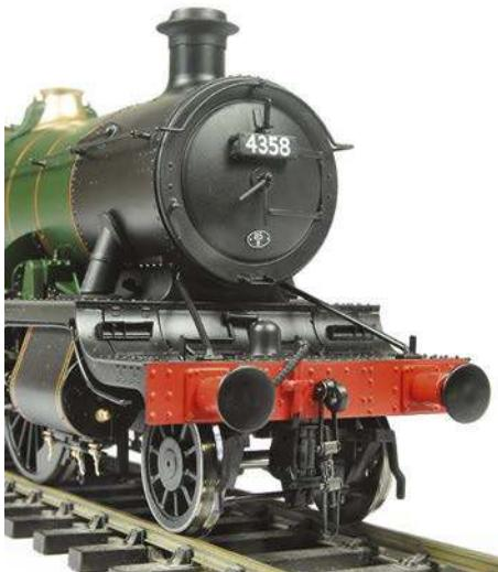
The front numberplate is attached in an entirely prototypical manner. A scale screw-link coupling is factory-fitted, and there's a nice rendition of the ATC shoe, along with its associated conduit along the offside valance.
