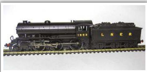
I've been RTR 'kit-bashing', so here are some photographs of a Bachmann 04, converted into a Q4 and a Bachmann K3 altered to a K5. The Q4 conversion took a lot of time. I shortened the running plate, made the firebox square with Plastikard, changed the dome for a
