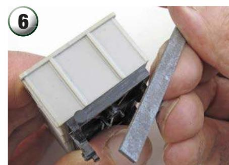
Many of my second-hand trucks have buffers missing. File the remnants of the old buffer away and then fit a new item using plastic rod or sprue left over from a kit.
