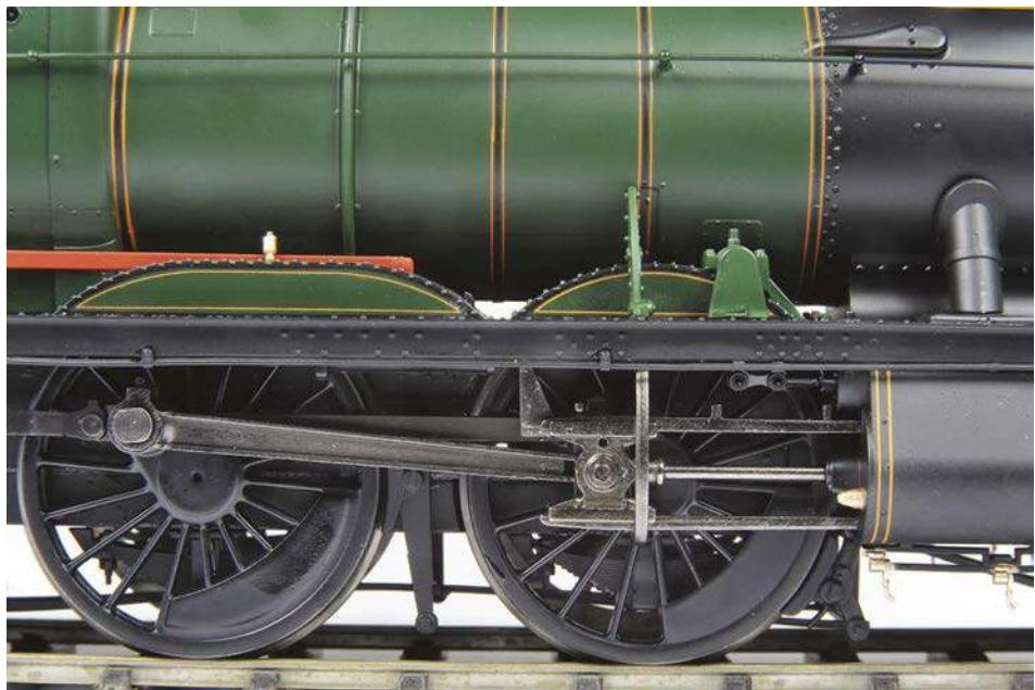
The 'drivers' are beautifully-modelled, and the motion is nicely-darkened. Note the extended centre splasher on this side (not on every locomotive) and the rare red reversing lever - a feature of Caerphilly Works, which Swindon eventually objected to.
