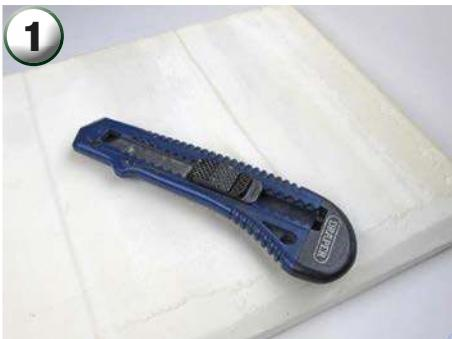
You can make the underlying support for the grass slope using any one of a variety of techniques. I used extruded foam as it is light and easy to form using a knife. It is also a lot less messy than expanded polystyrene.
