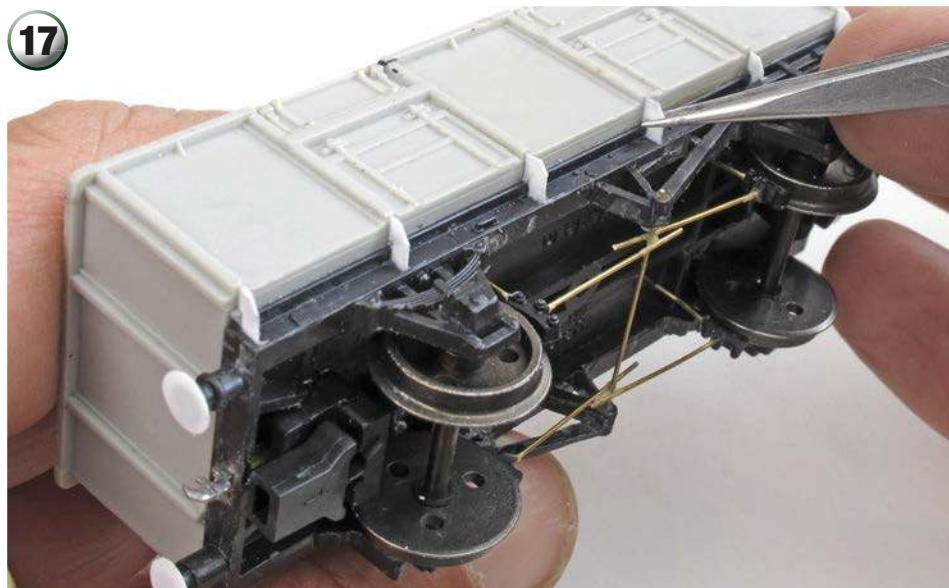
Using 0.25mm plastic card, make up 12 pieces to finish off the verticals on the bodysides. These need to be 2mm x 3.5mm in size. You need to cut off one corner and cut out a rectangle to account for the shape of the solebar. Fill in any small gaps with filler.
