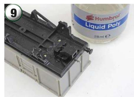
Glue NEM mounting blocks from Parkside Dundas in place using Liquid Poly. To get the spacing correct, fit the coupling pocket and ensure that it is level with the buffer beam.
