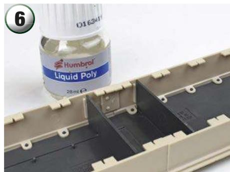
Join the platform pieces together using the tabs provided and glue with Liquid Poly cement.
