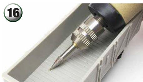
Use a rotary tool to clean up any brass rod protruding on the inside of the wagon.
