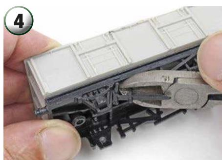
Remove all the brake gear except for the 'V' hangers and the brake levers using a pair of side cutters. File the remaining cut parts away smooth. Save the brake shoes as you'll be using them again.
