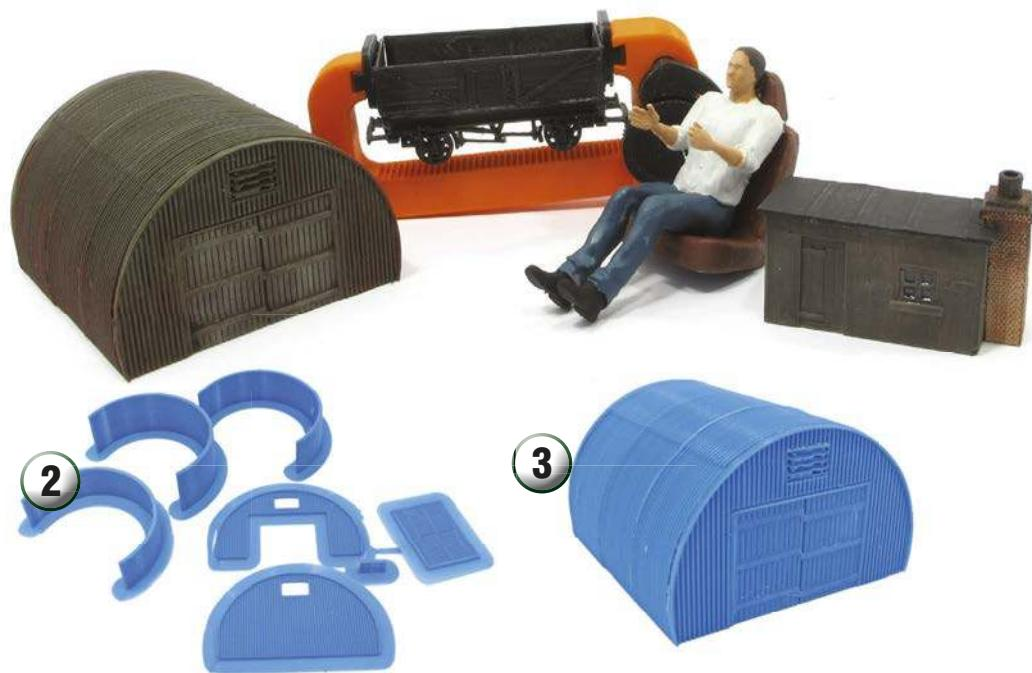
All parts are printed. They must be separated from the pad surrounds that help them stick to the printer bed. In most cases, these are pulled free, but some cleaning with a knife and abrasive stick finishes the job.
