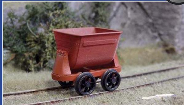
Based on information from a Robert Hudson catalogue from 1915, N Brass Locos has produced three narrow gauge 3D-printed wagon kits. Hudson's patented 'U'-shaped and 'V'-shaped double-sided tip trucks were more economical with space and were recommended for use in narrow tunnels where human or animal traction was used. N Brass Locos' version is based on the 10 cubic feet version. Kits include wheels, but no couplings.
