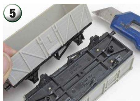
The brake levers are very thick so I decided to whittle them down using a knife. You may find it easier to remove them and fit a new piece of strip instead.
