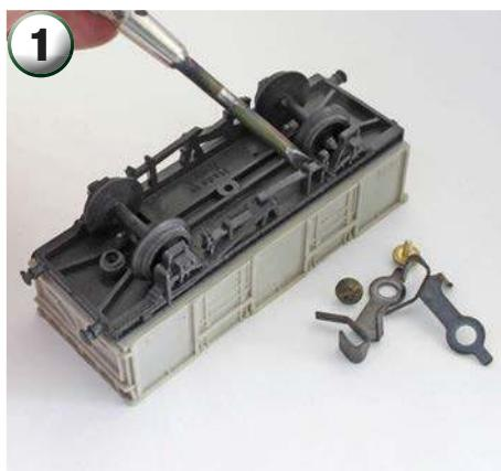
Second-hand items are often quite dirty. Lever out the wheels and undo the screws holding the couplings in place. Now gently wash the item in soapy water, brushing into all the corners, and allow to dry.
