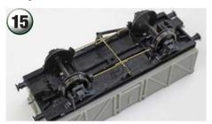
Glue the brake linkage in place on the floor and to the transverse member between the 'V' hangers. Note how one linkage goes under the transverse shaft and the other above. Ensure to leave enough clearance for the wheels to turn freely.
