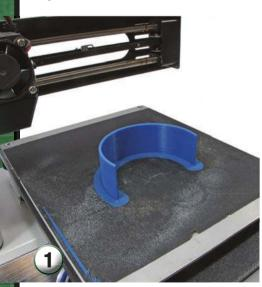
The curved parts are printed vertically, a clever move because it saves having to build a support structure inside. This is a separate file to the other parts, so you can print as many as you need.
