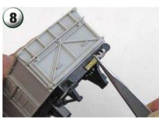
You will want to fit a coupling hook, no matter which coupling system you actually use to couple your trains. I made my own from scrap brass, but couplings are available from Slaters, Romford, 51L, Dart Castings, W&T and Alan Gibson.
