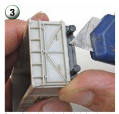
Remove flash and seam lines from the body and chassis using a knife and files.
