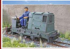
Ruston type 20DL. The prototype was supplied second hand to Woolwich Arsenal, and remained there long enough to be preserved. It is now 2ft gauge. Note the frame extensions fitted to Ruston Locomotives below 2ft gauge. This was to allow the drive chains to be on the outside of the wheels to clear the width of the gearbox, a feature perpetuated on the model.
