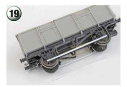
Using 0.25mm plastic card, cut out pieces 1mm x 52mm and glue below the axleboxes. You will have to file off a small amount of rivet detail to get a good surface for adhesion.
