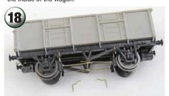
Using 0.45mm brass rod and pliers, bend up some door stops, one for each door, and fit in place with cyanoacrylate after drilling a suitable hole.
