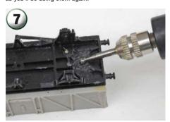
If you wish to fit new couplings then remove the old fittings using a rotary milling tool. Use a slow speed and work slowly to minimise production of toxic fumes. Work in a well ventilated area for this operation.
