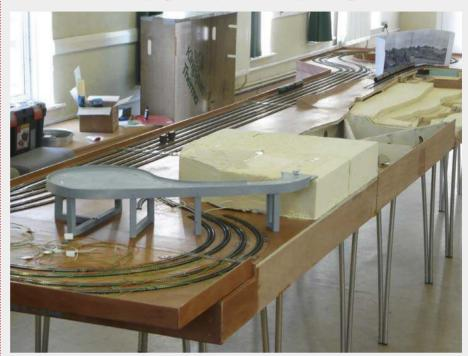
A photograph showing Wickwar in its early days. The beams and trackbed were made from 1cm 'Stryrofoam' as seen. Blocks of Styrofoam are in place as the basis of the scenery, yet to be carved to the correct contours. Some of the track and wiring is in place, and at the far end, the first black-andwhite trial of a backscene can be seen. Note the diagonal bracing
