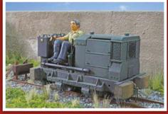
A smaller Ruston of 16hp. The prototype was supplied new to Woolwich with the nonstandard coupling gear. The model features an exhaust conditioner fitted to the rear of the locomotive. The wooden buffers on the model are made from a piece of pitch pine that was formerly part of an 1895-built 15in gauge Heywood coach that was replaced during its' restoration.
