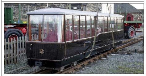
■ The Ravenglass & Eskdale Railway has taken delivery of the new observation carriage built for it by the Ffestiniog Railway at Boston Lodge Works. The carriage, built to a similar design to the FR's Pullman observation carriage launched in May 2018, is the first vehicle in a carriage replacement programme that the R&ER will be undertaking in conjunction with the FF&WHR.
