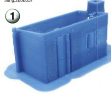
The hut is made from several different parts, each downloaded separately. I'm printing the main body, but for some reason, the roof won't print. You can see that there is quite a lot of support material in the door and window apertures. This is easily cut out with a sharp knife leaving accurate openings.
