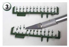
Line up the stalk sprues and then go down the length of each with a knife cutting out each stalk as you pass along. You will find it easier if you hold the top of each stalk down as you do so.
