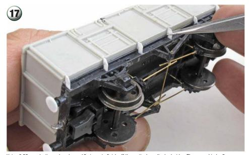
Using 0.25mm plastic card, make up 12 pieces to finish off the verticals on the bodysides. These need to be 2mm x 3.5mm in size. You need to cut off one corner and cut out a rectangle to account for the shape of the solebar. Fill in any small gaps with filler.
