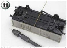
Drill 0.45mm holes in each 'V' hanger and thread through a piece of 0.45mm brass rod. Secure with cyanoacrylate.
