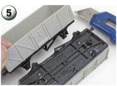
The brake levers are very thick so I decided to whittle them down using a knife. You may find it easier to remove them and fit a new piece of strip instead.
