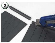
First remove the sprue from the end of each platform surface. Make several light passes with a knife and then bend to break along the score.
