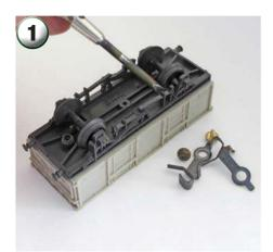
Second-hand items are often quite dirty. Lever out the wheels and undo the screws holding the couplings in place. Now gently wash the item in soapy water, brushing into all the corners, and allow to dry.
