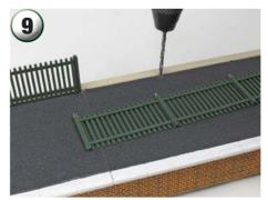
Drill holes for the station fence and glue in place using Poly Cement.
