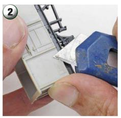
Remove the raised detail starting with a knife and then moving to a coarse file, then a fine file and finally fine grit paper.
