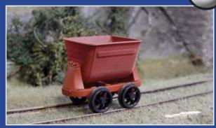
Based on information from a Robert Hudson catalogue from 1915, N Brass Locos has produced three narrow gauge 3D-printed wagon kits. Hudson's patented 'U'-shaped and 'V'-shaped double-sided tip trucks were more economical with space and were recommended for use in narrow tunnels where human or animal traction was used. N Brass Locos' version is based on the 10 cubic feet version. Kits include wheels, but no couplings.
