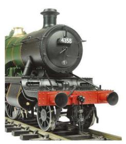
The front numberplate is attached in an entirely prototypical manner. A scale screw-link coupling is factory-fitted, and there's a nice rendition of the ATC shoe, along with its associated conduit along the offside
