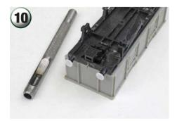
Fit larger buffer heads. Stamp these out from thin plastic card using a 5mm hollow punch. File the old buffer head flat first and then round the new buffer faces after fitting.
