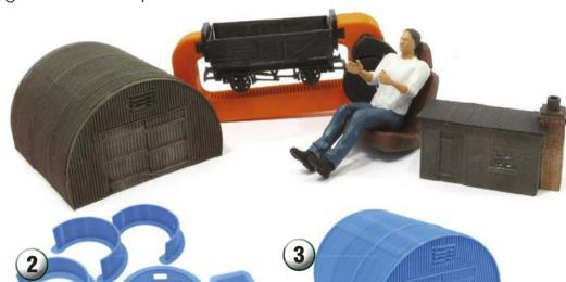
All parts are printed. They must be separated from the pad surrounds that help them stick to the printer bed. In most cases, these are pulled free, but some cleaning with a knife and abrasive stick finishes the job.
