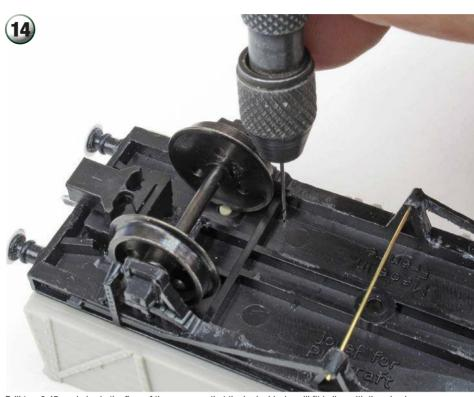
Drill two 0.45mm holes in the floor of the wagon so that the brake blocks will fit in line with the wheels.
