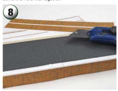
Add the self-adhesive facing to the platform sides. Stagger the pieces so that the platform join is less obvious. You can use stone or brick-embossed plastic card for the facing if you want a better finish.
