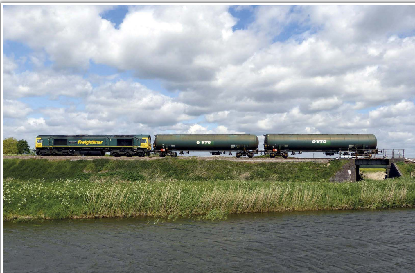
The earliest months of the fuel workings to Ipswich employed the VTG/Greenbrier design of modern TEA bogie tankers. Most commonly associated with lengthy block trains, two of the ex-Freightliner batch look bizarre behind 66592 Johnson Stevens Agencies on May 12, 2015, as the 6E50 Ipswich-Lindsey passes Turves, between March and Peterborough. ADRIAN TIBBLE
