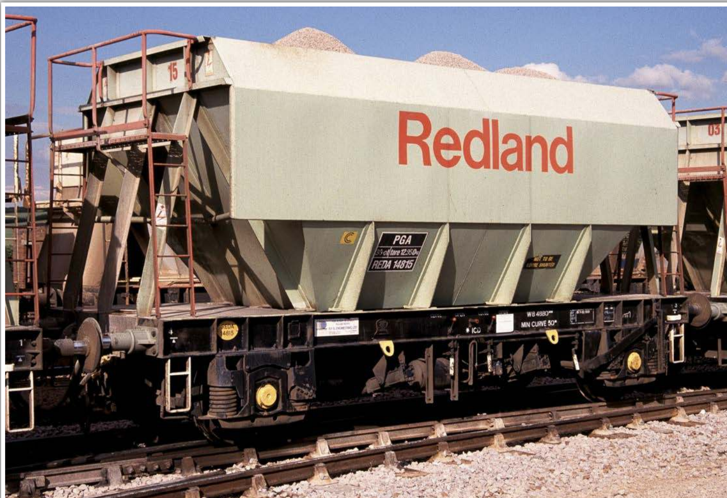
One of the Standard Wagon built PGAs, No. REDA 14815, is pictured at Mountsorrel in August 1997. A feature of the Redland PGAs was the stencilling of the last two digits of their number high up on the end for the benefit of the operatives situated in the above-rail loading cabin at Mountsorrel. Also of note is the incorrect wheelbase lettering on the solebar. DAVID RATCLIFFE
