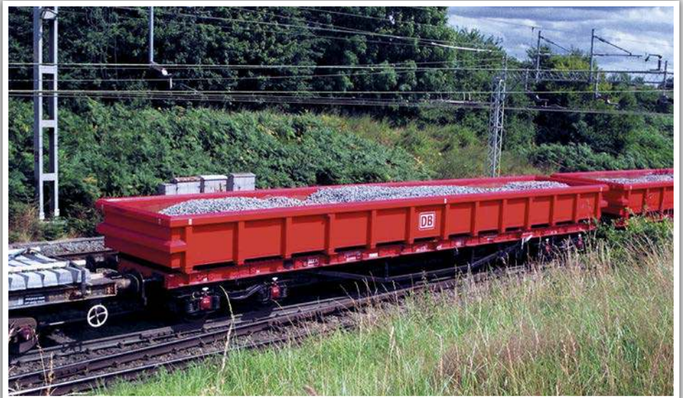
BELOW: MVA No. 910164, a 'Lobster' converted from a BBA, is pictured at Peak Forest on May 24, 2016. By this date it was in revenue traffic on behalf of Cemex working between Doveholes Quarry and the stone terminal at Ripple Lane. DAVID RATCLIFFE
