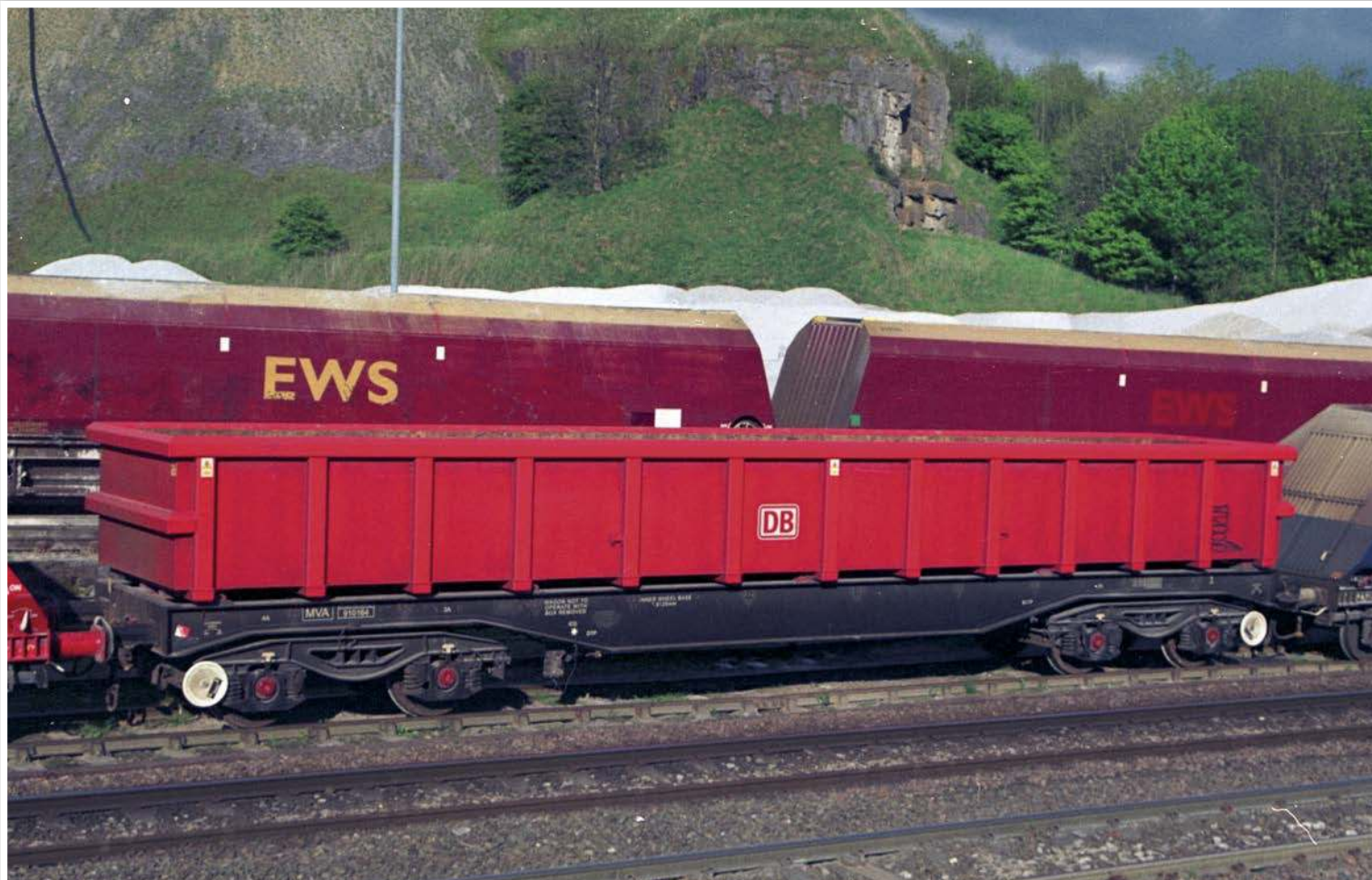
BELOW: MVA No. 910164, a 'Lobster' converted from a BBA, is pictured at Peak Forest on May 24, 2016. By this date it was in revenue traffic on behalf of Cemex working between Doveholes Quarry and the stone terminal at Ripple Lane. DAVID RATCLIFFE
