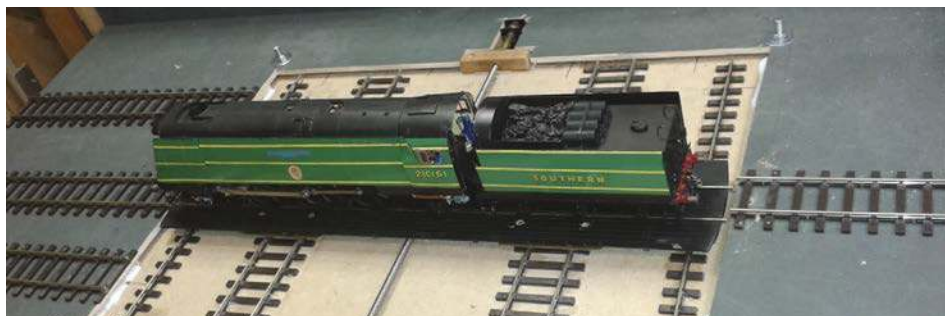
A bird's eye view of the traverser's basic structure, which shows the universal drive screw powered by a Portascap motor via a flexible connector. Four bolts were used to locate and support the traverser base while being worked or having to be removed for any reason. Once completed, bolts were removed for a permanent under-board support.
