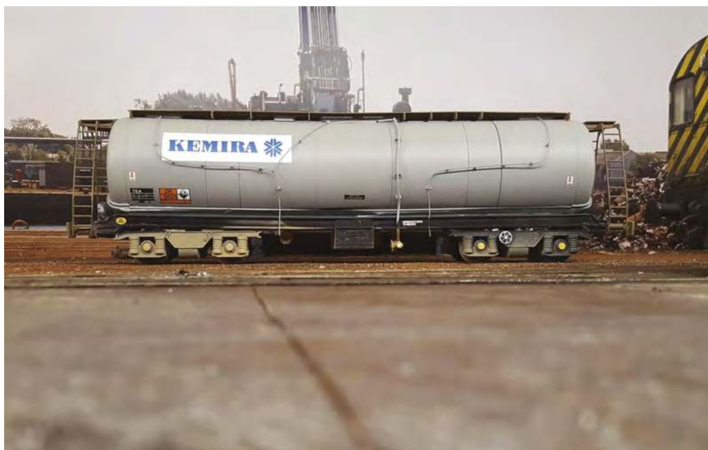
Paul Rolley's TEA nitric acid tank wagon, as used on runs to Sellafield for dissolving the metal around nuclear fuels before reprocessing. This model is to be made available shortly as a kit.
