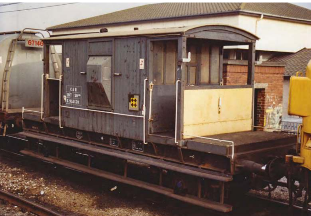
Taken on November 27, 1991, LNER 20T brake van B955139 was being used by Trainload Coal sector as a barrier vehicle and coded CAR. Note the vinyl sticker, plated metal ends and accumulation of dirt on the windows. TREVOR SMITH
