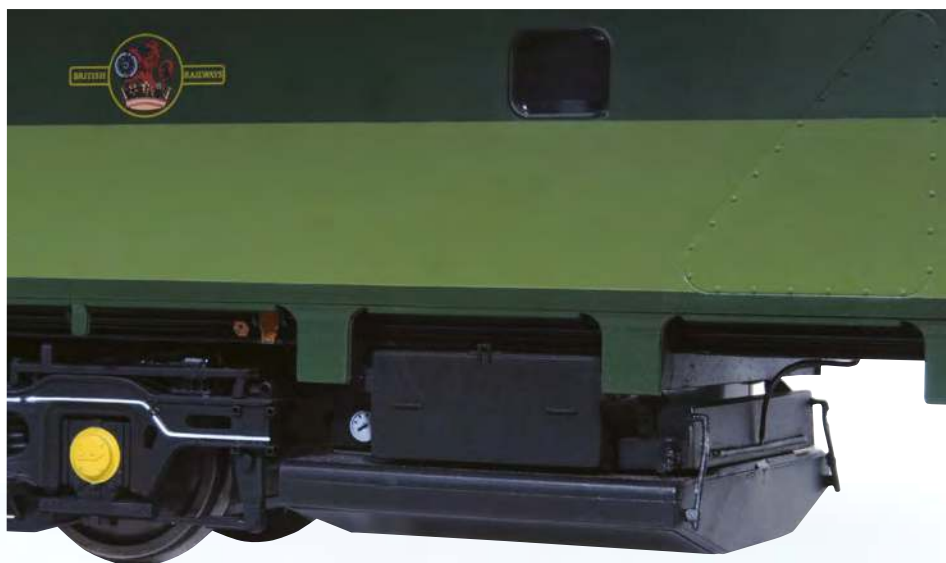
A largely sparse underframe area devoid of water tanks is to be found on the Class 25/3s, though its fuel tank is well observed with gauge and pipework.
