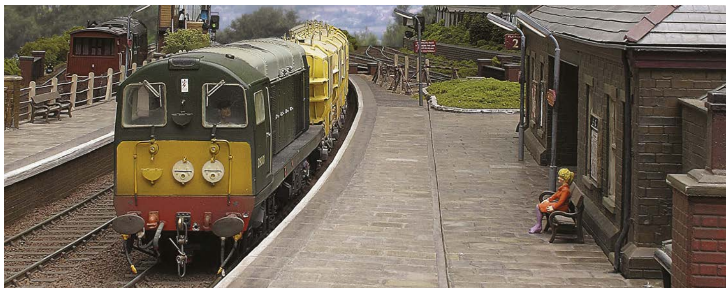
Keith Harrison and David Hampson's 'Apethorne Junction' owes its smooth operation largely to a large return loop at one end of the layout. The line in this shot runs behind the camera in a loop, returning to the right, behind the Class 20 with its rake of cement hoppers. See the trackplan of this layout on page 92.
