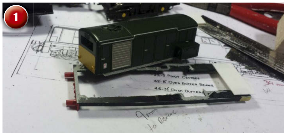
Firstly, the Class 17 body and chassis were stripped to their component parts and work started on removing the bonnet sections from the running plate, making sure to preserve as much of the details of the bonnet side doors as possible.
