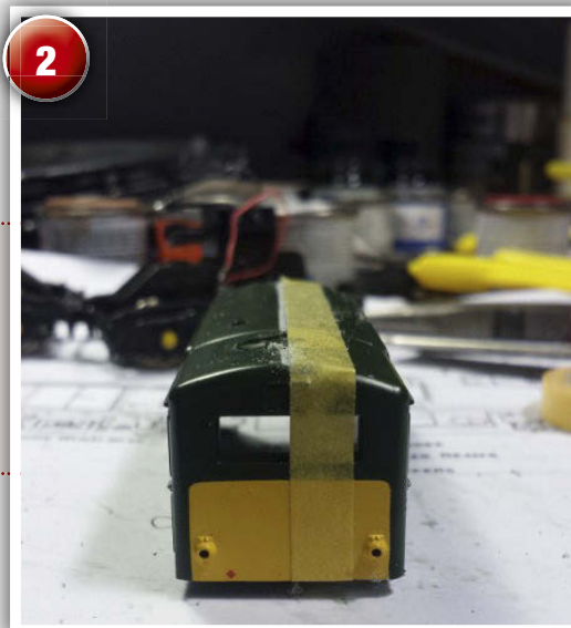
Firstly, the Class 17 body and chassis were stripped to their component parts and work started on removing the bonnet sections from the running plate, making sure to preserve as much of the details of the bonnet side doors as possible.
