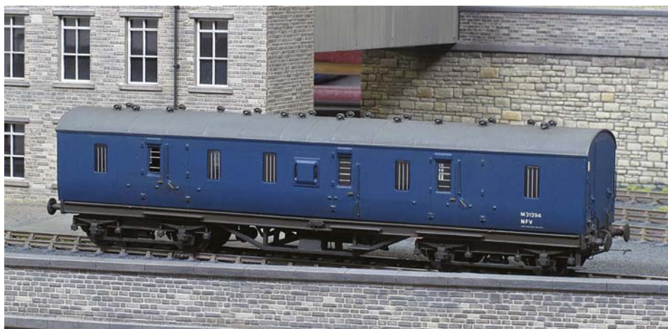
Ex-LMS/Stanier 50' full brake. This uses an old Mainline model as the basis. The bogies have been replaced with Comet, while a certain amount of extra detail has been added to the underframe (including new buffers – also from Comet, plus scratchbuilt footsteps). On the body, the end corridor connections have been removed (as was done on some vehicles at this period), with new end framing and other detail being fabricated. New, separate wire handrails were fitted, along with door handles, while the windows have been flush-glazed with individually cut pieces of clear acrylic, with the glazing bars represented by pieces of pre-painted 0.3mm nickel-silver wire.
