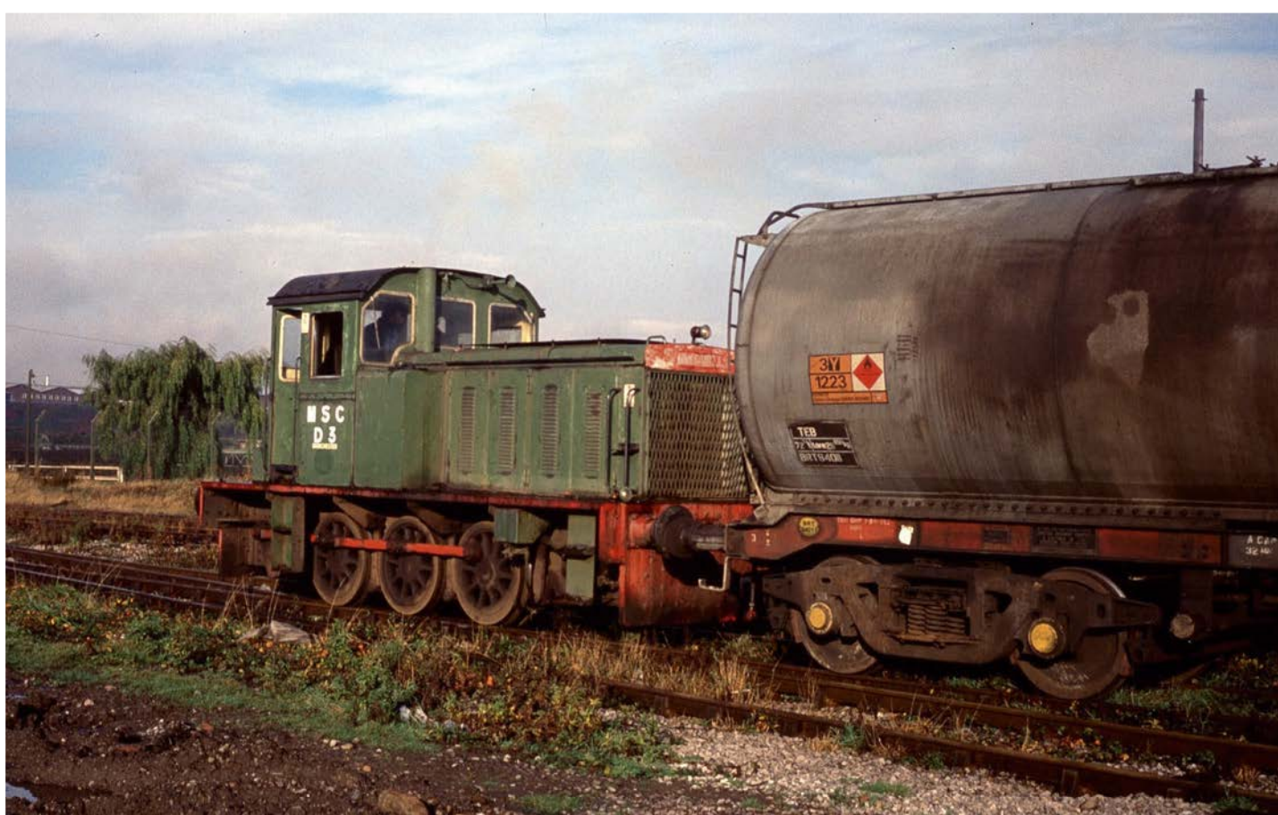
Opened in 1965, Weaste oil depot was situated next to the Manchester Ship Canal and, to access the unloading sidings trains, had to traverse a short section of the privately owned Manchester Ship Canal Railway. Consequently the BR locomotive would leave its train at Weaste Junction with all shunting into and out of the oil depot being performed by one of the Ship Canal's own locomotives. MSC No. D3, a Hudswell Clarke 204 bhp 0-6-0DM (works No. HC D1188/built 1960) shunts loaded tanks of kerosene at Weaste on 8th December 1989.
