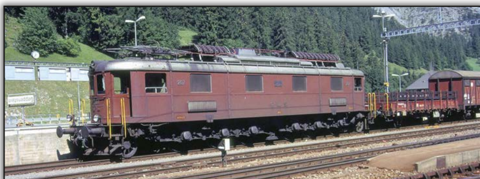
Ae 6/8 No. 207 is at Kandersteg on the BLS Spiez to Brig line on the 14th August 1991. The regenerative braking racks can be seen on the roof. DAVID FORD
