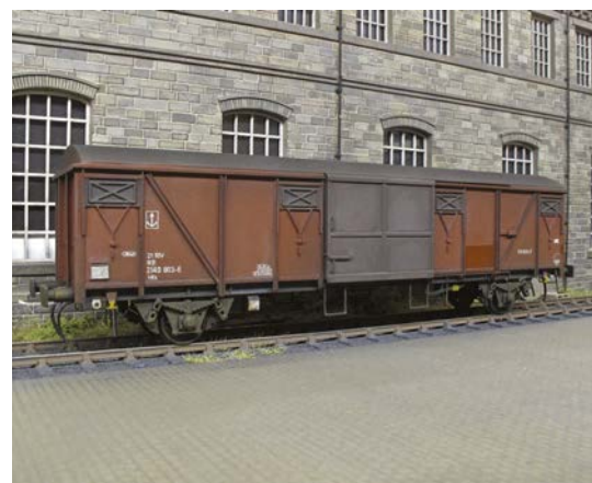
The completed Belgian Ferry Van. Painting was by hand using Humbrol enamels. A coat of Johnson's Klear was applied to areas where the transfers were to go, with a further coat to seal them in after allowing to dry thoroughly. A couple of coats of Testors Dullcote spray varnish were then applied, after which final weathering could take place.
