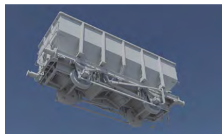
CAD images of the models have been released showing a wealth of chassis detail, instanter couplings, spring and hanger detail.
