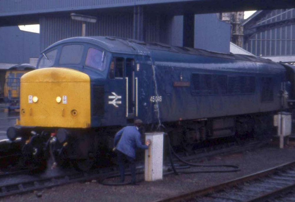
On 10th May 1979 Saltley secondman Mike McClelland gets wet as the boiler water tank overflows on platform 5 at Bristol Temple Meads while his driver Charlie Fletcher finds it rather amusing. Mike is closing the main valve and will close the bottom valve on the loco before removing the pipe. This was an important fact I forgot to my cost on one occasion at Bristol. NEVILLE SLOPER
