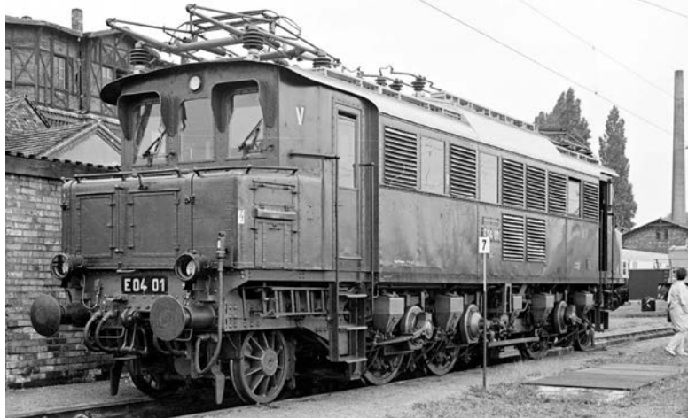
A development of Class E17, but for lighter express passenger services, was the Class E04 1-Co-1, the prototype of which, DR No. E04 01 (numbered at the other end 204 001) was exhibited at Halle in May 1995. Note the apparently 'missing' third driving axle. As the class was intended for lighter duties one driven wheelset was simply omitted without altering the positions of the remaining three driving axles!
