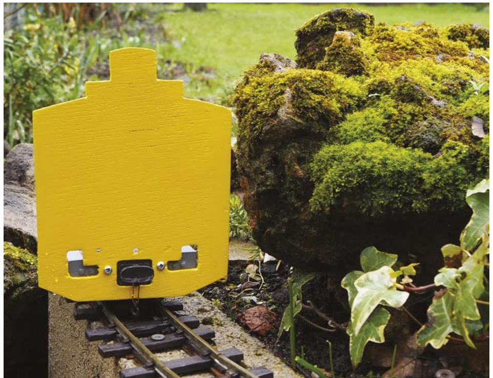
Above: My home-made loading gauge which is fitted to the track measuring wagon seems to be invaluable for rail setting on the rock embankments below Mt Bludfreezin.
