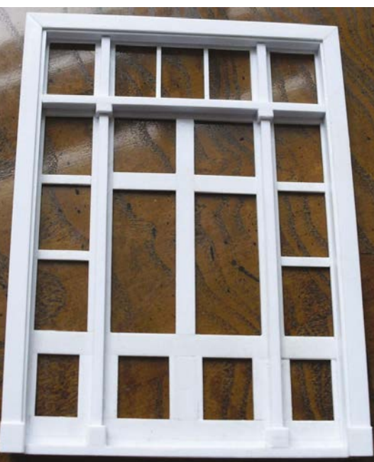
Window and door master made of 'Evergreen' styrene strips used to make a mould for producing resin castings.
