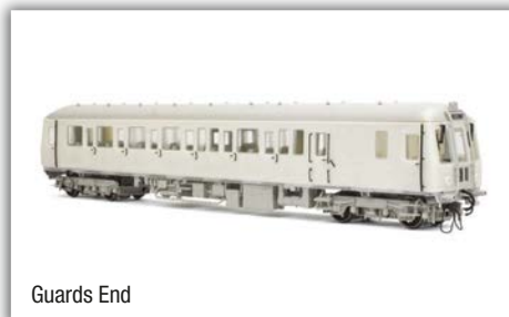
Model: O Gauge Class 122 DMU Expected: Q4 2018 Features: Three different buffer, exhaust and chassis types, interior detailing and DCC sound option
