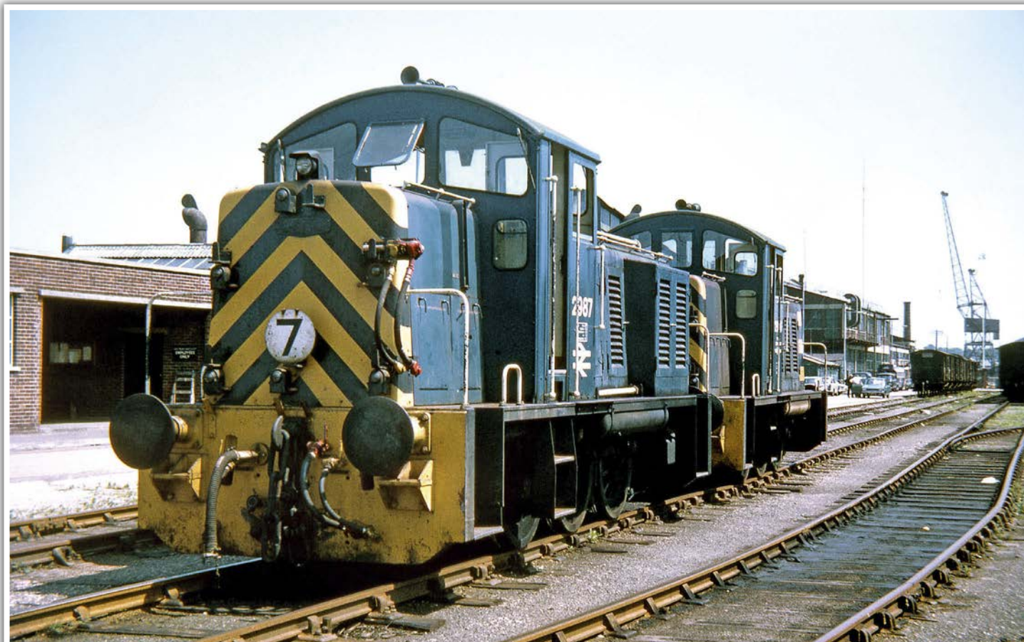
Southampton Western Docks on July 12, 1970. The additional cabinet added to the solebar to house the exhausters for the air brakes as seen on 2987. Behind is classmate D2996. These locomotives became 07003 and 07012 respectively. RAIL PHOTOPRINTS
