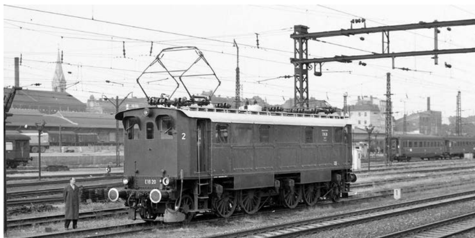
An early Bavarian express passenger electric 1Bo-Bo1 was Class E16, epitomised by No. E16 20 that was photographed outside München Hauptbahnhof on 7th September 1958. This side showed no sign of the Büchli drives from the motors to the wheelsets; these were prominent on the other side of the locomotive. All of these older passenger electric locomotives were painted green with black running gear. (Ed. Regular readers will be familiar with the appearance of the Büchli drives from the recent articles about Swiss locomotives in TRACTION).
