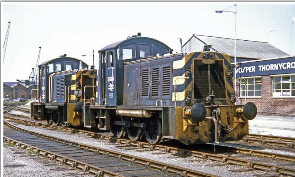
Viewed from the other end are the same two locomotives. Nearest, 2996, has a shunter's pole across the top of its bufferbeam, which is a much simpler layout because it is vacuum-braked only. The additional white waist-level pipes on 2987 can be seen. RAIL PHOTOPRINTS
