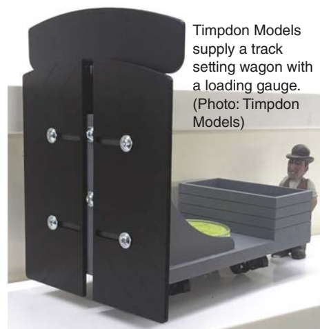
Track setting and ballasting is a key issue. My track setting and ballasting wagon has a calibrated rail to ensure accuracy of the two spirit levels.
