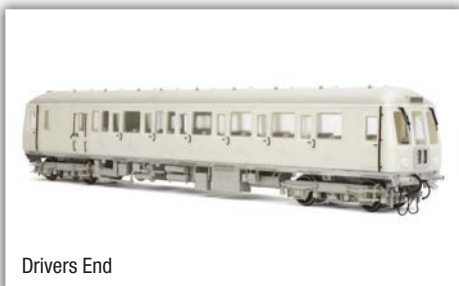
Model: O Gauge Class 122 DMU Expected: Q4 2018 Features: Three different buffer, exhaust and chassis types, interior detailing and DCC sound option
