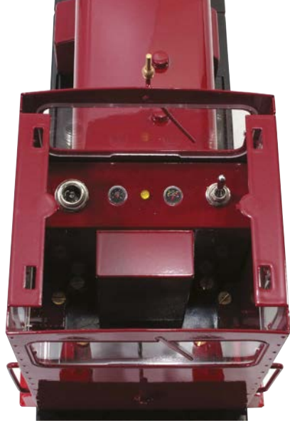
Removing the roof gives access to the on/off switch and charging socket.
