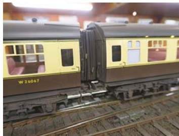
Magnetic coupling corridor connections
