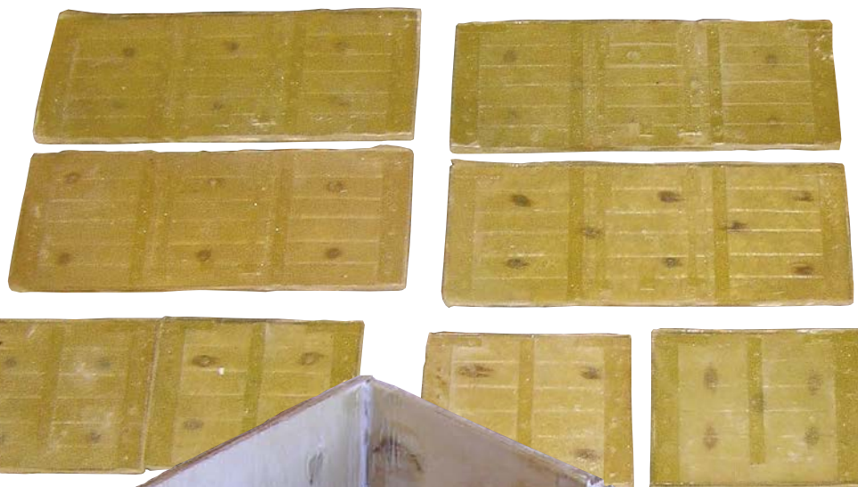
Parts for two trucks out of the mould and de-flashed.
