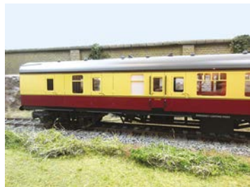
Brass sides with die-cast chassis
