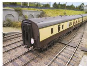
Working brake light on brake ends
