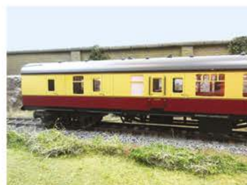
Brass sides with die-cast chassis
