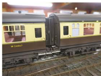
Magnetic coupling corridor connections
