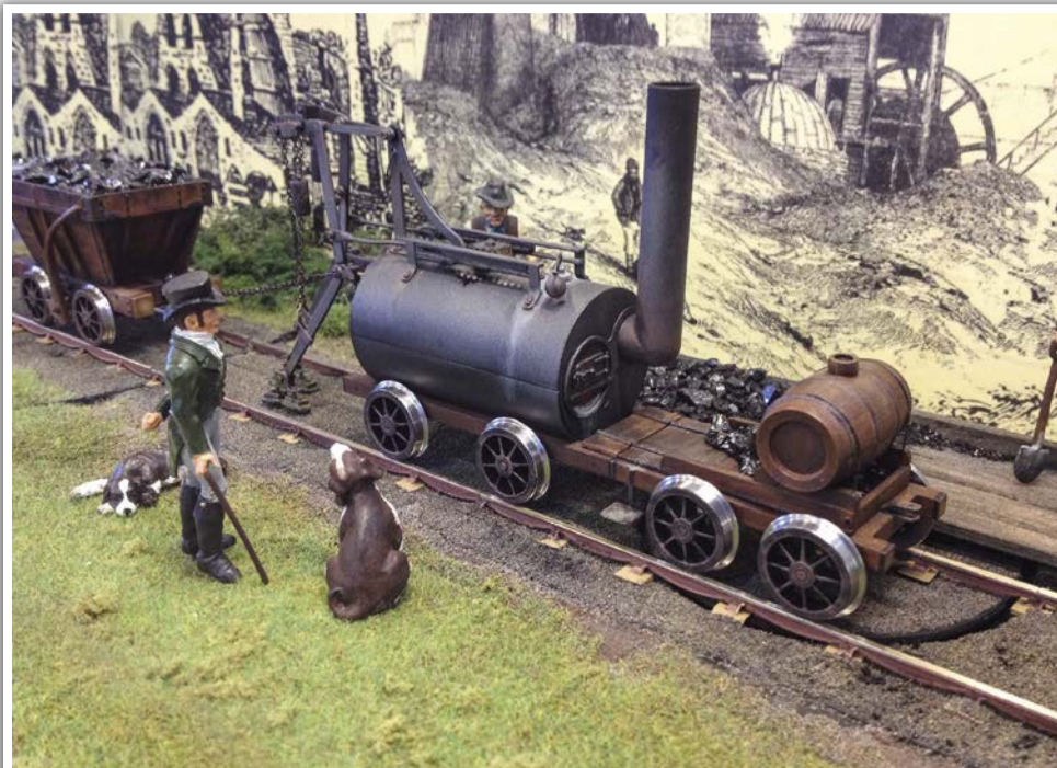
Hauling its loaded coal wagon via a chain, Brunton's 'horse to go by steam' is almost other worldly.
