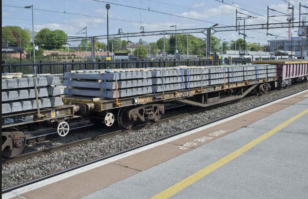
DB Schenker YWA 'Salmon' bogie sleeper carrying wagon 996485 is caught at Northampton, in the consist of 6A11 - Bescot Up Engineers Sidings to Bourne End Junction engineers' on May 3, 2014. DAN ADKINS
