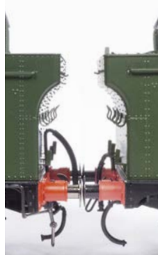
Back to back, the 64XX left, 57XX right. A nice array of bunker rivet detail and lamp brackets. Note how buffers and bunkers align perfectly between the two.
