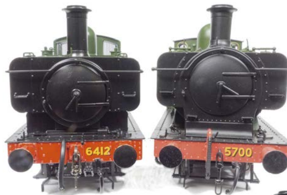
The sister act - left the 64XX, right, the 57XX. Note the difference in boiler position and water tank heights through evolution on a design which stood the test of time for many years.
