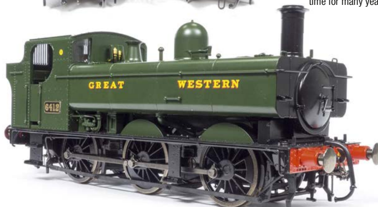
Dapol's 64XX - a fine model indeed. The GWR introduced the non-auto fitted 74XX class in 1936. Its higher 180psi boiler pressure and right-angled join between cab sheet and bunker top edge distinguished it from the 64XX with its radius profile in this area.
