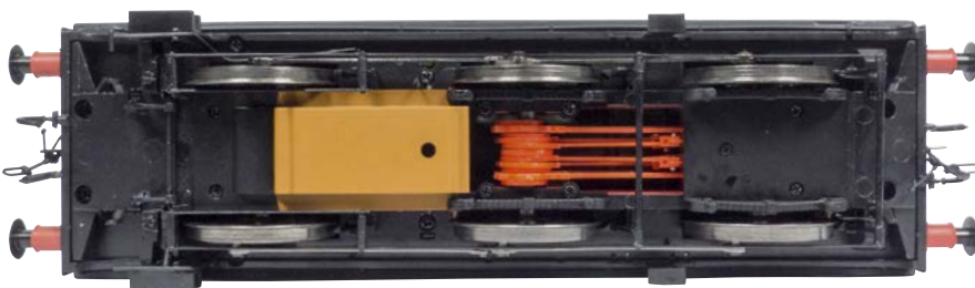
The flip side - the 64XX above and 57XX below. Both are driven via the rear axle, but the new 57XX offers a more realistic view between the frames. Note the different methods of compensation.
