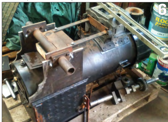
PHOTO 6: Beginning to take shape as the hornplates are offered up.
