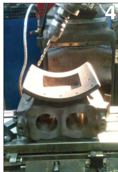
PHOTO 4: More careful measuring as the cylinder saddle is drilled.
