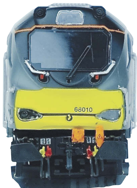
Left: The distinctive 'Stormtrooper' face is captured perfectly. Commendably, the Chiltern Railways locomotives have the extra AAR multiple working/push-pull control socket mounted to the left of the electric train supply jumper cable. Bufferbeam hoses and cables are factory-fitted at one end.
