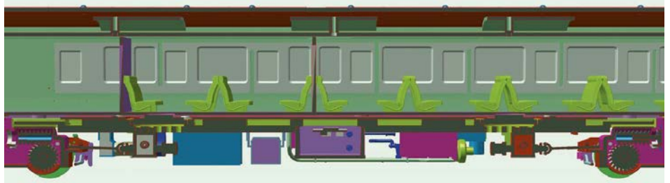
CAD artwork has been developed for Dapol's Class 121 and 122 project, allowing 3D test prints to be displayed at the show. Note the location of the bogie-mounted motors in the cutaway below.
