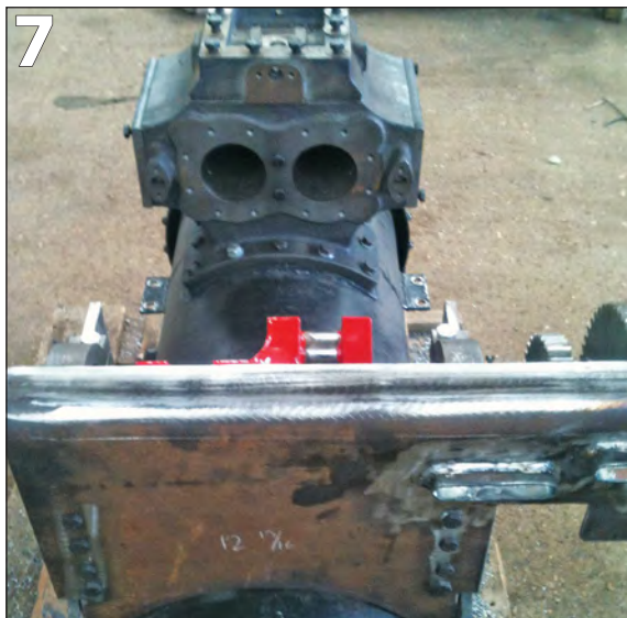
PHOTO 7: Setting the motion bracket.
