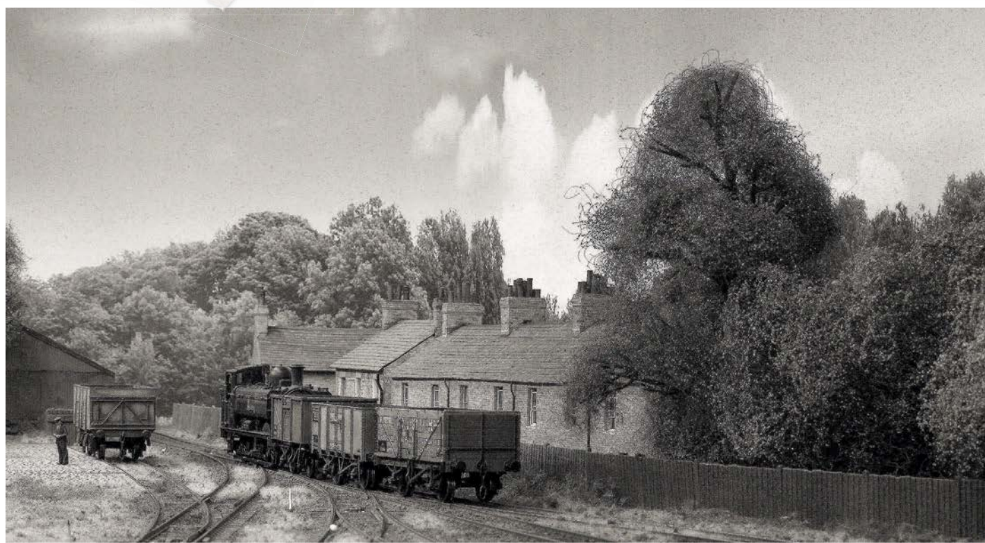
The Goods office manager checks his timings as Pannier 7781 pauses during shunting the yard. The locomotive origins are a Bachmann DC 57xx pannier. To capture the everyday look, the fire iron hooks are populated with a set of etched fire irons, the rear cab shutter has been opened, the lamp brackets replaced and three link couplings fitted. Note the Fireman's shovel wedged in the handrail, ready to move coal in the bunker. Small details such as these add to a locomotive's personality.
