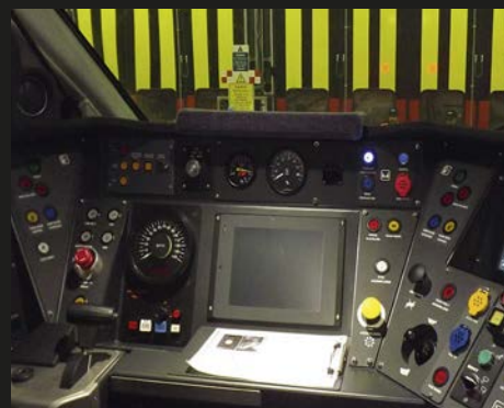
The Cab of a GWR Class 800 showing the ATP Speedometer (left), the ETCS Driver Machine Interface (centre) and Train Management / GSM-R Systems (right) SIMON PALEY. Taken with kind permission of Hitachi Rail Europe.
