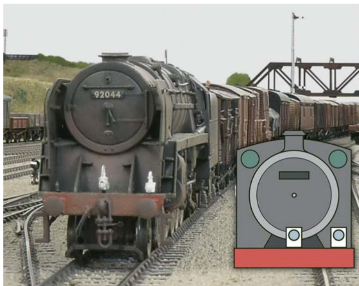
Class E. Express freight, livestock, perishable or ballast train with not less than one third of the vehicles vacuum braked and piped to the engine.
