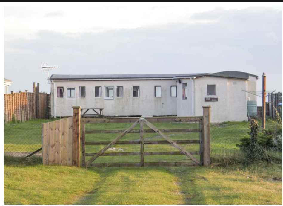
Pagham Beach in West Sussex has a number of railway cottages, but it's easier to identify them from the rear. This Victorian carriage grounded in the 1920s is protected by the almost obligatory pebble dashed finish for weather protection and isn't completely disguised by later additions. CLIVE BARKER
