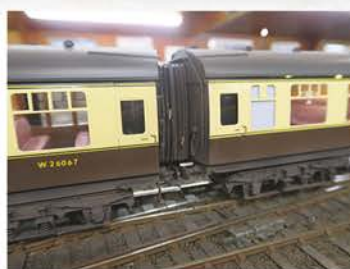
Magnetic coupling corridor connections
