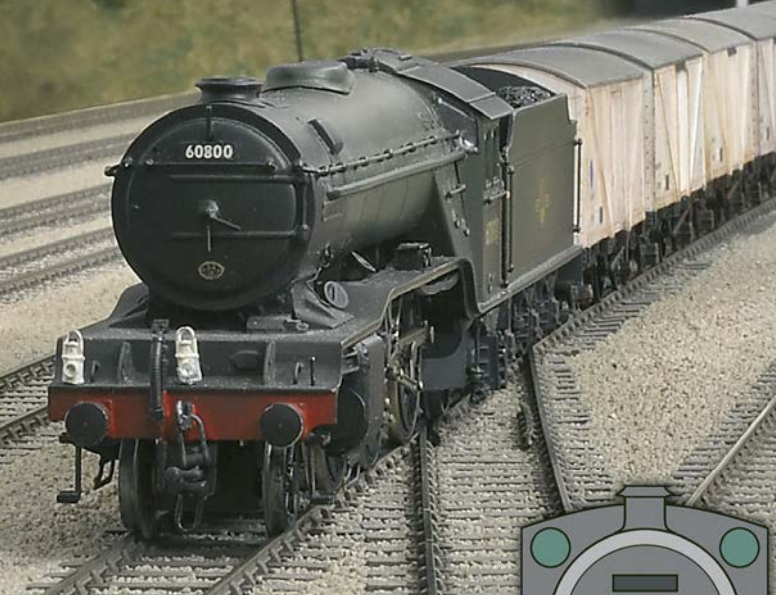
Class C. Parcels, fish, fruit, livestock, milk or other perishable train composed entirely of vehicles conforming to coaching stock requirements; express freight, livestock, perishable or ballast train pipe-fitted throughout and with automatic vacuum brake operative on not less than half of the vehicles; empty coaching stock (not specially authorised to carry class 'A' headcode).
